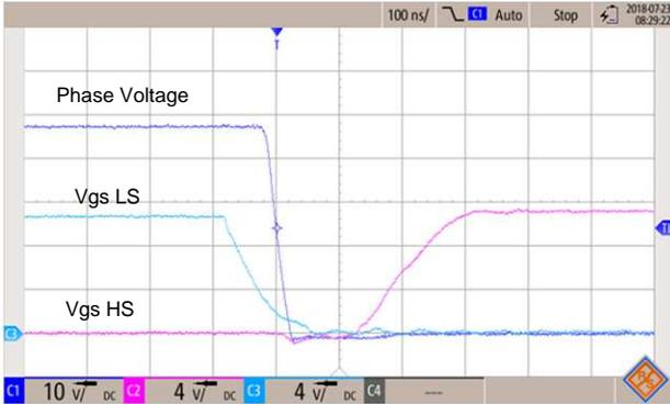
**Figure 9. Hard Switching Phase A Voltage Rising Edge, Phase Current at 48 V, -10 A**
