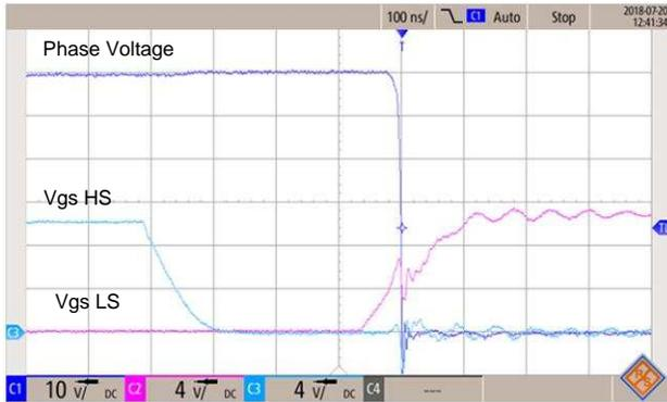
Figure 15. Soft Switching Phase A Voltage Rising Edge, Phase Current at 60 V, 10 A
