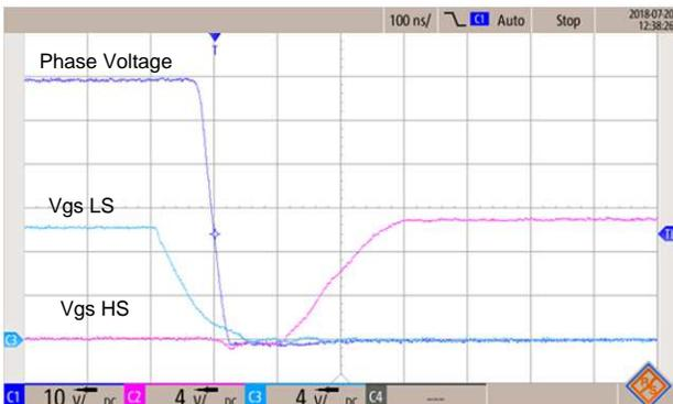
**Figure 13. Hard Switching Phase A Voltage Rising Edge, Phase Current at 60 V, -10 A**
