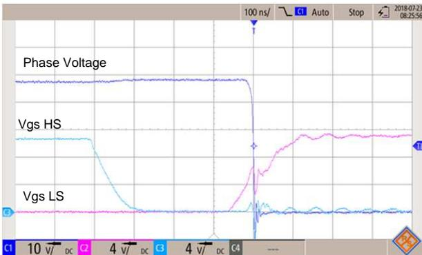
**Figure 11. Soft Switching Phase A Voltage Rising Edge, Phase Current at 48 V, 10 A**
