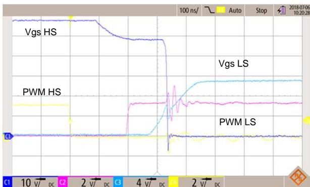
**Figure 22. Independent Mode PWM vs  $V_{GS}$  LS and HS, Phase A Current at 48 V, 5 A Soft Switching**
