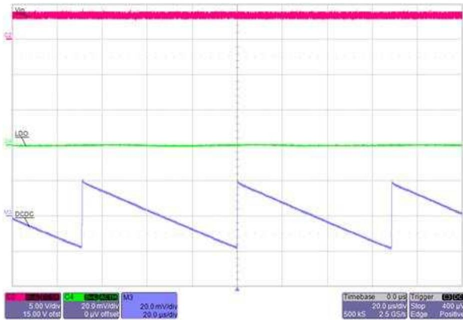
Figure 7. TIDA-01566 Output Ripple ( $V_{in} = 3.6\text{ V}$ , Load = 1 mA)
