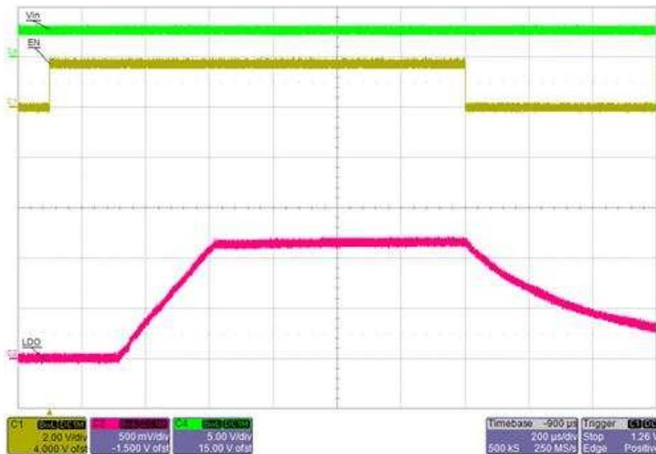
Figure 35. TPS7A10 Start-Up and Shutdown ( $V_{IN} = 3\text{ V}$ , Load = 0 A)
