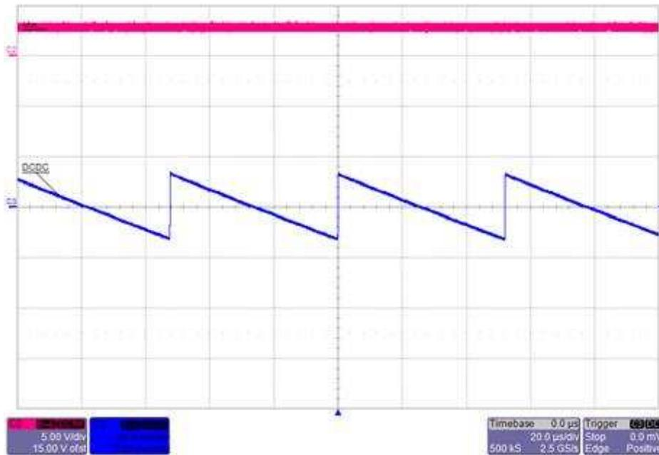
Figure 16. TPS62801 Output Ripple ( $V_{IN} = 3\text{ V}$ , Load = 1 mA)
