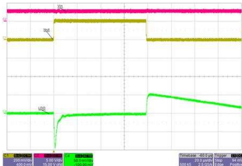
Figure 33. TPS7A10 Load Transient Response ( $V_{IN} = 3$  V, 1-mA to 200-mA Load Step)
