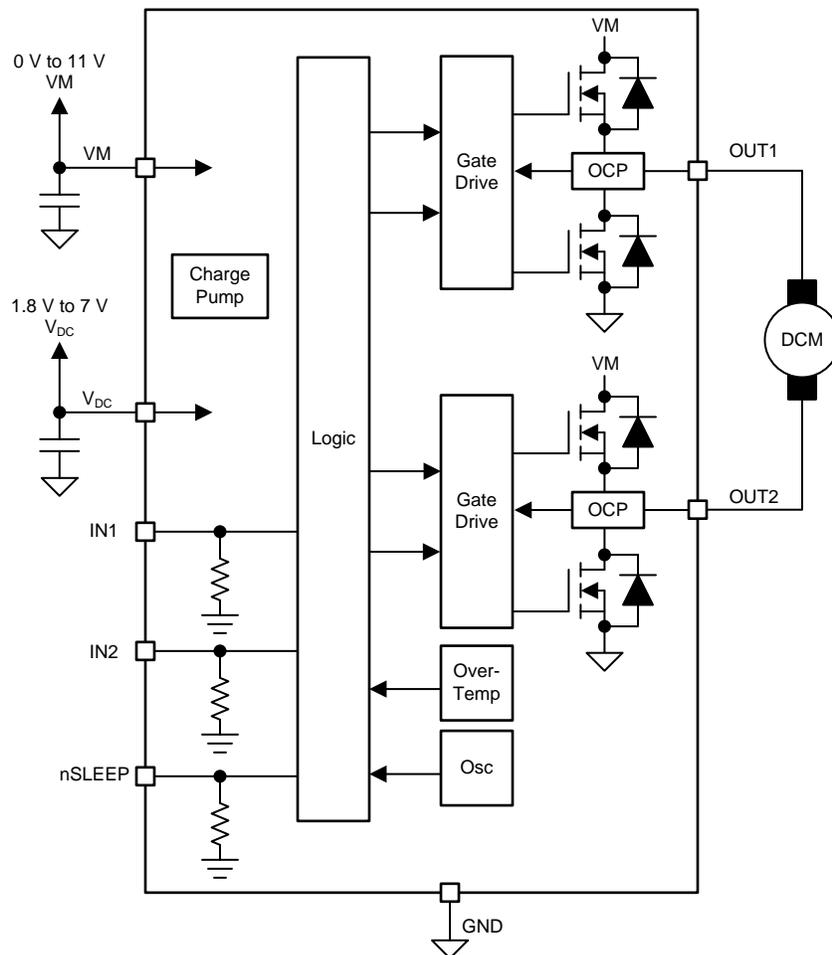
Figure 5. DRV8837C Functional Block Diagram
