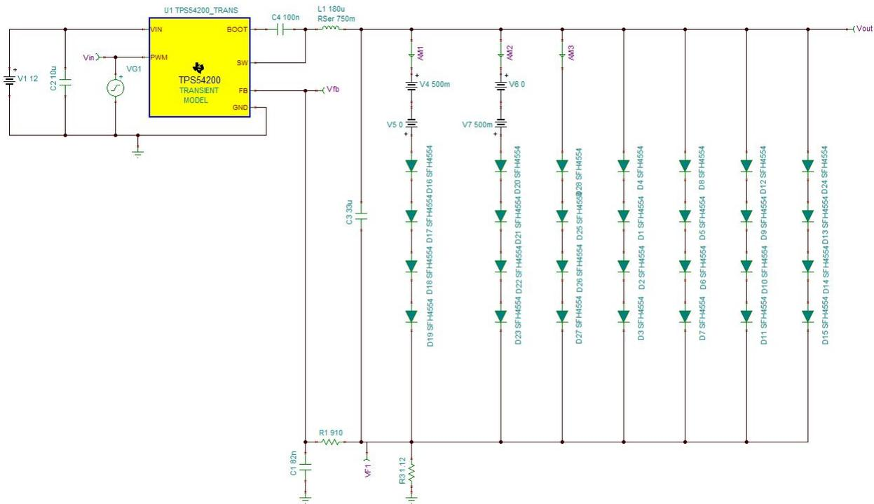
Figure 9. Simulation Circuit Without Channel Ballasting
