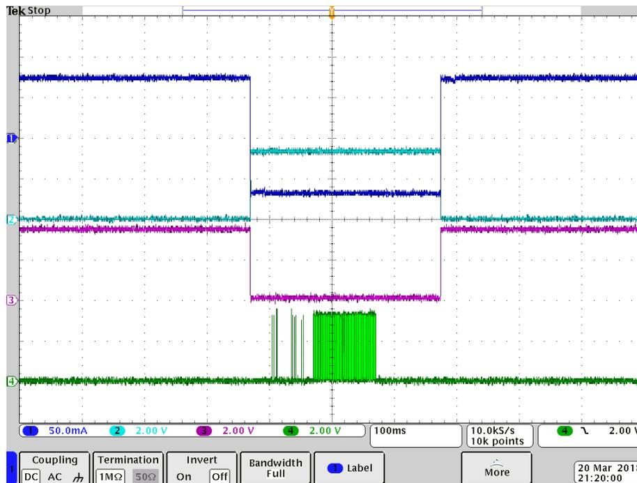
**Figure 43. Bidirectional Current Control Using the DRV8837C**
