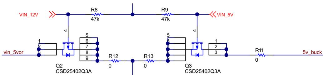
Figure 7. ORing Circuit for 12-V and 5-V Input
