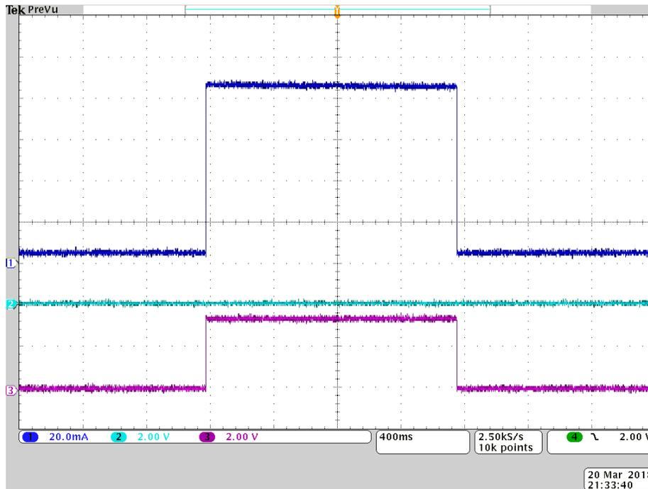
**Figure 44. Current Consumption Difference in Sleep Current and Coil Current**
