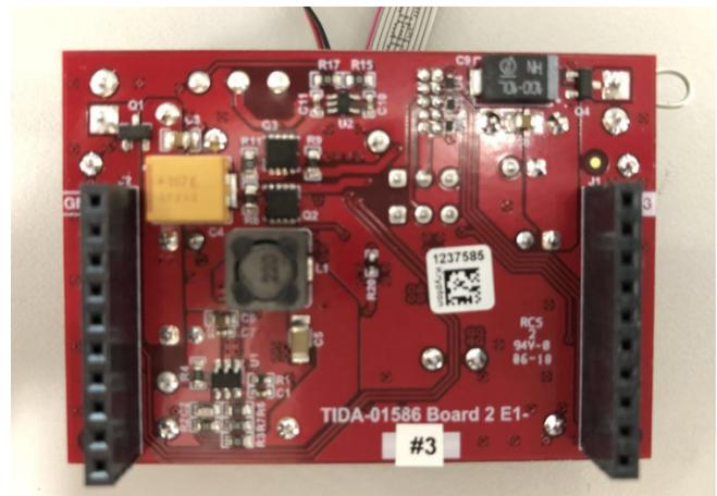
Figure 18. Power and Control Board (Board-2) Back Side
