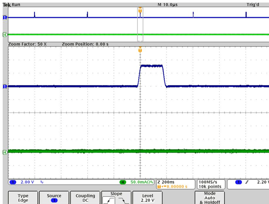
Figure 35. PWM Duty Cycle at 1% for Buck LED Driver
