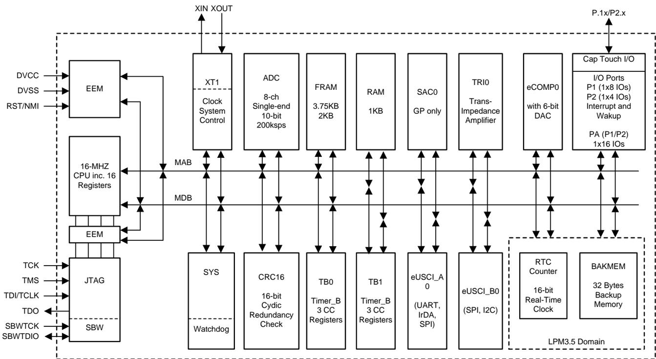
Figure 2. MSP430FR231x Functional Block Diagram
