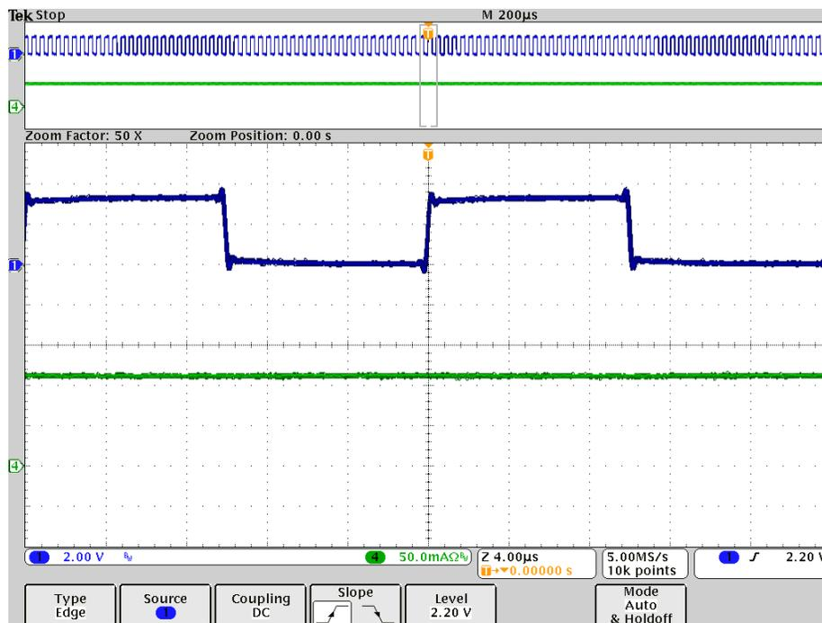
Figure 40. PWM Duty Cycle at 50% for Boost LED Driver
