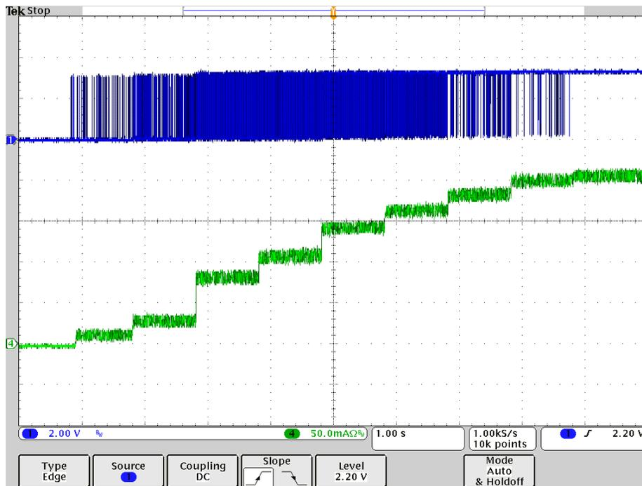
Figure 38. Buck LED Driver From Disable to 100% Duty Cycle
