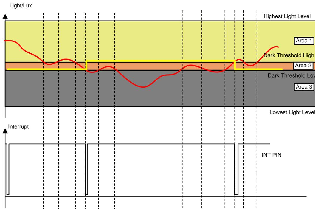
Figure 15. OPT3001 Interrupt Control Method With Light-Level Hysteresis
