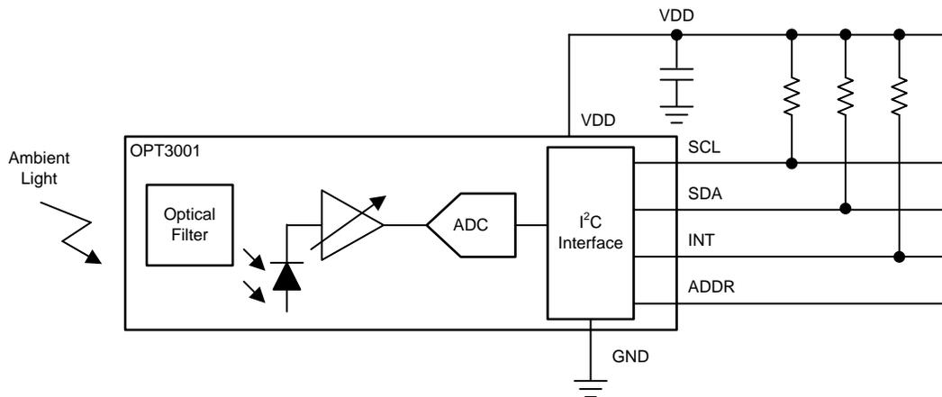
**Figure 6. OPT3001 Functional Block Diagram**
