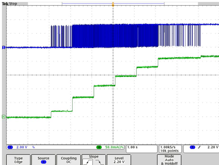
Figure 42. Boost LED Driver From Disabled to 100% Duty Cycle
