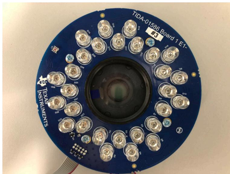
Figure 19. IR LED Array and ALS Board (Board-1)
