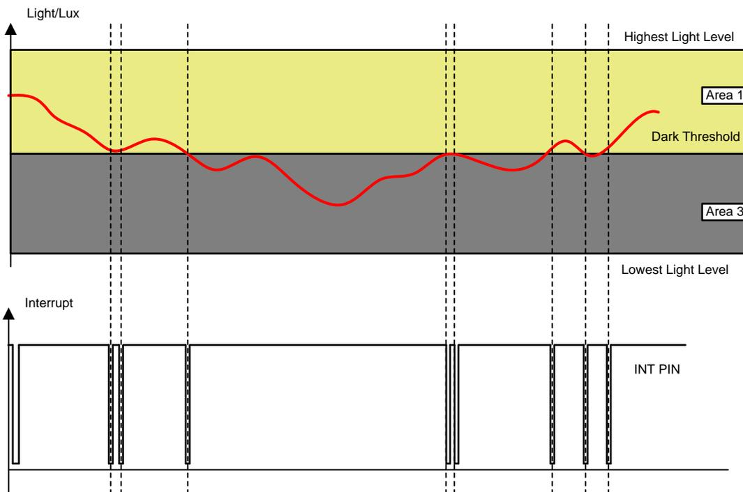
Figure 14. OPT3001 Interrupt Control Method Without Light-Level Hysteresis
