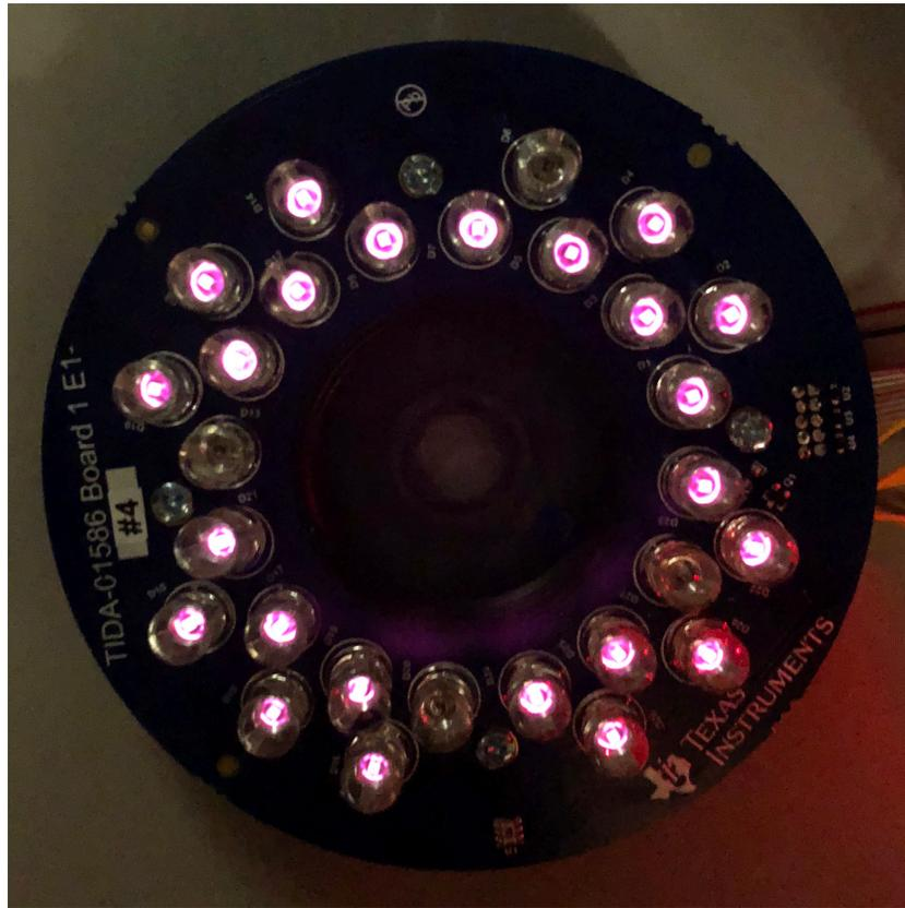
Figure 33. IR LEDs illumination Without Ballasting
