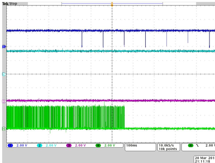
Figure 31. Ambient Light Level From LED Dimming Area to LED Disabled Area
