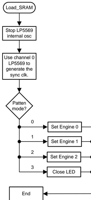
Figure 9. Load SRAM Flowchart
