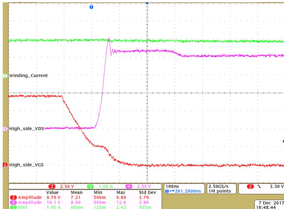
Figure 21. High-Side FET Turnoff: High-Side  $V_{GS}$  and  $V_{DS}$  at 2-A Winding Current
