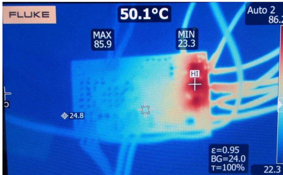
Figure 25. Thermal Image of Board With Sinusoidal Control at 2.37-A<sub>RMS</sub> Winding Current
