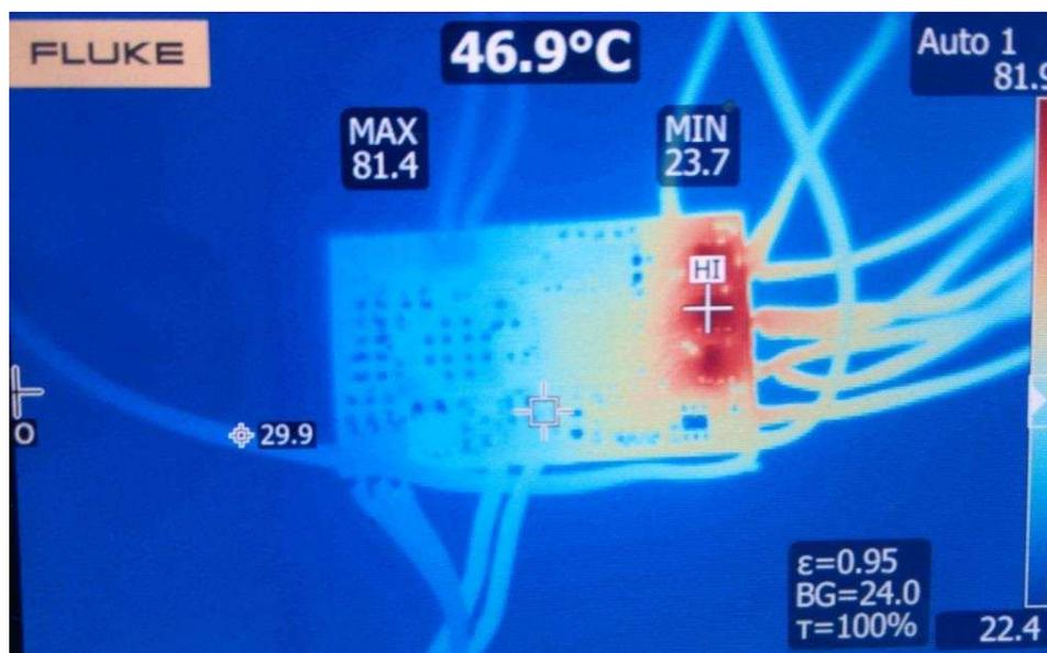
**Figure 23. Thermal Image of Board With Trapezoidal Control at 2.28-A<sub>RMS</sub> Winding Current, 100% Duty Cycle**
