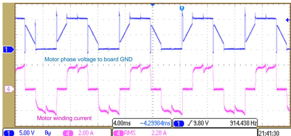
**Figure 22. Load Test Results With Trapezoidal Control at 2.28-A<sub>RMS</sub> Winding Current, 100% Duty Cycle**
