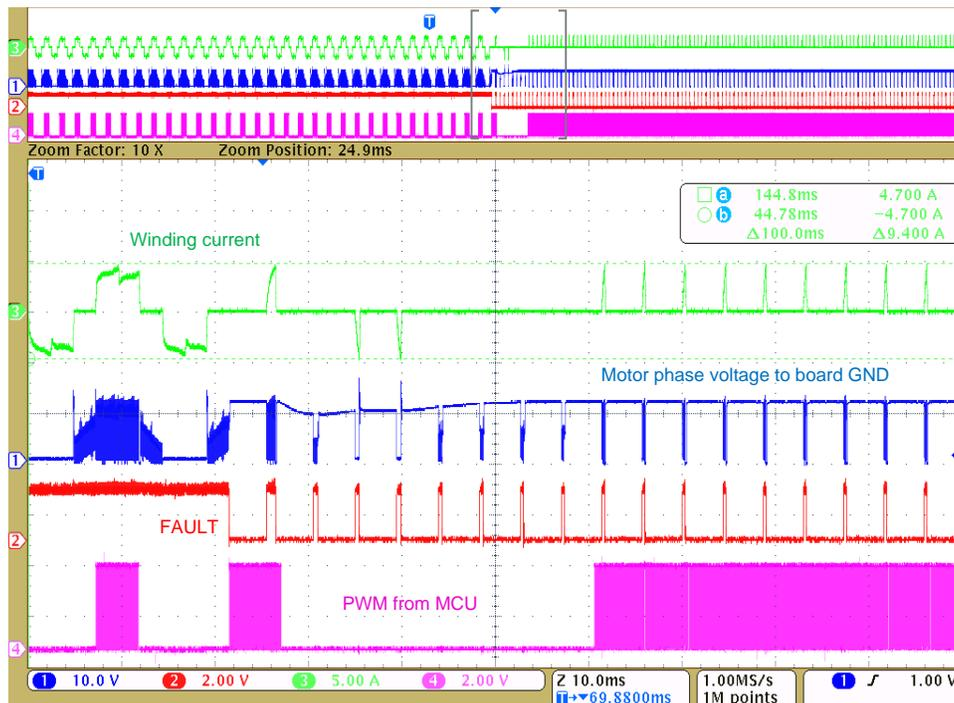
Figure 27. Overcurrent Protection With MOSFET  $V_{DS}$  Monitoring
