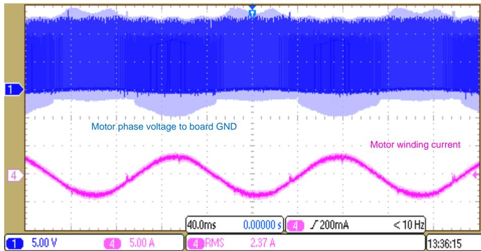
Figure 24. Load Test Results With Sinusoidal Control at 2.37-A<sub>RMS</sub> Winding Current
