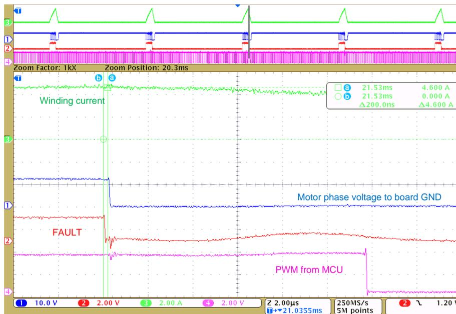
Figure 28. Zoomed View of Overcurrent Protection With MOSFET  $V_{DS}$  Monitoring
