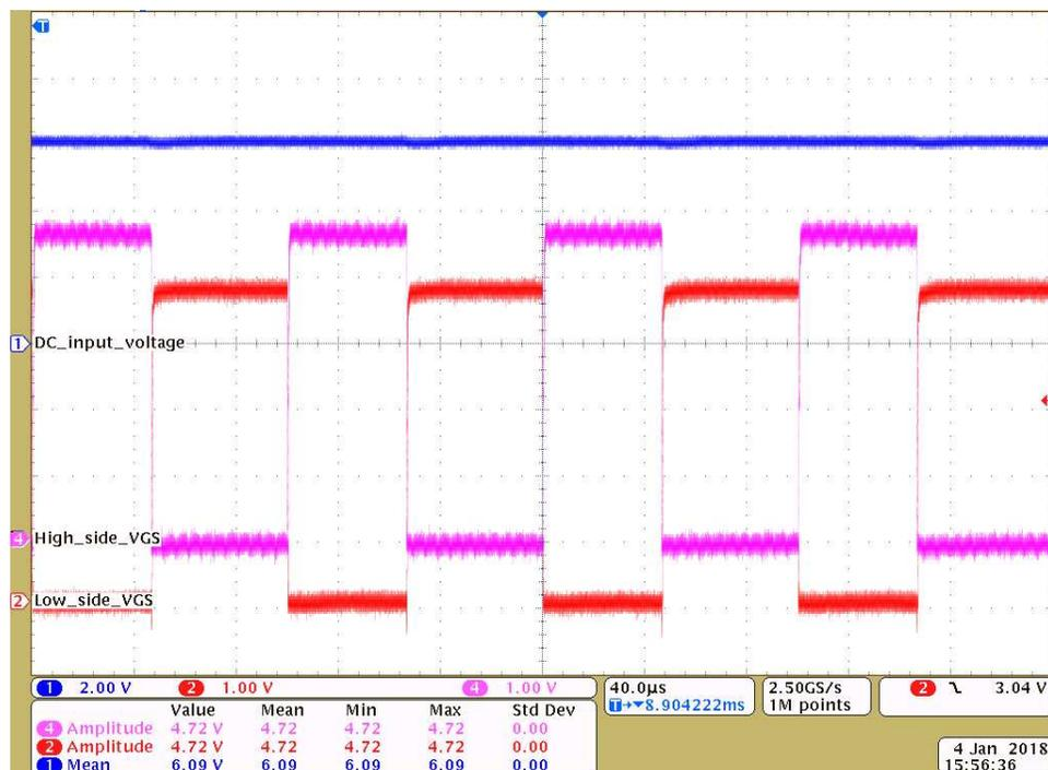
Figure 14. Low-Side and High-Side Gate Drive Voltage at 6-V DC
