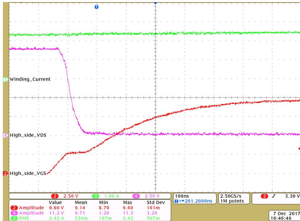
Figure 20. High-Side FET Turnon: High-Side  $V_{GS}$  and  $V_{DS}$  at 2-A Winding Current
