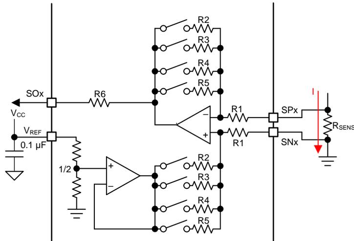
Figure 6. DRV8304 Current Sense Amplifier
