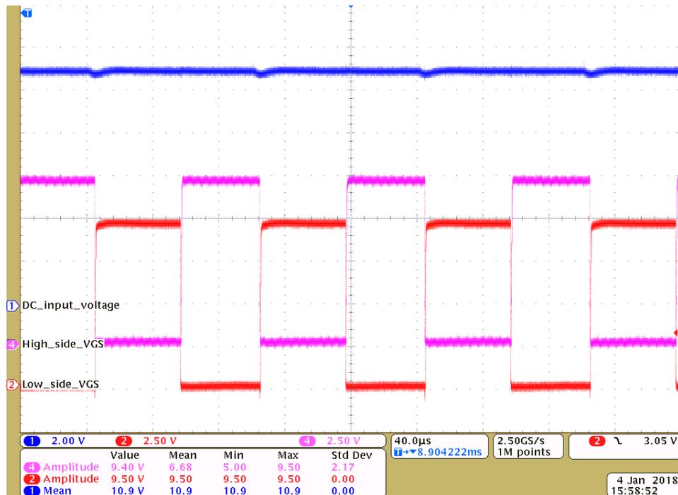
Figure 13. Low-Side and High-Side Gate Drive Voltage at 10.8-V DC
