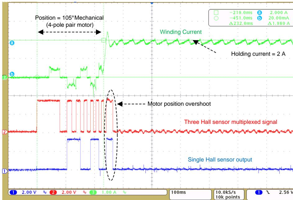
Figure 29. Test Results for Position Control at 105° Mechanical
