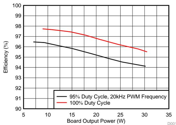
**Figure 26. Power Stage Efficiency versus Output Power**
