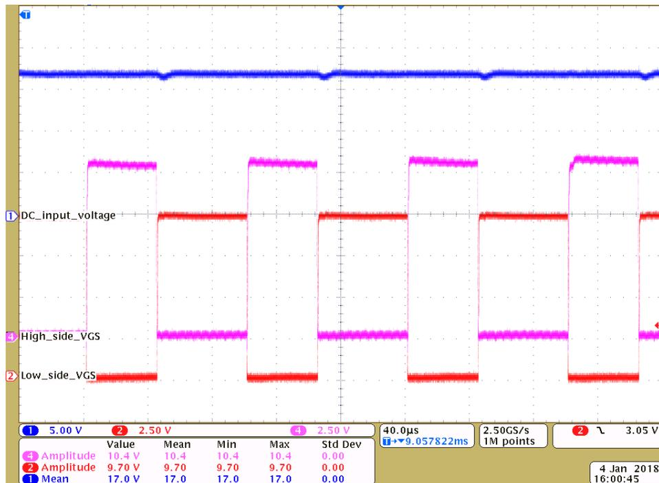
Figure 15. Low-Side and High-Side Gate Drive Voltage at 17-V DC
