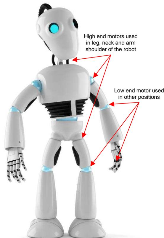
**Figure 1. Typical Humanoid—Motor Drive Locations**
