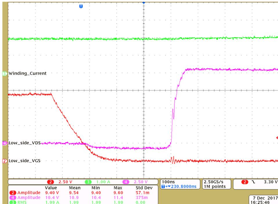
Figure 19. Low-Side FET Turnoff: Low-Side  $V_{GS}$  and  $V_{DS}$  at 2-A Winding Current
