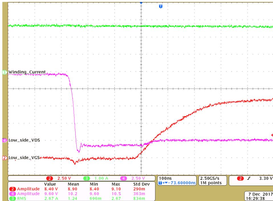
Figure 18. Low-Side FET Turnon: Low-Side  $V_{GS}$  and  $V_{DS}$  at 2-A Winding Current
