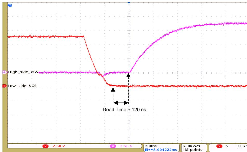
**Figure 17. Dead Time at Trailing Edge of Low-Side  $V_{GS}$**
