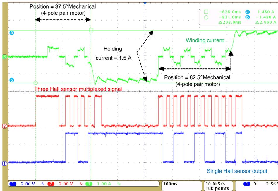
Figure 30. Test Results for Position Control With a Step Change in Position Reference
