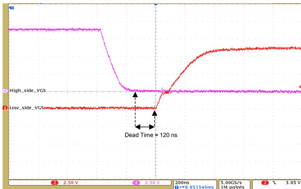
Figure 16. Dead Time at Rising Edge of Low-Side  $V_{GS}$
