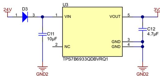
Figure 12. Schematic of TPS7B6933
