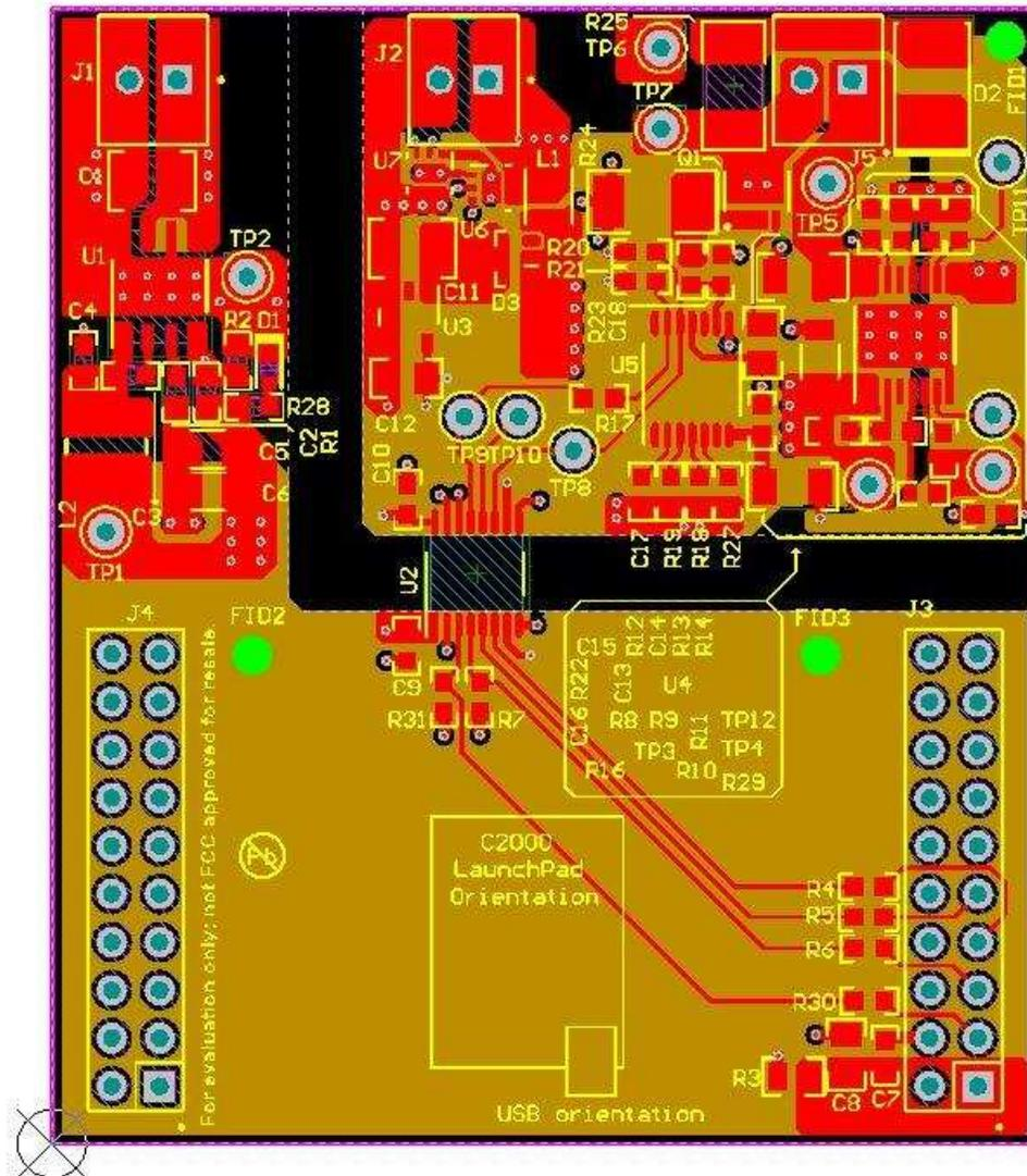
Figure 25. Isolation Barrier and Power Plane of Layout
