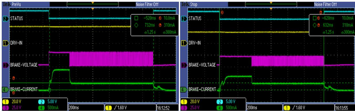
Figure 16. Hold Current of Brake Fixed to 300 mA at 19-V and 28-V Input Voltage
