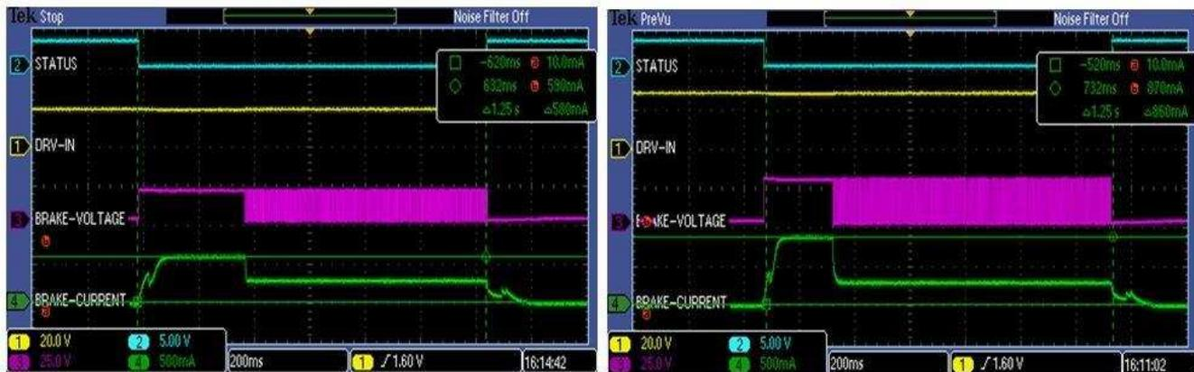
Figure 17. Relative Increase in Peak Current at 19-V and 28-V Input Supply Voltages
