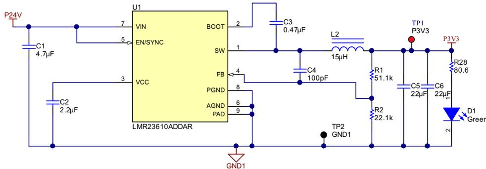
Figure 11. Schematic of LMR23610
