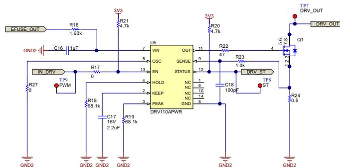
Figure 8. Schematic of Low-Side Current Controller
