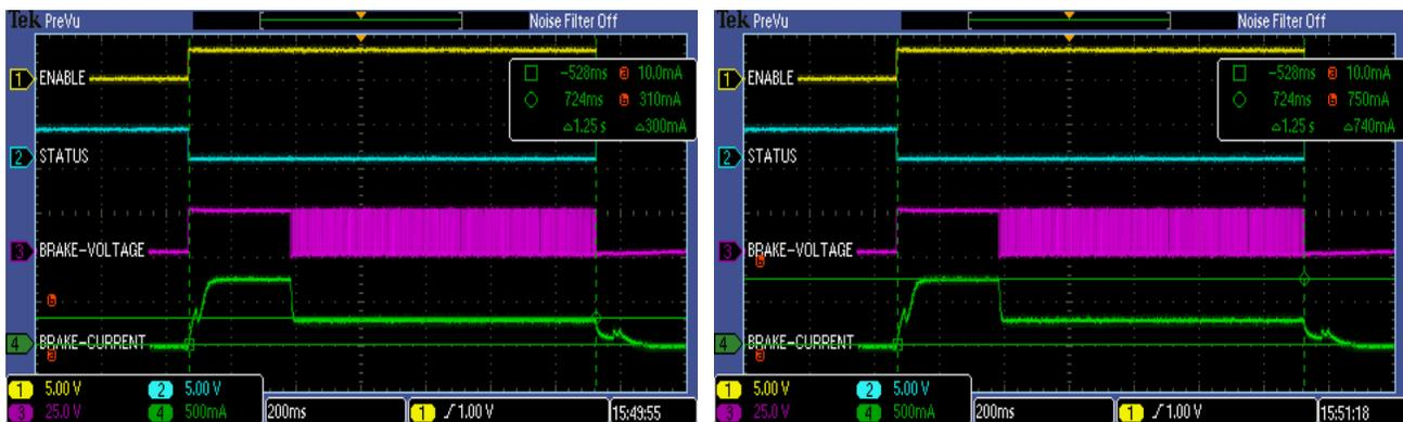
Figure 14. Hold and Peak Currents of Brake Coil
