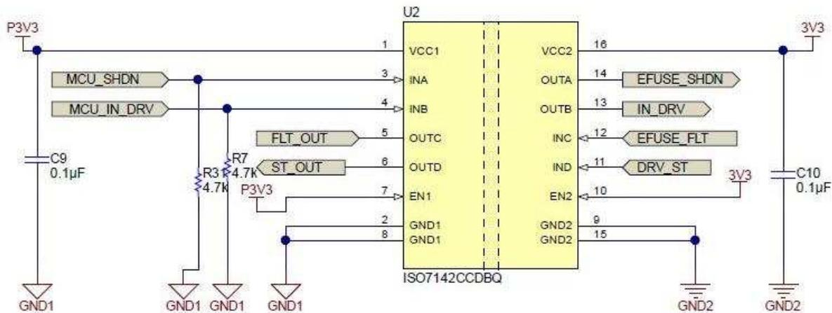
Figure 6. Schematic of ISO7142
