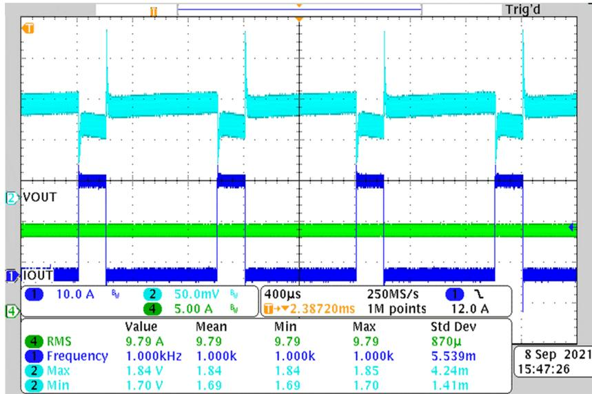
Figure 3-4. Load Transient Behavior
