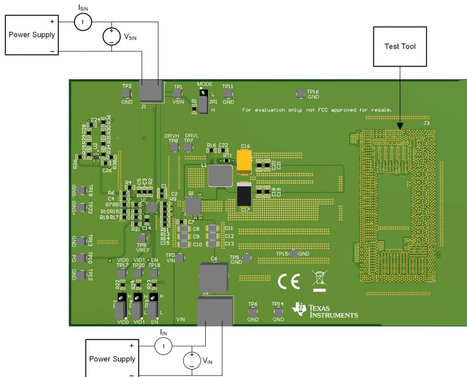
Figure 3-1. Test Setup
