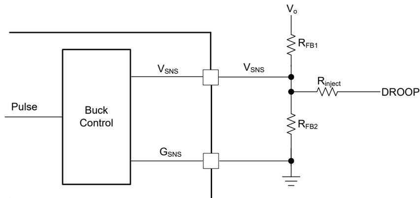
Figure 2-6. Resistor Network for Voltage Scaling
