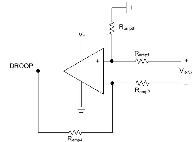
Figure 2-5. Operational Amplifier for Subtraction
