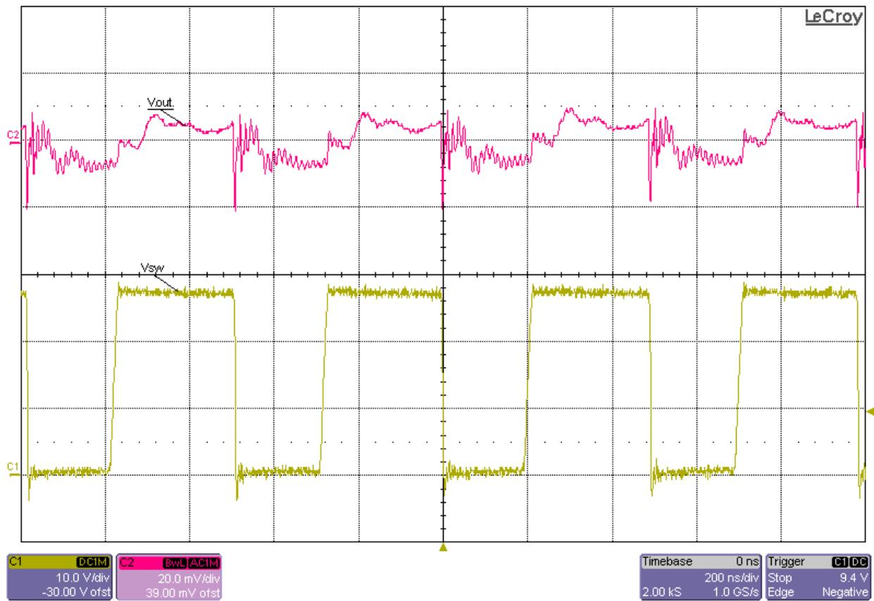
Switch Node Voltage and Output Voltage Ripple at 16Vin and 0.4A Load (Vripple ≈ 30mVp-p)
