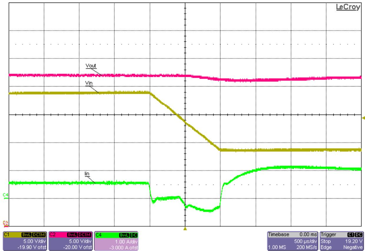
**Line Transient from 24Vin to 13.5Vin (0.4A Constant-Current Load on the output)**
