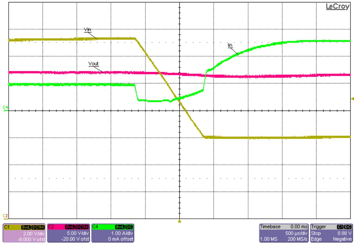
Line Transient from 13.5Vin to 6Vin (0.4A Constant-Current Load on the output)
