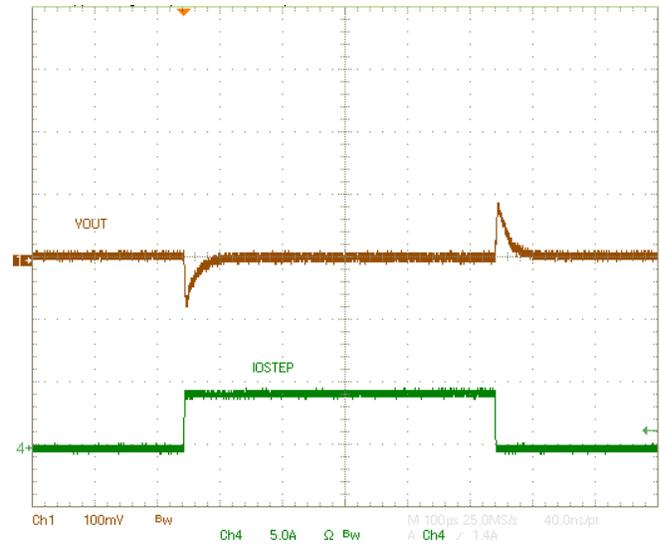
Figure 13. EVM Transient Waveform
