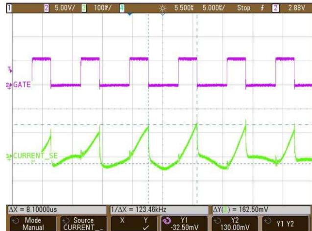
Figure 29. Current Sense Waveform With Gate Drive at Full Load ( $V_{OUT} = 80\text{ V}$ ,  $I_{OUT} = 160\text{ mA}$ )
