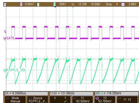
Figure 38. Output Voltage Ripple at the Negative Rail at 50-V Full Load
