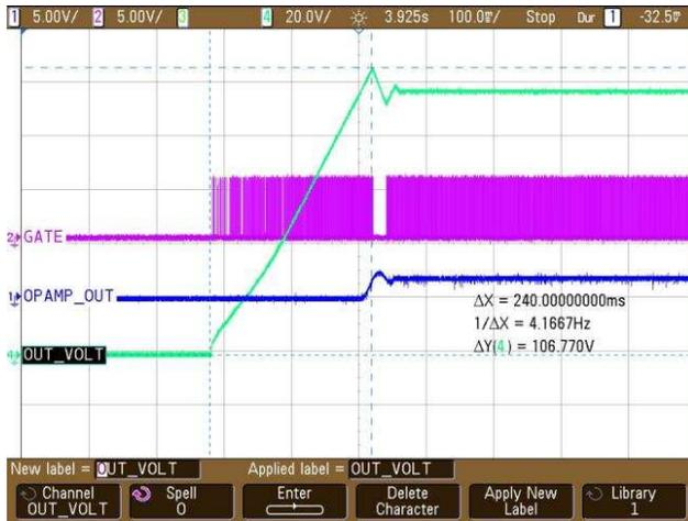
Figure 58. Soft Start at Set Voltage of 100 V
