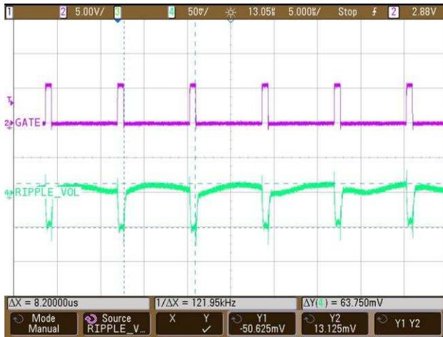
Figure 44. Output Voltage Ripple at the Positive Rail at 10 V, 300-mA Load
