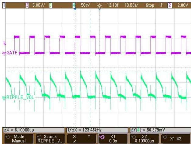
**Figure 23. Output Voltage Ripple at the Positive Rail at 100-V Full Load**
