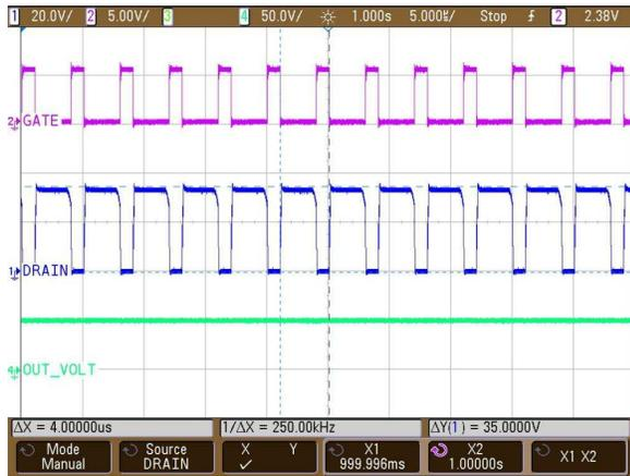
**Figure 62. Gate, Drain, and Output Voltage Waveforms for Synchronization to 250-kHz External Clock**
