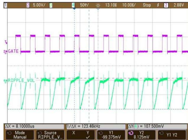
**Figure 24. Output Voltage Ripple at the Negative Rail at 100-V Full Load**
