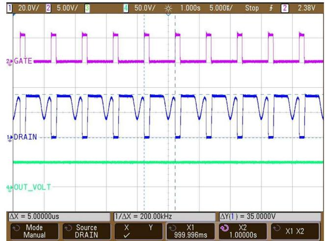
**Figure 61. Gate, Drain, and Output Voltage Waveforms for Synchronization to 200-kHz External Clock**
