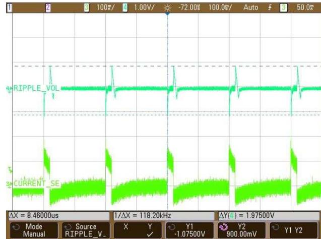
Figure 55. Ripple Voltage for Elastography Mode at  $V_{OUT} = 100$  V,  $I_{OUT} = 125$  mA
