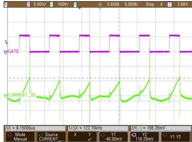
**Figure 22. Current Sense Waveform With Gate Drive at Full Load ( $V_{OUT} = 100\text{ V}$ ,  $I_{OUT} = 125\text{ mA}$ )**
