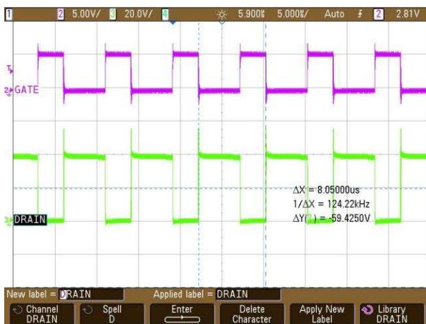
Figure 28. Stress on the Drain of the MOSFET With Gate Drive at Full Load ( $V_{OUT} = 80\text{ V}$ ,  $I_{OUT} = 160\text{ mA}$ )
