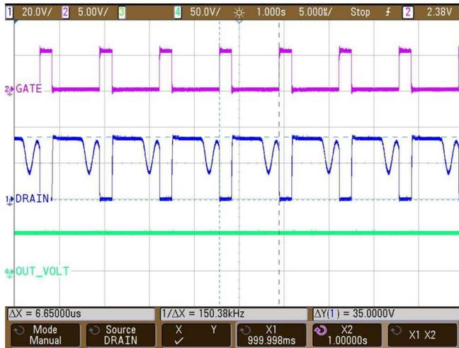
**Figure 60. Gate, Drain, and Output Voltage Waveforms for Synchronization to 150-kHz External Clock**
