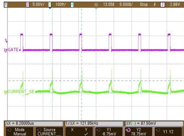
Figure 43. Current Sense Waveform With Gate Drive at 300-mA Load ( $V_{OUT} = 10\text{ V}$ ,  $I_{OUT} = 300\text{ mA}$ )
