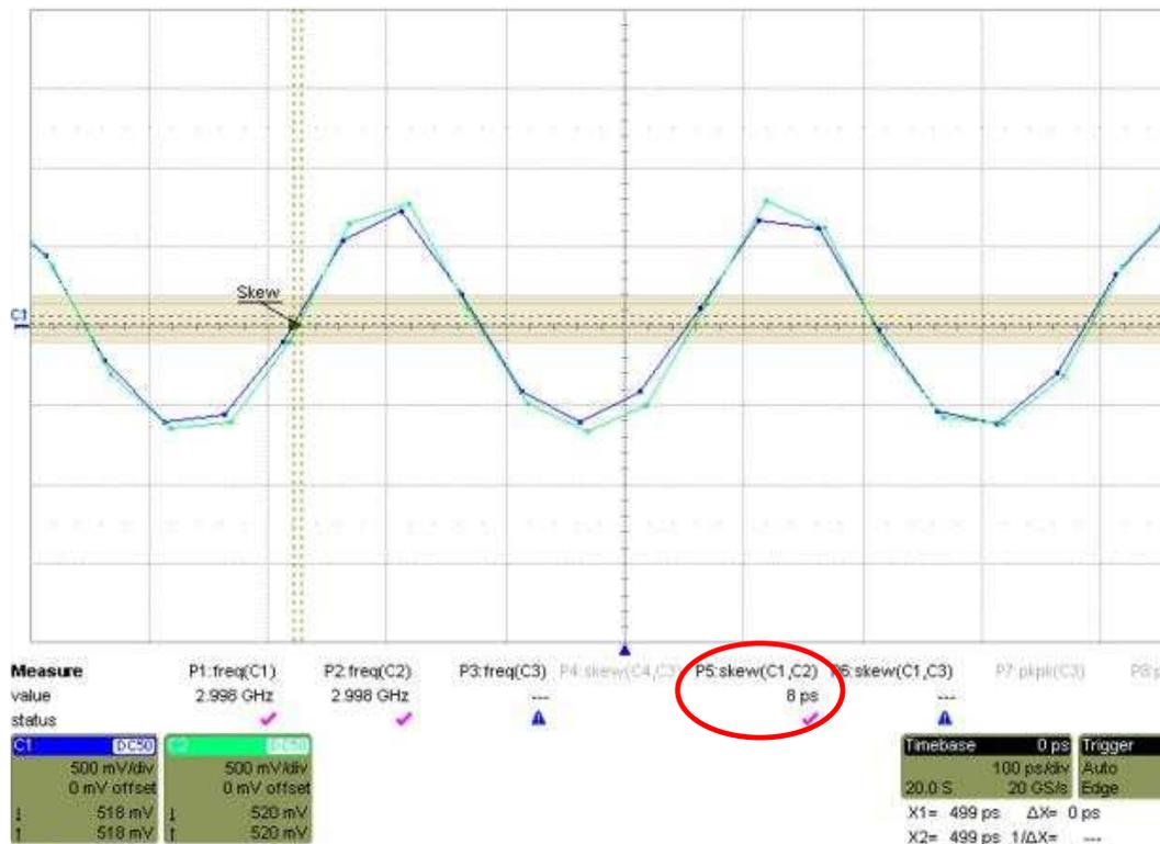
Figure 13. Board-to-Board Clock Measured Skew
