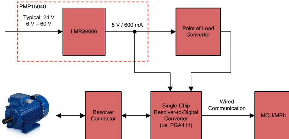
**Figure 2. PMP15040 Rotary Encoder Block Diagram**
