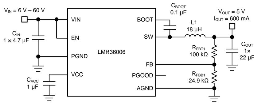
**Figure 6. LMR36006 Schematic**
