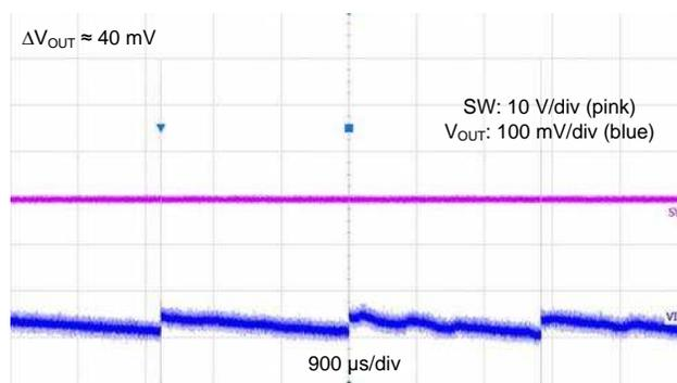
**Figure 23.  $V_{IN} = 60 \text{ V}$ ,  $I_{OUT} = 0 \text{ A}$**
