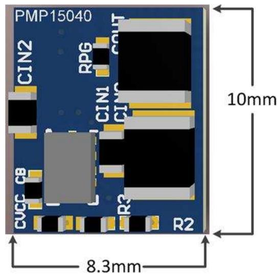
Figure 11. PMP15040 Board Dimensions
