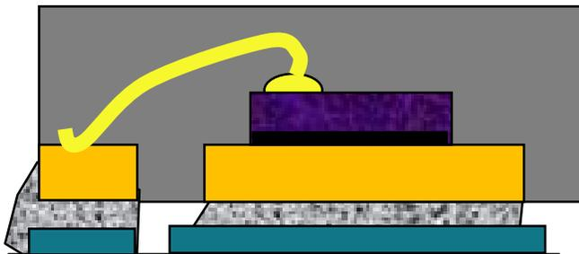
**Figure 7. Standard QFN Package**
