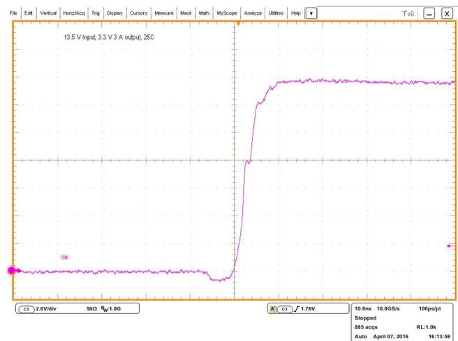
**Figure 10. FCOL QFN Device Switch Node Signal**
