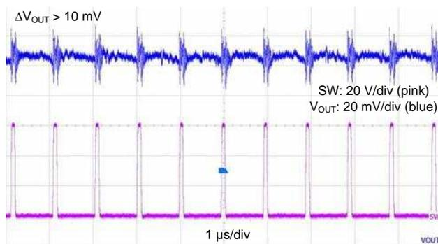
**Figure 24.  $V_{IN} = 60 \text{ V}$ ,  $I_{OUT} = 600 \text{ mA}$**
