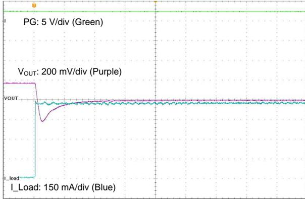
**Figure 25. Load Transient:  $I_{OUT} = 0\text{ A}$  to  $600\text{ mA}$ ,  $V_{IN} = 24\text{ V}$ ,  $t_R = 1\text{ A}/\mu\text{s}$**
