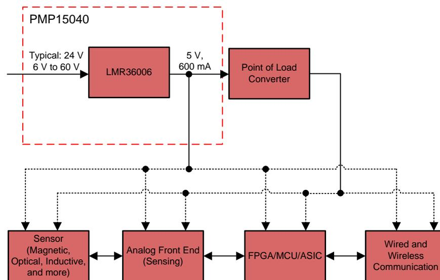
**Figure 1. PMP15040 Field Transmitter Block Diagram**
