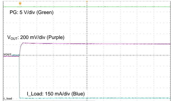
**Figure 26. Load Transient:  $I_{OUT} = 600\text{ mA}$  to  $0\text{ A}$ ,  $V_{IN} = 24\text{ V}$ ,  $t_F = 1\text{ A}/\mu\text{s}$**
