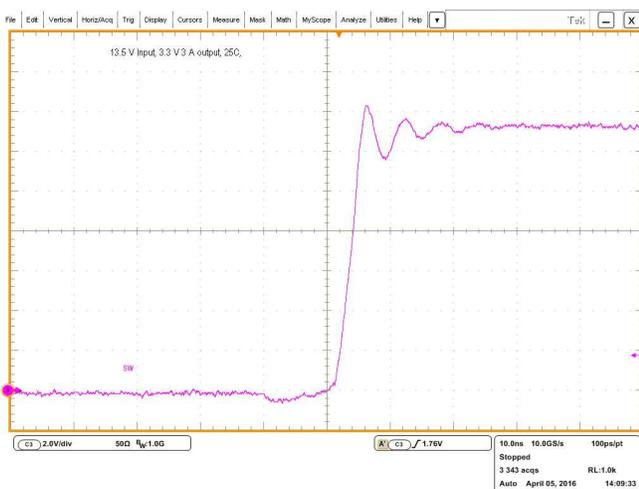
**Figure 9. Wirebond Device Switch Node Signal**
