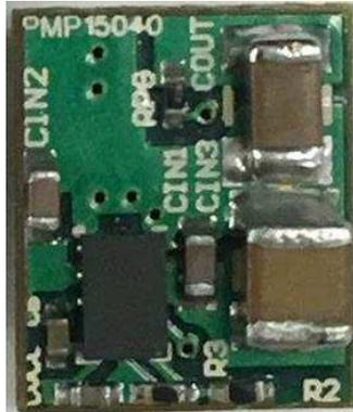
Figure 4. Front of the PMP15040 Board
