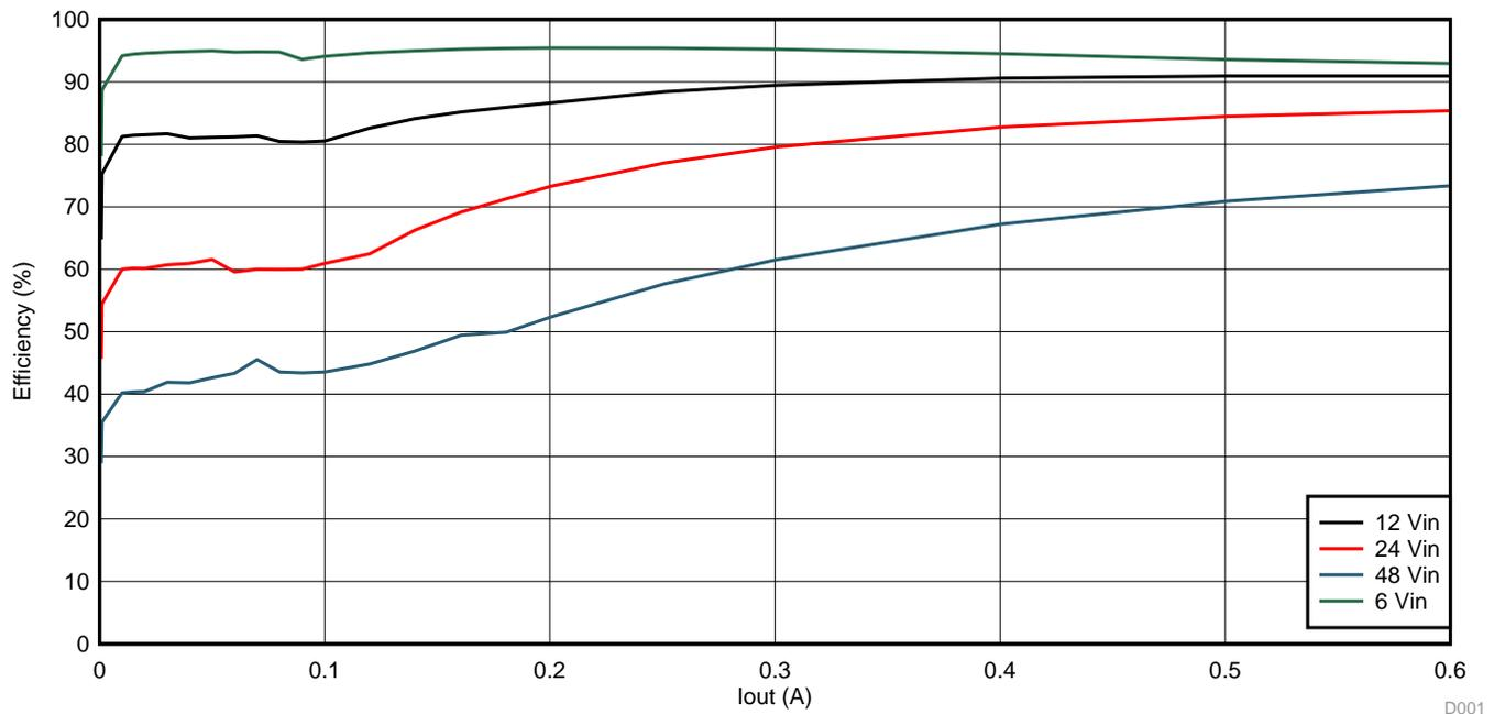
Figure 18. Efficiency vs. Output Current
