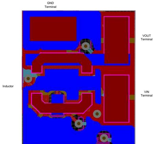
Figure 13. PMP15040 PCB Layout: Bottom Layer
