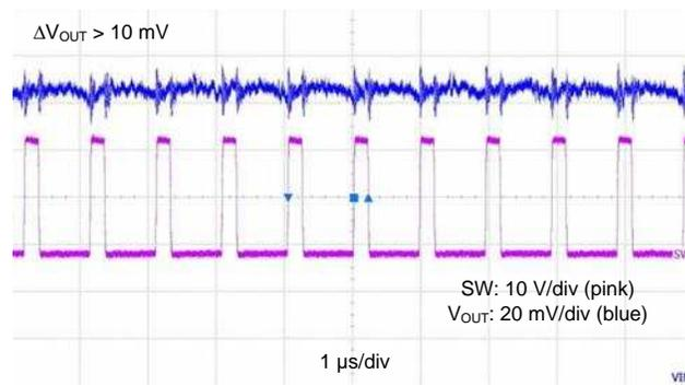
**Figure 22. Steady-State Waveform:  $V_{IN} = 24 \text{ V}$ ,  $I_{OUT} = 600 \text{ mA}$**
