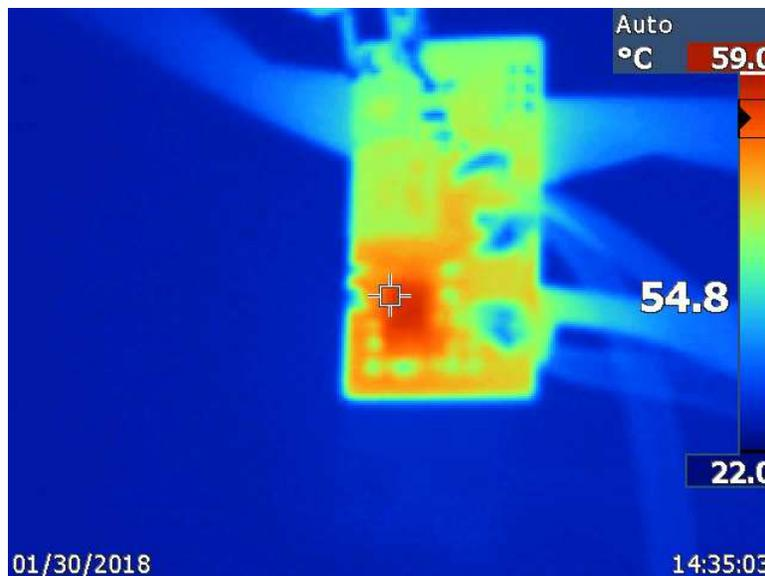
**Figure 8. PMP15039 Thermal Image:  $V_{IN} = 24\text{ V}$ ,  $I_{OUT1} = 300\text{ mA}$ ,  $I_{OUT2} = 1\text{ A}$**
