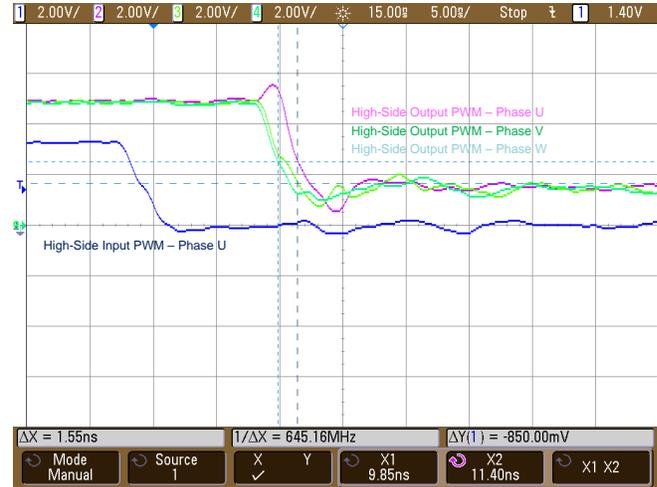
Figure 33. High-Side PWM Propagation Delay Skew—Falling Edge (Measured 1.55 ns)
