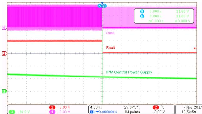
Figure 53. Fault Signal Detection
