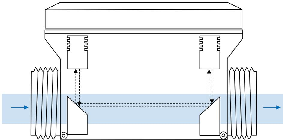
**Figure 11. In-Line and Reflective Transducer Placement**
