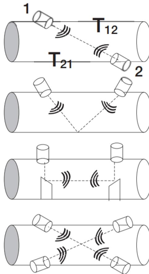
**Figure 12. Various Configurations of In-Line Placement of Transducer Pairs**
