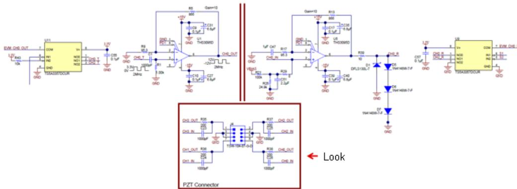
Figure 8. Transducer Pin View for Impedance Matching
