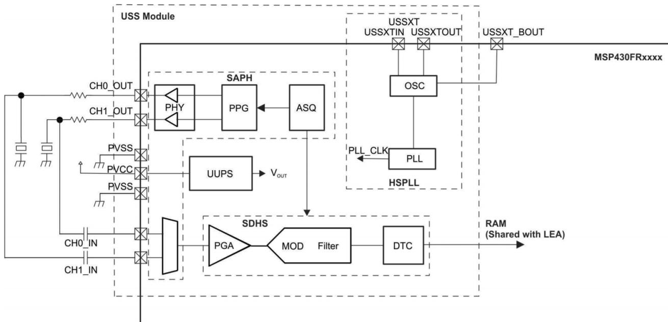
Figure 17. Ultrasonic-Sensing Solution Functional Block Diagram
