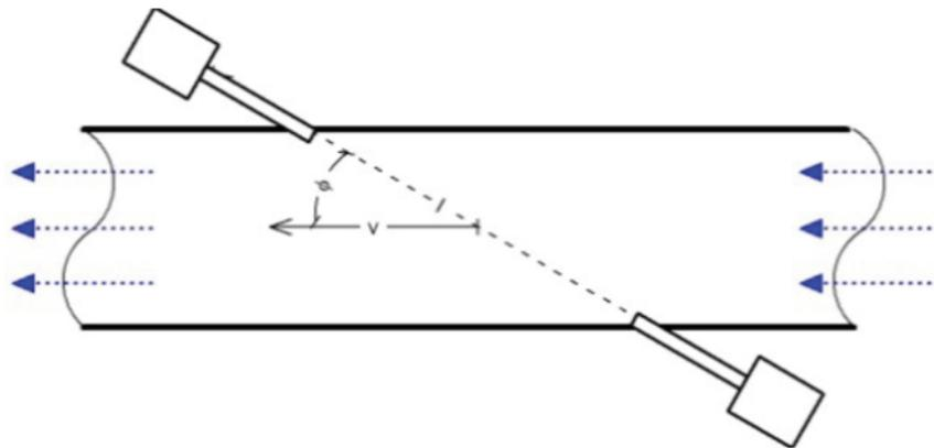
**Figure 10. In-Line and Diagonal Transducer Placement**
