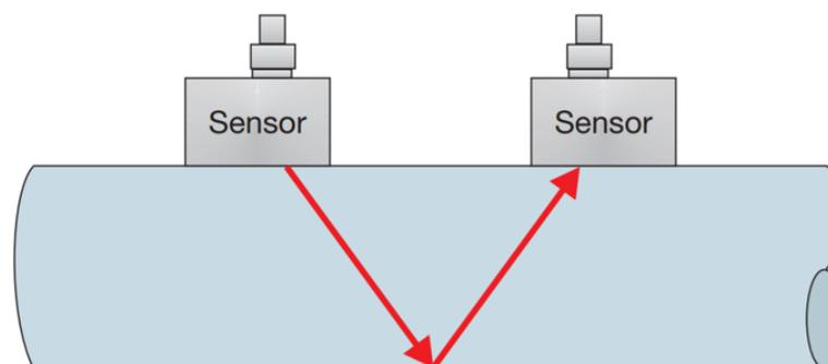
**Figure 13. Clamp-On Transducer Placement**
