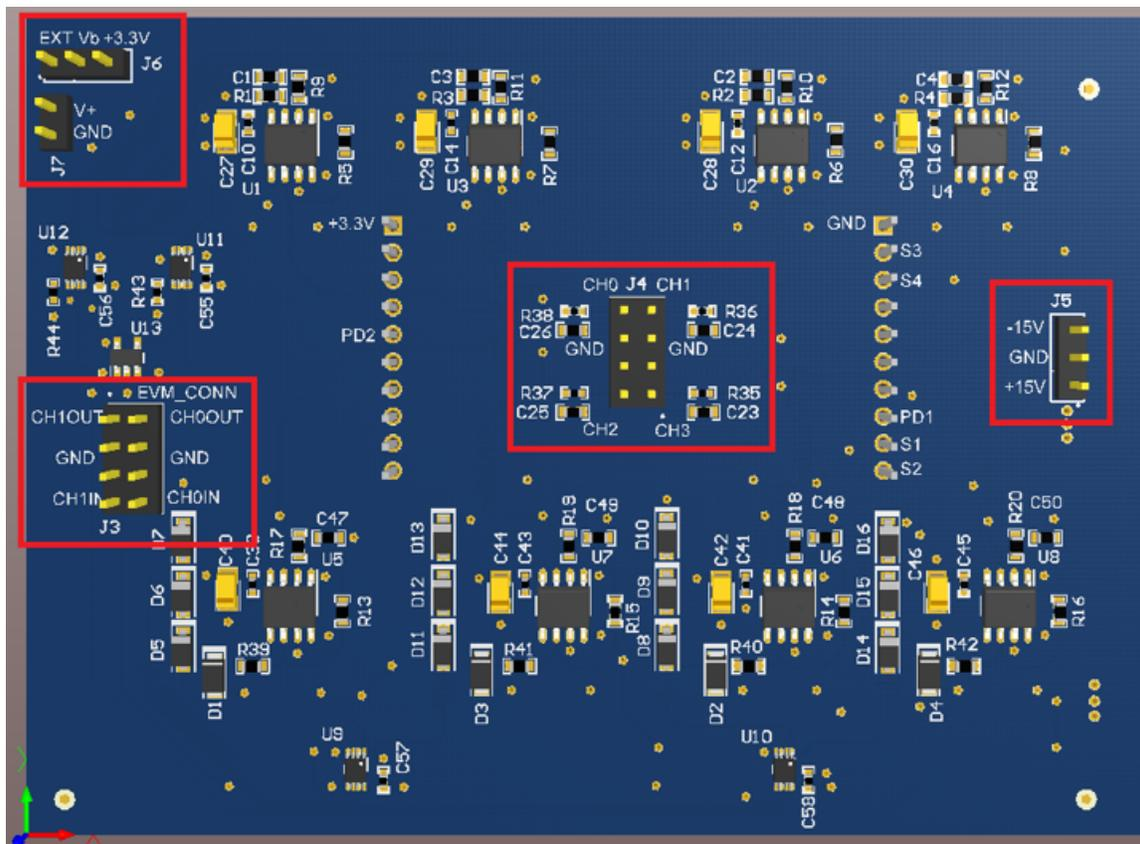
**Figure 19. TIDA-01486 Hardware Configuration**
