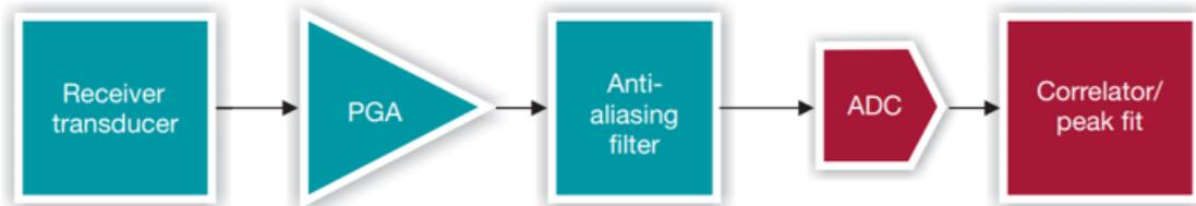
**Figure 15. Correlation-Based Differential TOF Estimator**
