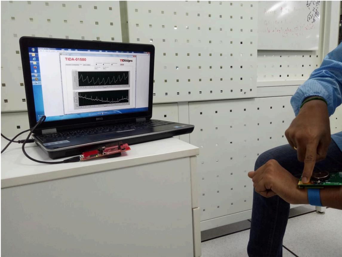
**Figure 3-23. Test Setup for Capturing Data**
