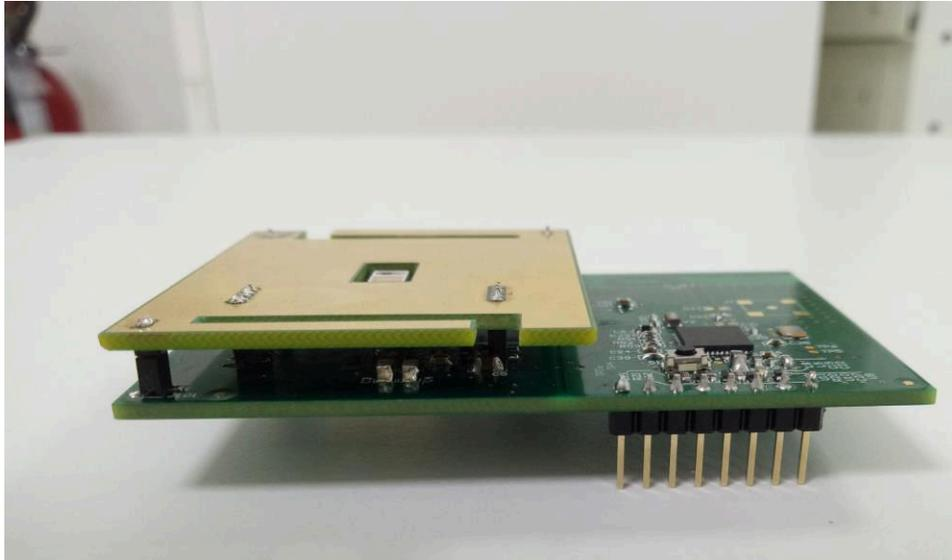
**Figure 3-6. ECG and PPG Board Mounted on Main Board (Side View)**
