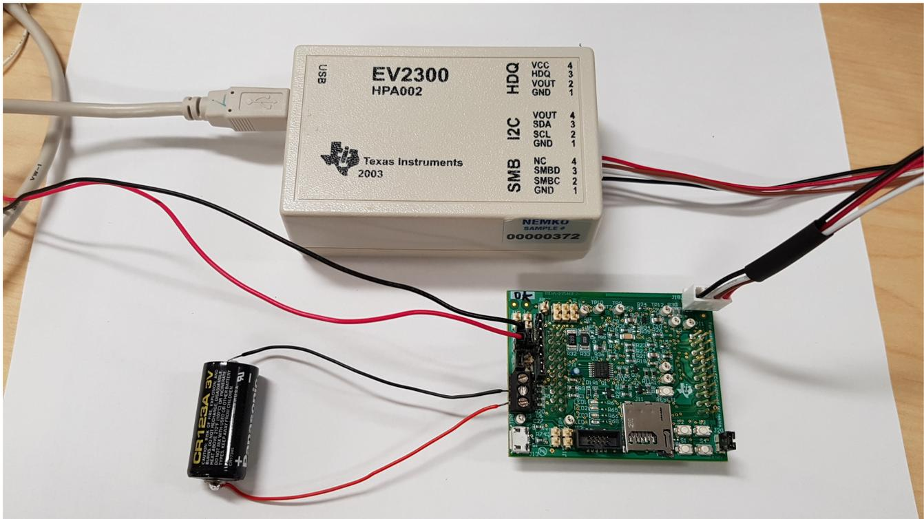
Figure 10. EV2300 and Battery Connection
