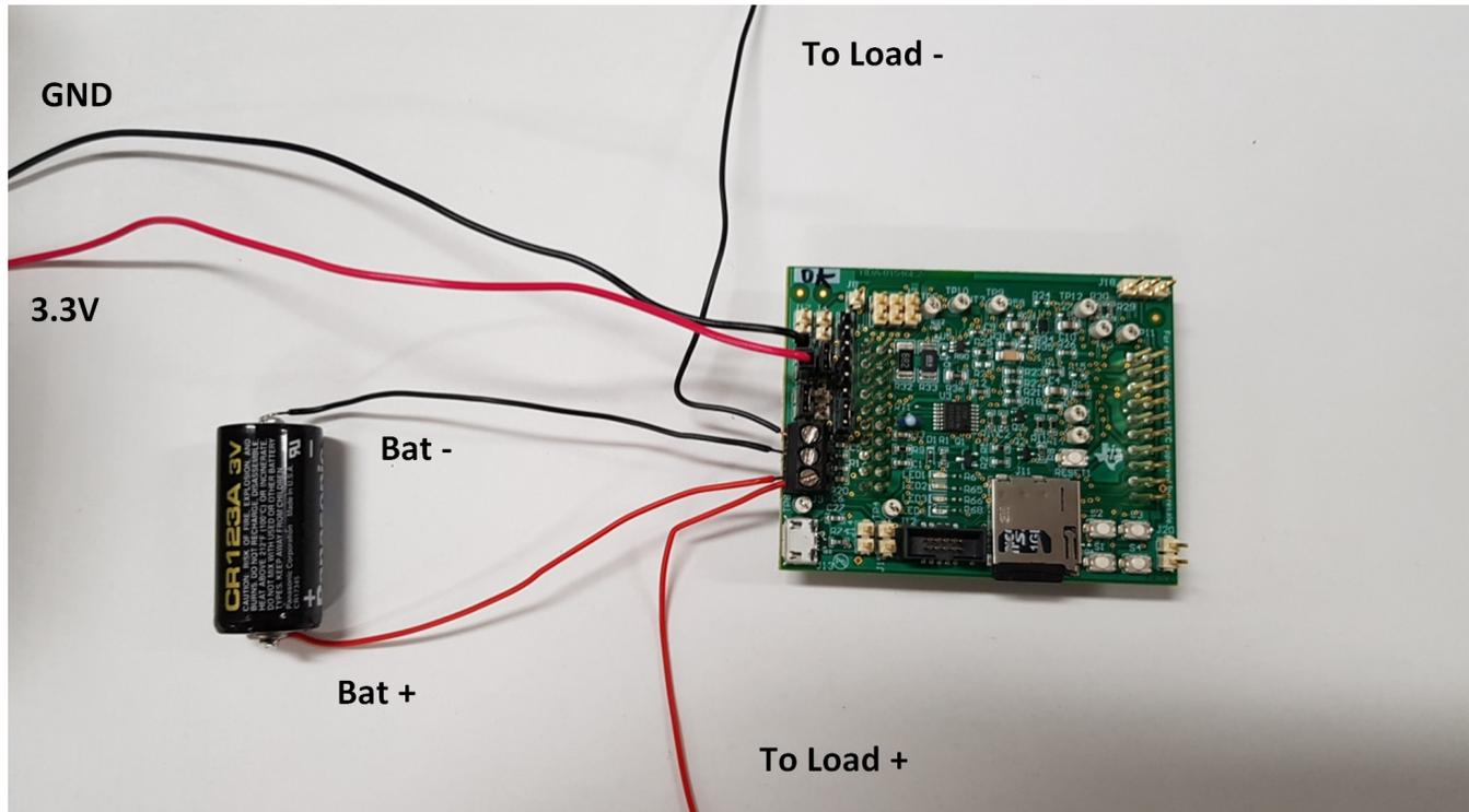
**Figure 12. Battery and Load Connection**
