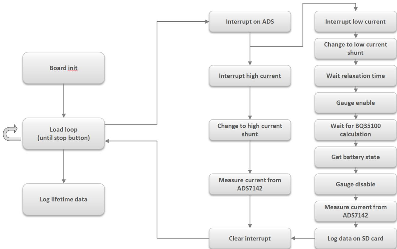
**Figure 3. Flow Chart of SOH Mode Software**
