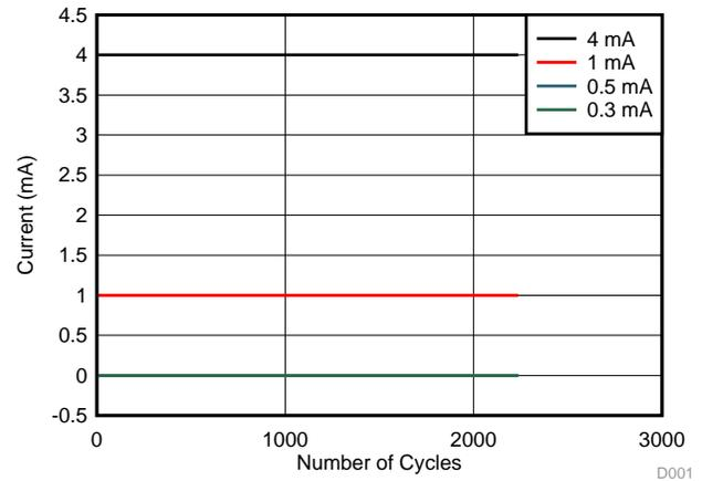
Figure 16. Current Discharge (mA) Measured by Gauge
