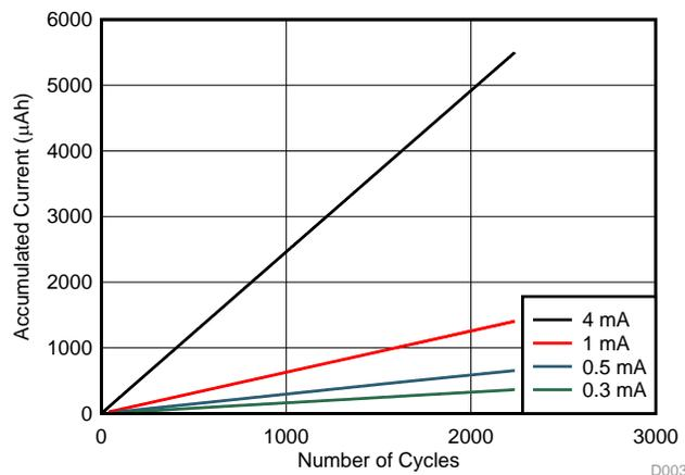
Figure 17. Accumulated Discharge Coulombs ( $\mu\text{Ah}$ ) Measured by Gauge
