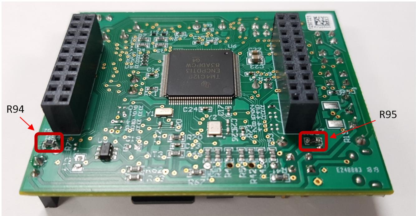
Figure 14. Load Switch Resistance Placement
