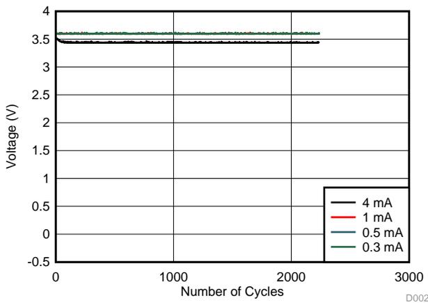
Figure 15. Battery Voltage Measured by Gauge
