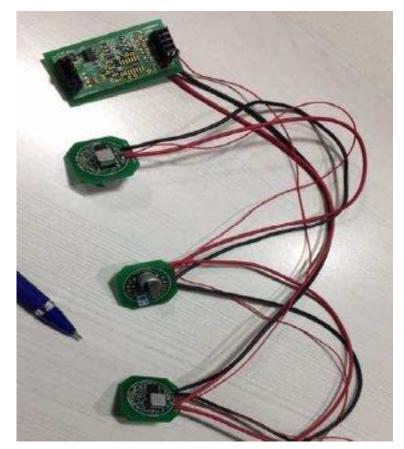
Figure 14. TIDA-01597 System Hardware - Three Sensor Transducer Boards and an OWI Transceiver
