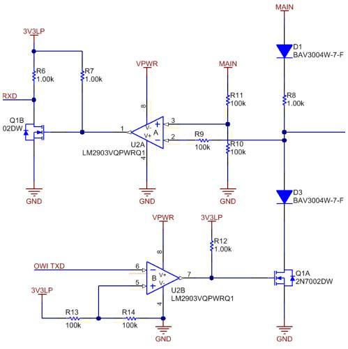
Figure 10. TCI Level Translator Schematic
