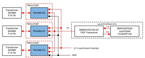
Figure 1. TIDA-0597 Block Diagram
