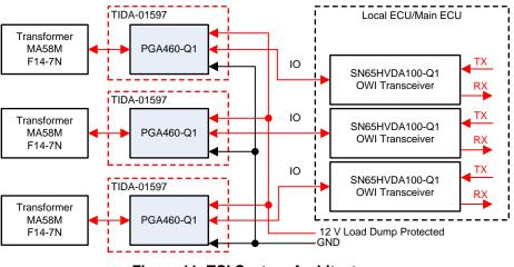
Figure 11. TCI System Architecture
