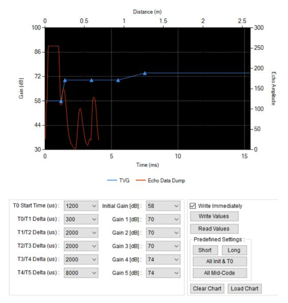
Figure 6. Time-Varying Gain Settings
