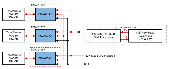
Figure 12. OWI System Architecture
