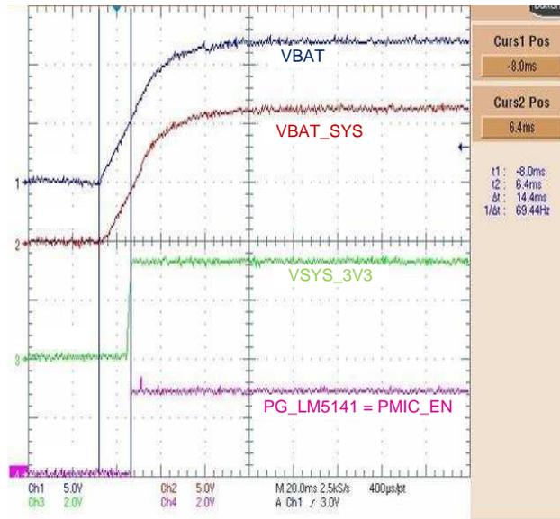
Figure 6. Reference Design Initial Front End Power Up Stage
