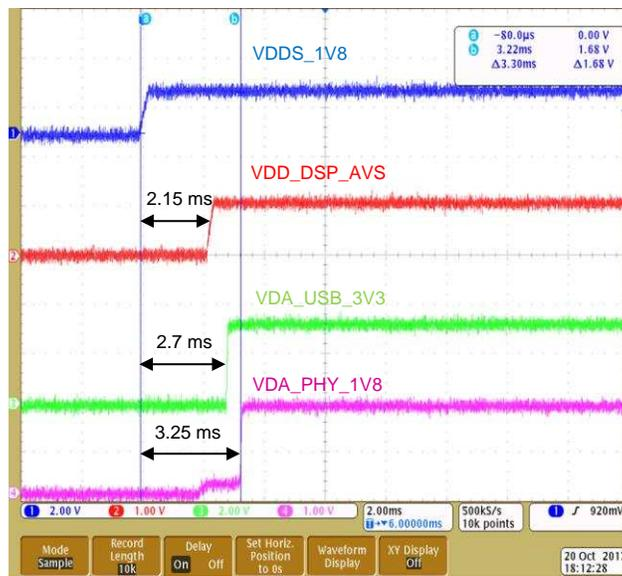
Figure 9. TPS65919 Stages Six to Eight Power Up
