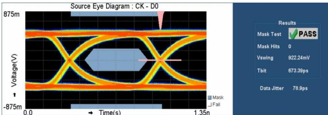
**Figure 5. HDMI Eye Diagram Waveform**
