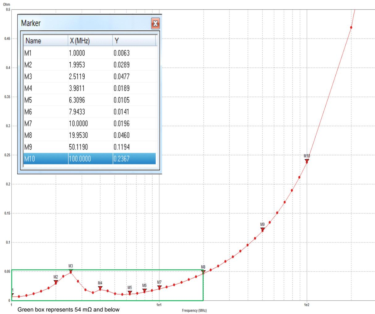
Figure 19. Target Impedance: VDD\_DSP\_AVS
