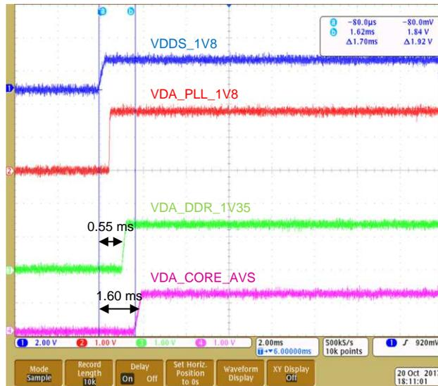
Figure 8. TPS65919 Stages Four and Five Power Up
