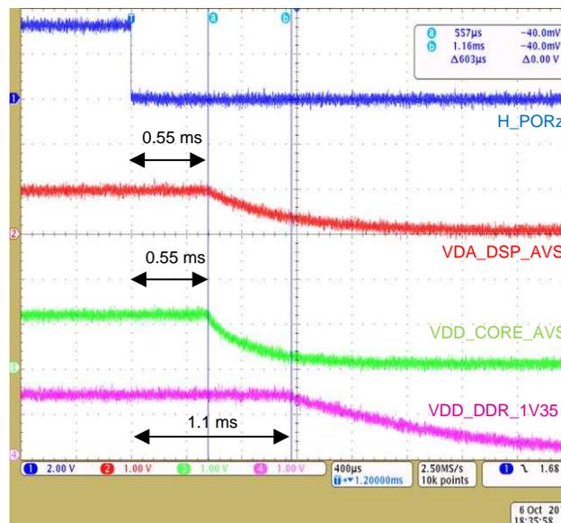
Figure 15. TPS65919 Stage Two and Three Power Down (Continued)
