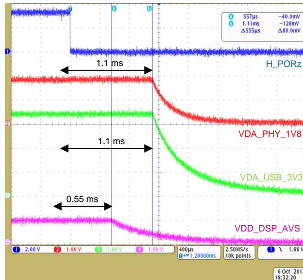
Figure 14. TPS65919 Stage Two and Three Power Down
