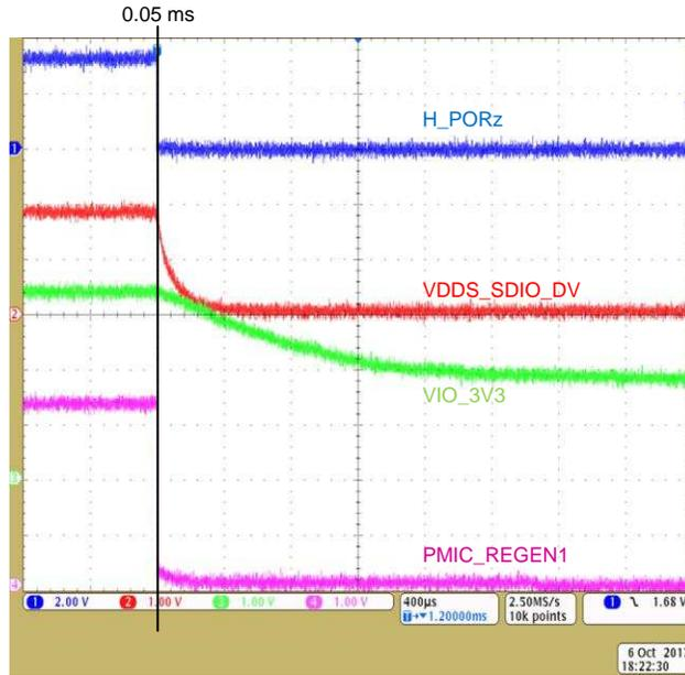
Figure 12. TPS65919 Stage One Power Down
