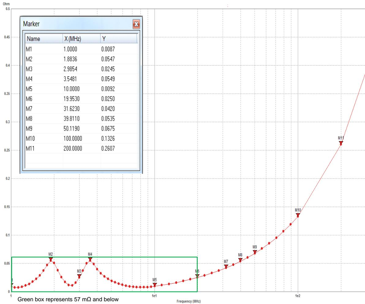
Figure 21. Target Impedance: VDD\_CORE\_AVS
