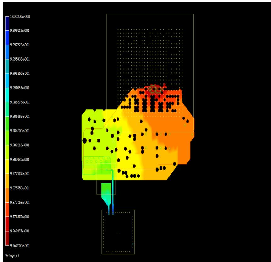
Figure 18. VDD\_DSP\_AVS IR Drop Analysis
