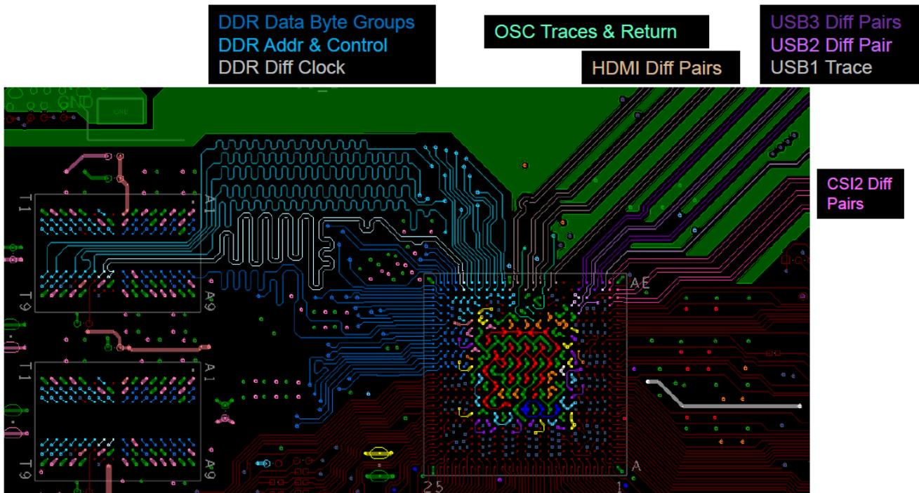
Figure 4. High-Speed Signaling Breakout Overview(Top)
