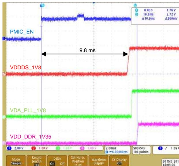
Figure 7. TPS65919 Stages One to Three Power Up
