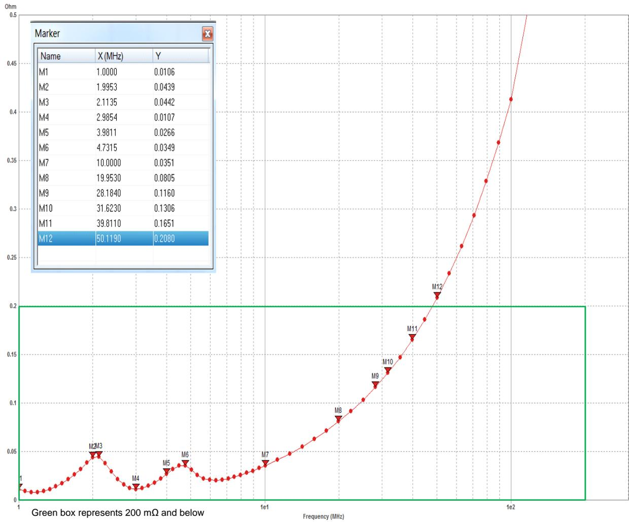
Figure 23. Target Impedance: VDD\_DDR\_1V35
