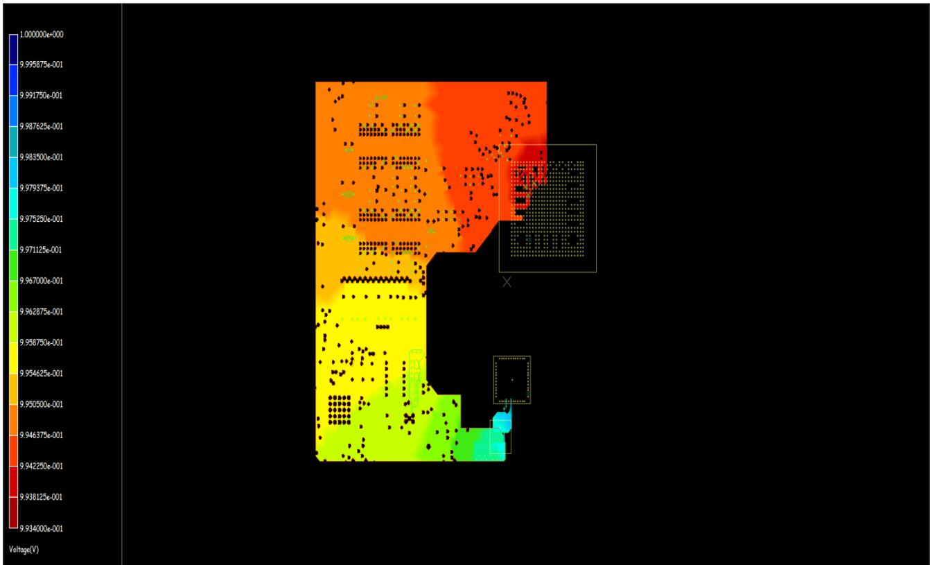
Figure 22. VDD\_DDR\_1V35 IR Drop Analysis
