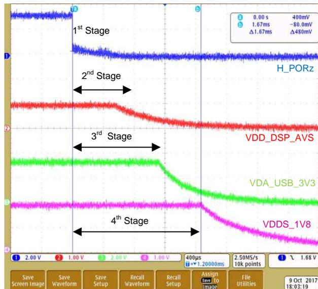
Figure 17. TPS65919 All Four Stages Power Down
