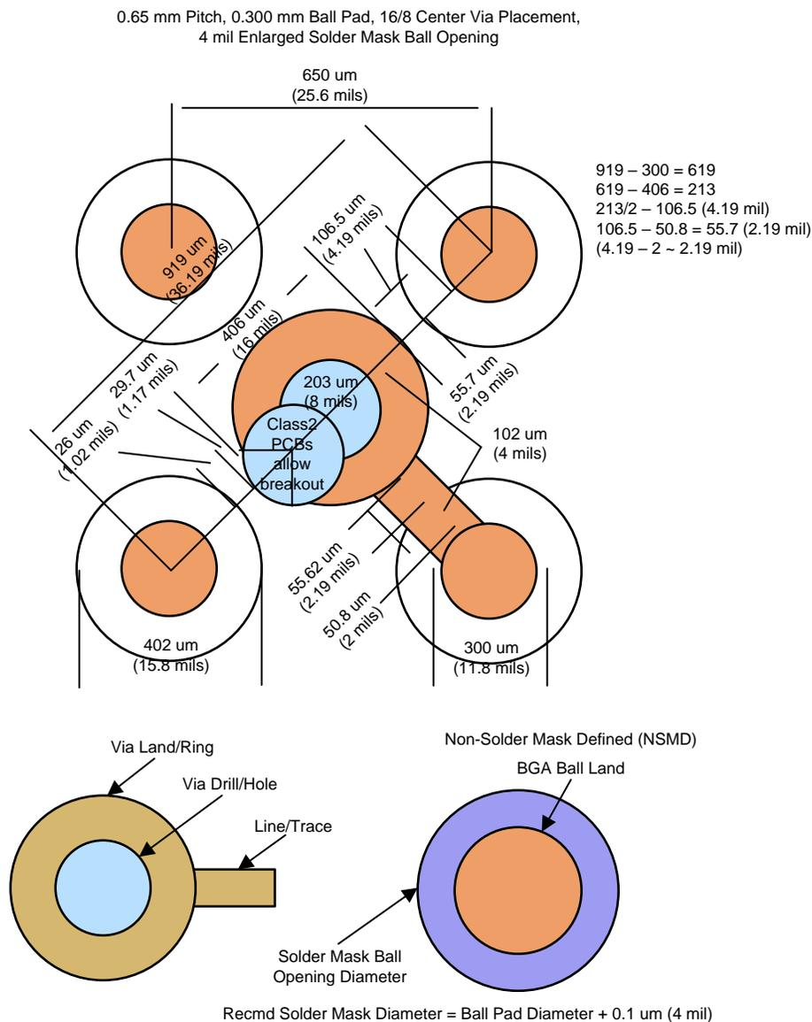
**Figure 2. 16/8 Center Via Placement Breakout Scheme**
