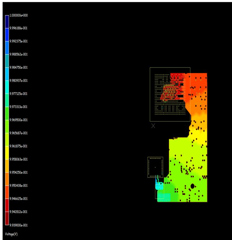
**Figure 20. VDD\_CORE\_AV5 IR Drop Analysis**
