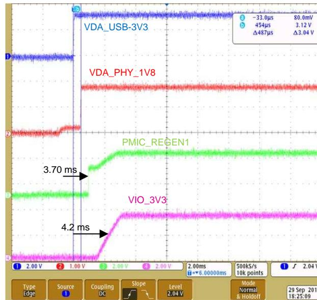
Figure 10. TPS65919 Stages Seven to Ten Power Up
