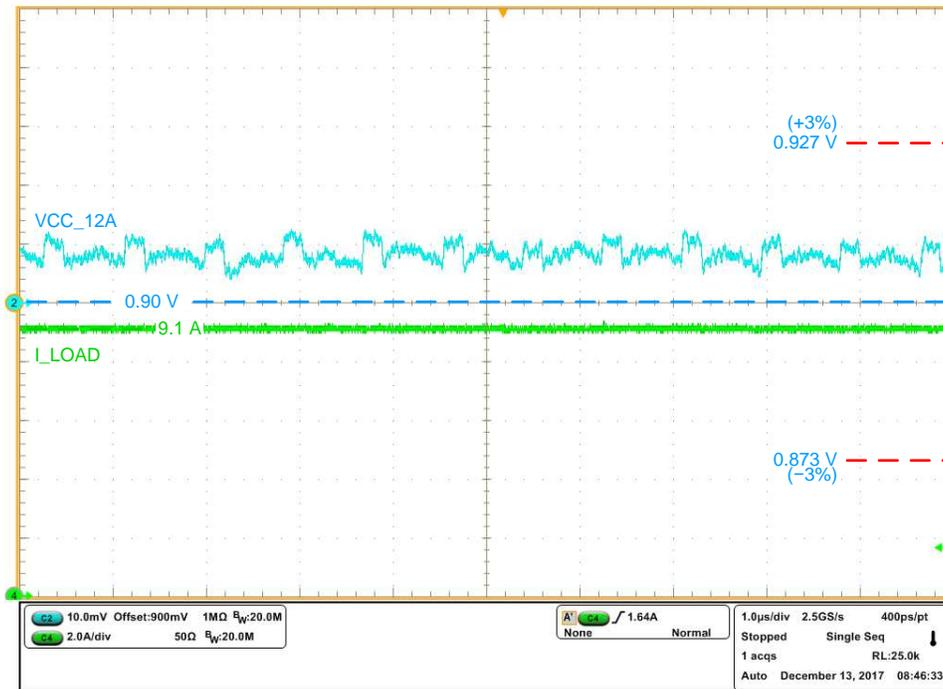
Figure 22. VCC\_12A Full Load Test
