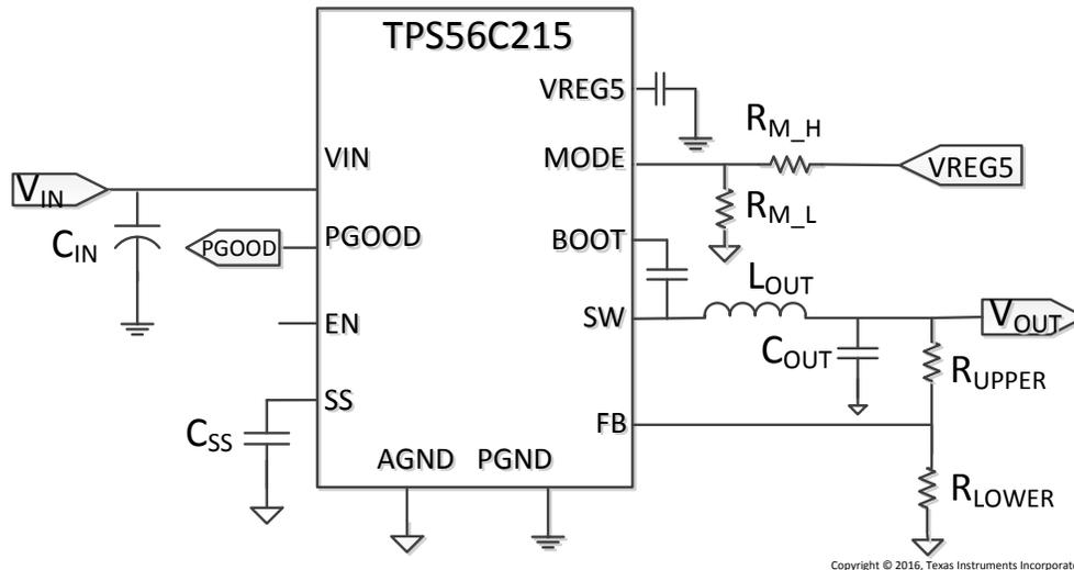
**Figure 8. TPS56C215 Simplified Application Circuit**
