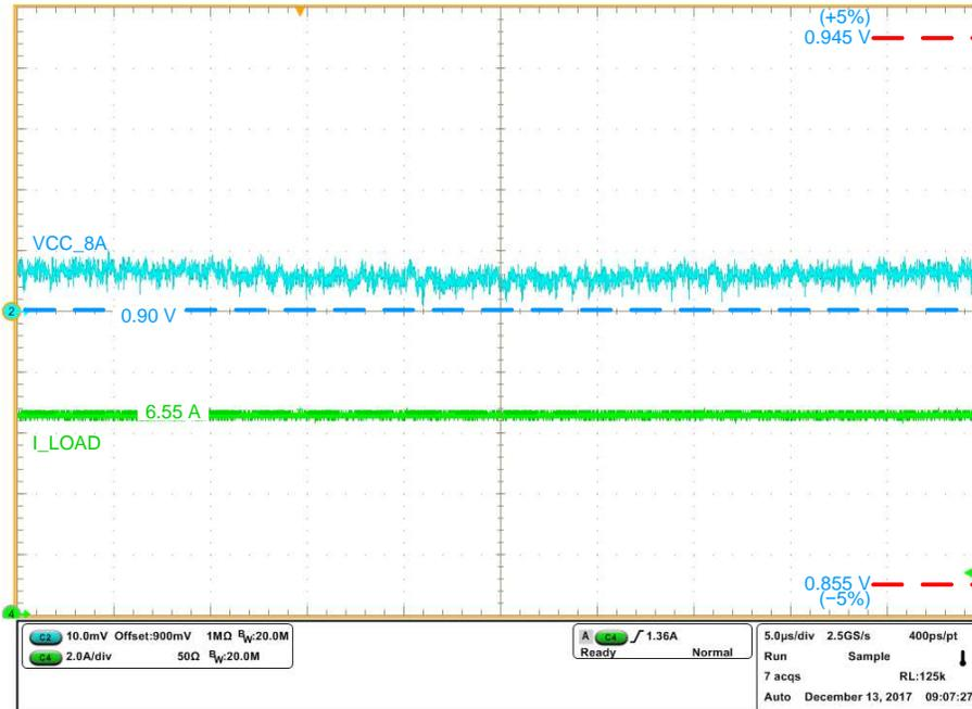
Figure 19. VCC\_8A Full Load Test
