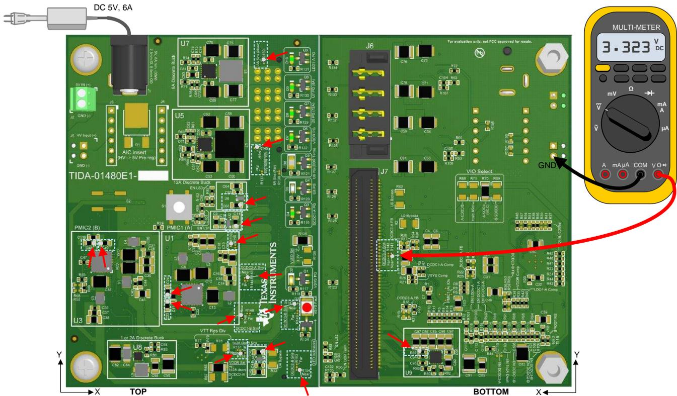
**Figure 13. Setup and Measurement Locations for DC Voltage Measurements**
