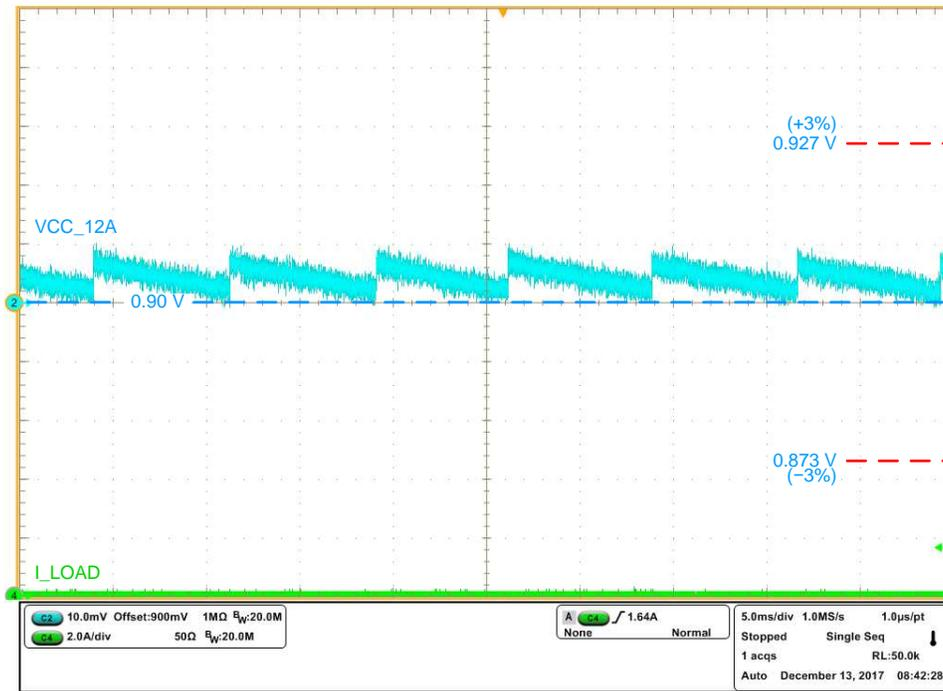
Figure 21. VCC\_12A No Load Test
