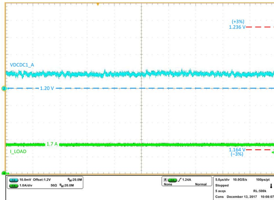
Figure 16. VDCDC1\_A Full Load Test
