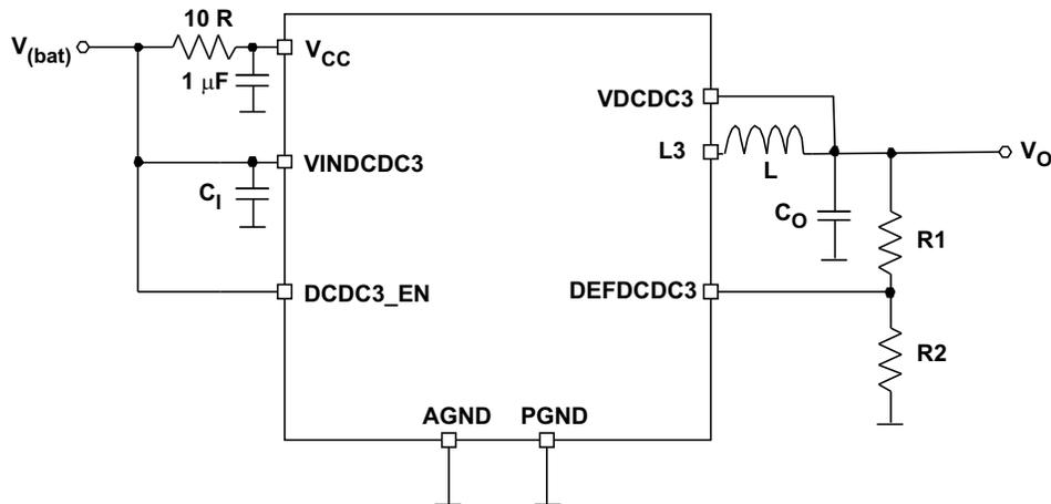
Figure 12. TPS65023 External Resistor Divider for DCDC3
