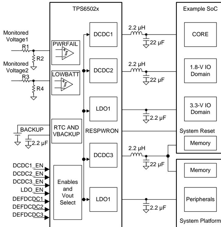
Figure 7. TPS65023 Simplified Application Circuit
