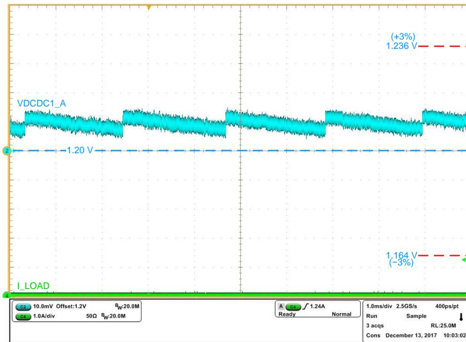
Figure 15. VDCDC1\_A No Load Test
