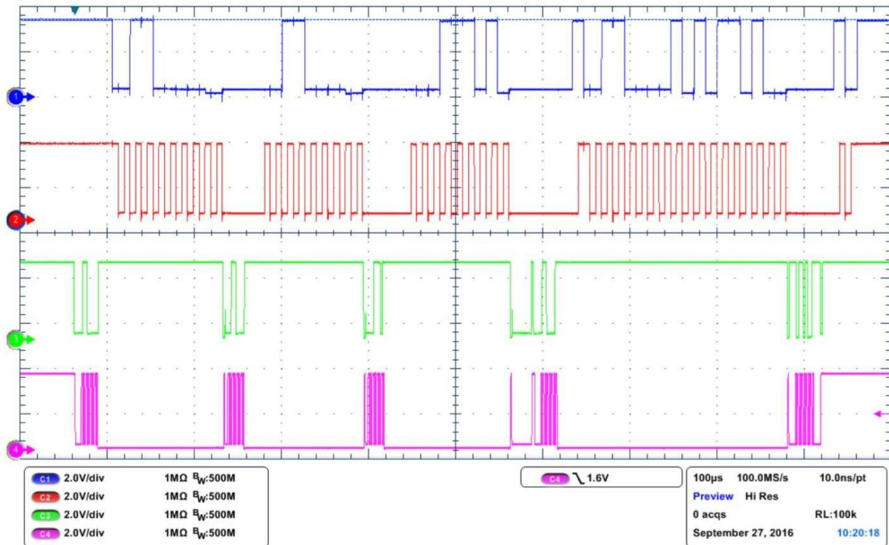
**Figure 13. I<sup>2</sup>C Communication Waveforms**
