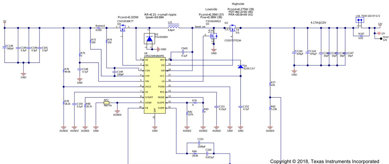
Figure 9. LM5121 Boost Converter Stage
