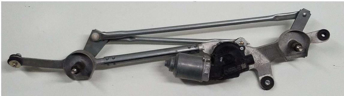
**Figure 20. Front Wiper Hardware**
