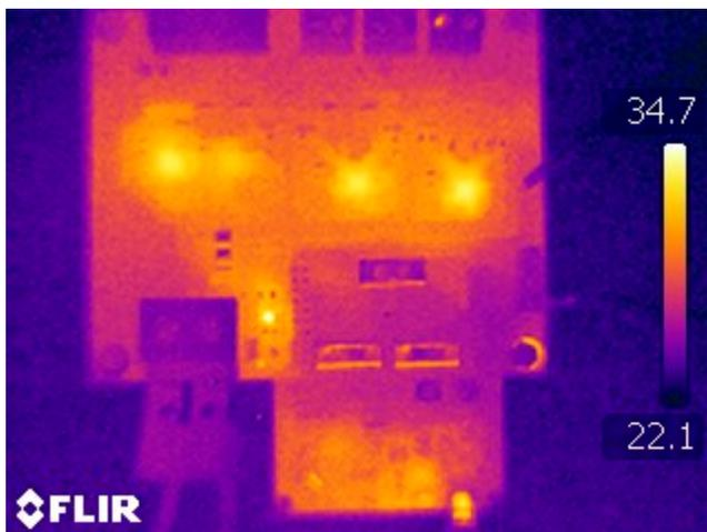
Figure 47. Infrared Image With Front and Rear Wiper Motors Active
