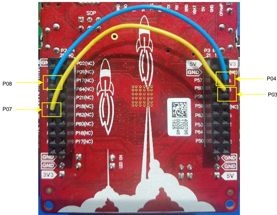
**Figure 15. Jumper Wires Required on CC3220SF-LAUNCHXL**
