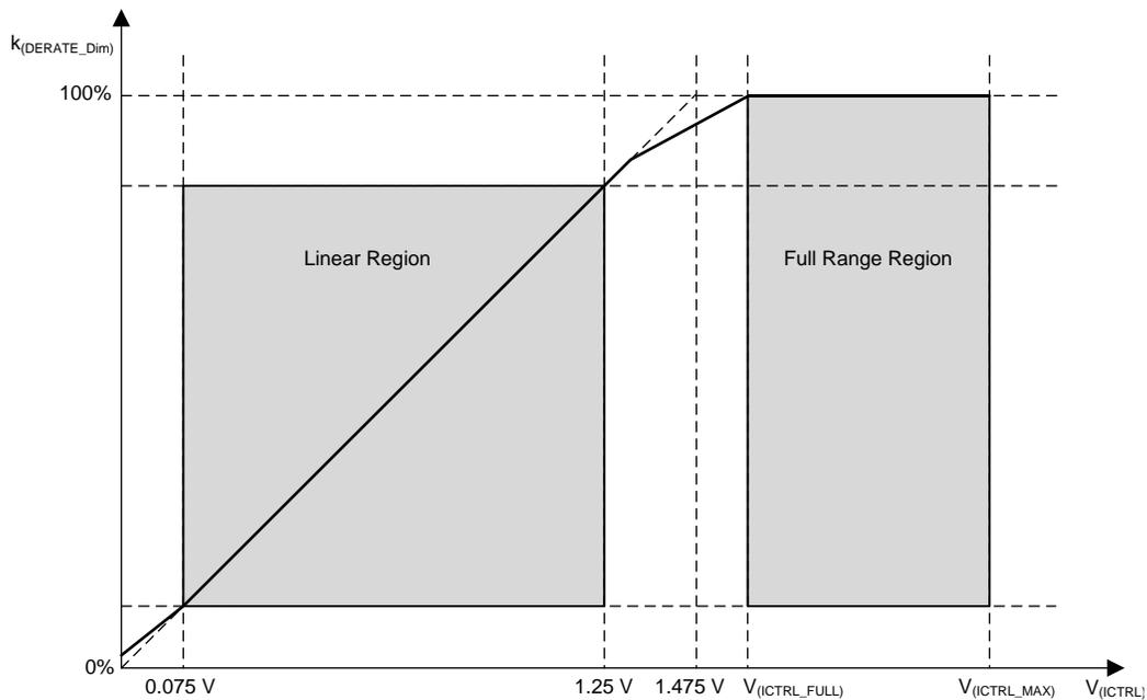
Figure 6. Analog Dimming Ratio
