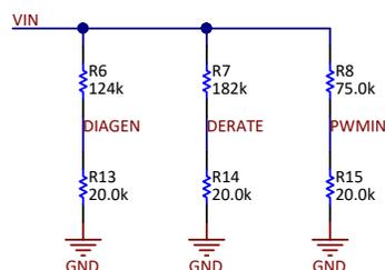
Figure 4. DIAGEN, DERATE and PWM Threshold Setting
