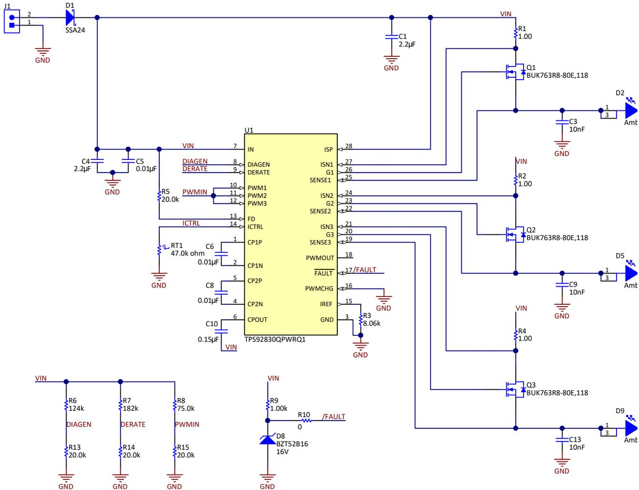
Figure 2. TIDA-01376 Schematic
