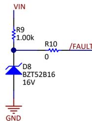
Figure 3. Fault Bus Configuration of TPS92830-Q1
