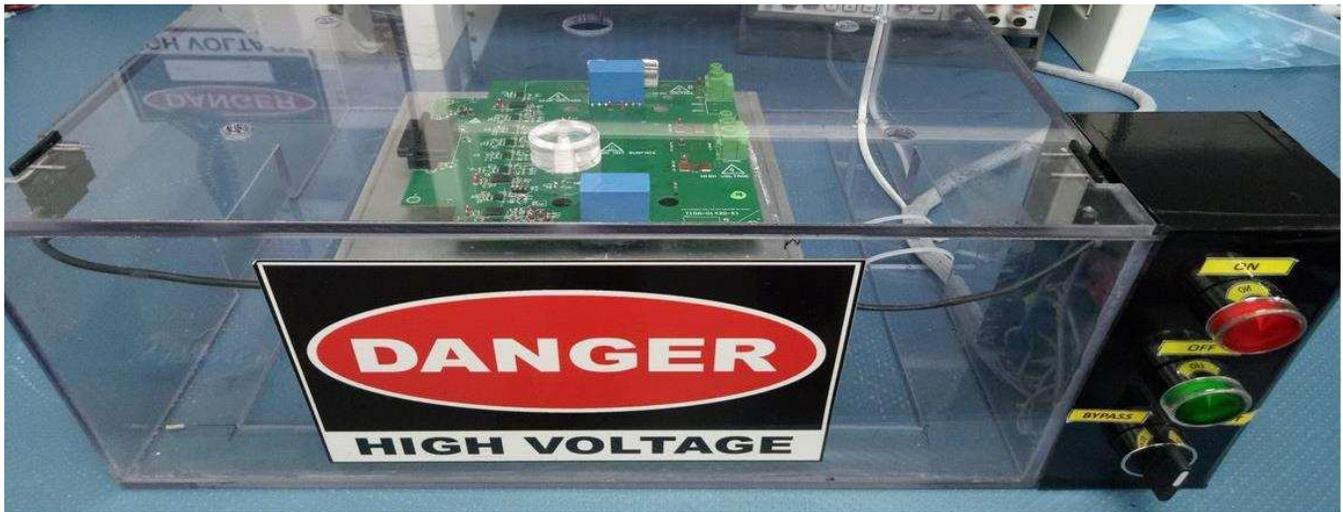
Figure 33. Image of Board Inside High-Voltage Safety Box
