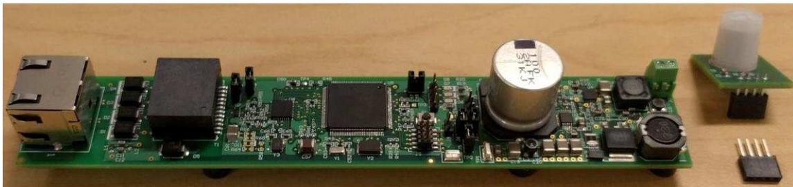
**Figure 9. TIDA-01463 PCB With IR Sensor**
