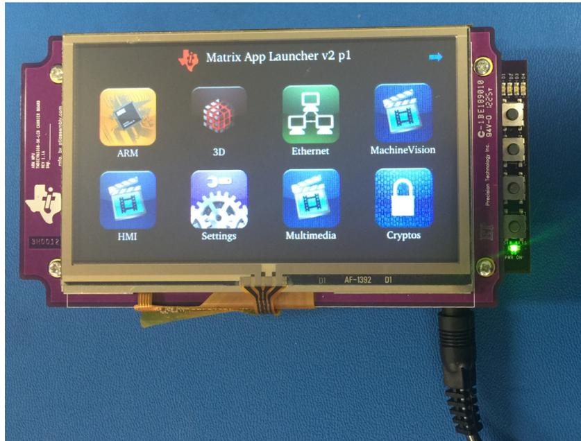
Figure 5. AM335x Starter Kit Setup (LCD Face Up)
