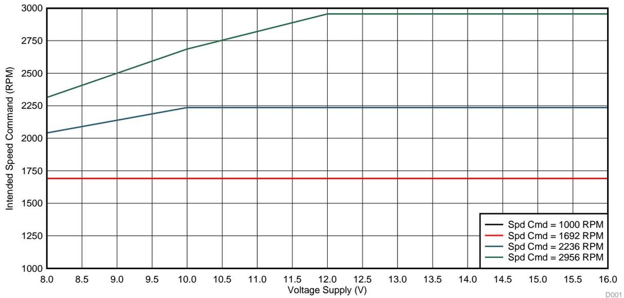
**Figure 22. Speed Regulation: Speed (RPM) versus Voltage Input**
