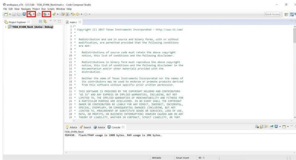
**Figure 7. Building and Debugging Project in CCS**
