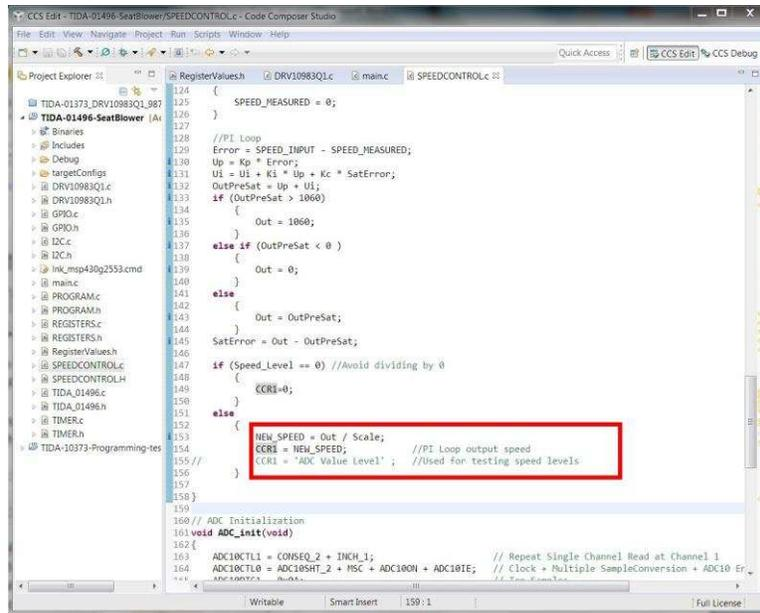
**Figure 13. Example of Changing SPEEDCONTROL.c File for Testing**
