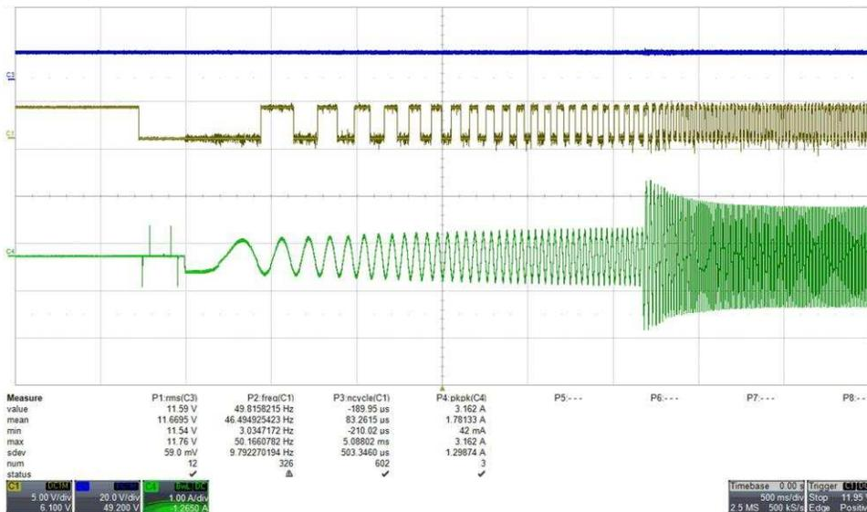
Figure 19. Startup Profile, GUI Control, 12 V, 100% Speed
