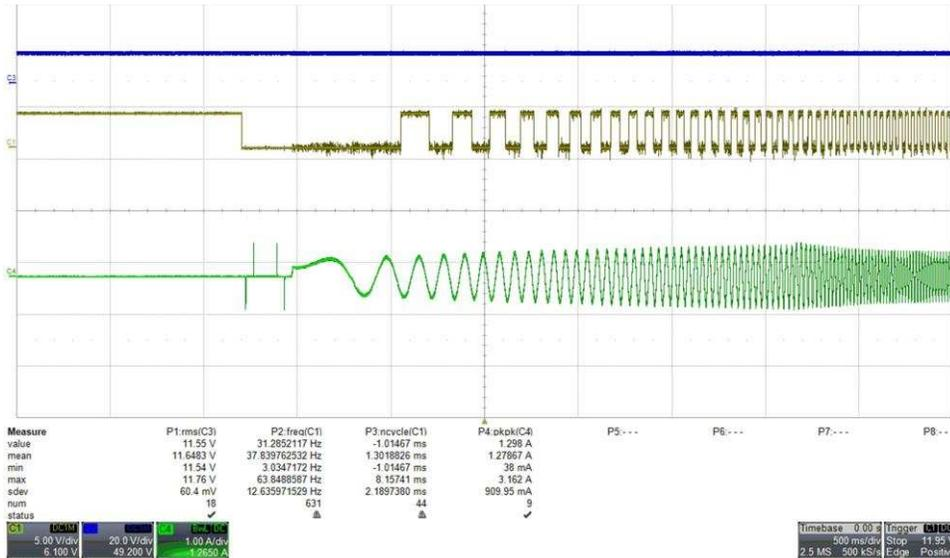
Figure 18. Startup Profile, GUI Control, 12 V, 50% Speed
