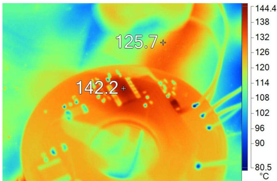
Figure 28. Thermal Image After 15 Hours at 12 W, 125°C Ambient
