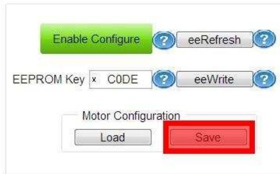
**Figure 8. How to Save a Motor Configuration File in DRV10x GUI**
