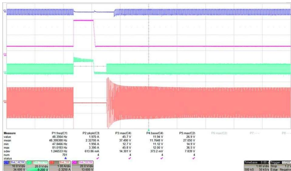
**Figure 23. Load Dump Protection Waveforms After Injecting 45-V Pulses**
