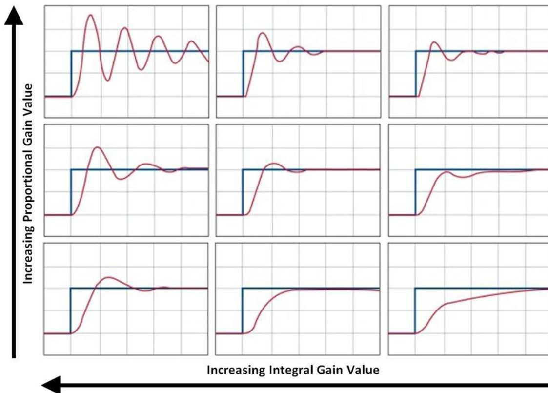
Figure 15. Effects of Tuning PI Controller Gains
