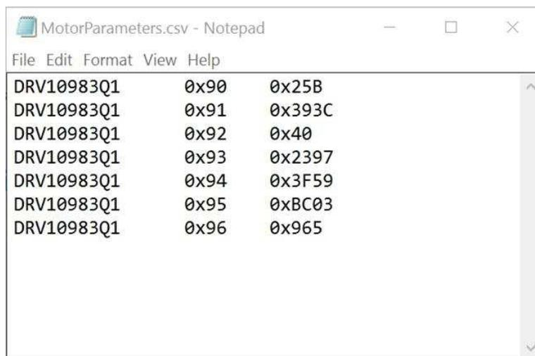
**Figure 9. Example Motor Configuration File in .csv Format**
