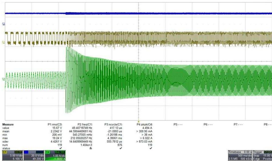
Figure 21. Startup Profile, MSP430 Control, 16 V, 100% Speed
