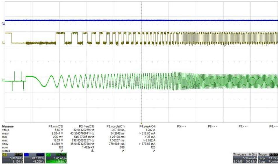
Figure 20. Startup Profile, MSP430 Speed Control, 8 V, 100% Speed
