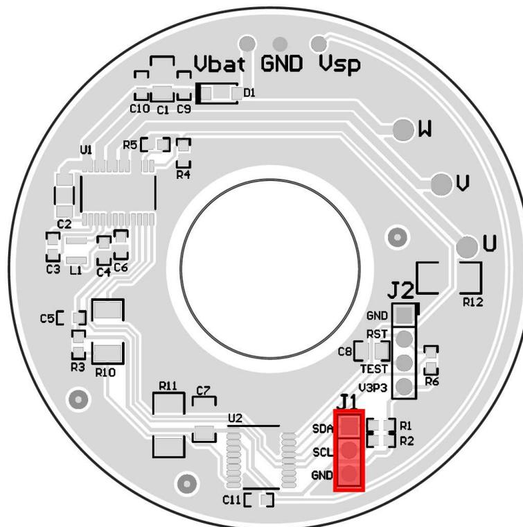
**Figure 4. Hardware Setup for I<sup>2</sup>C Communication**
