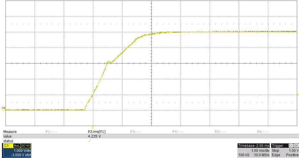
Output voltage startup waveform, 3A load
