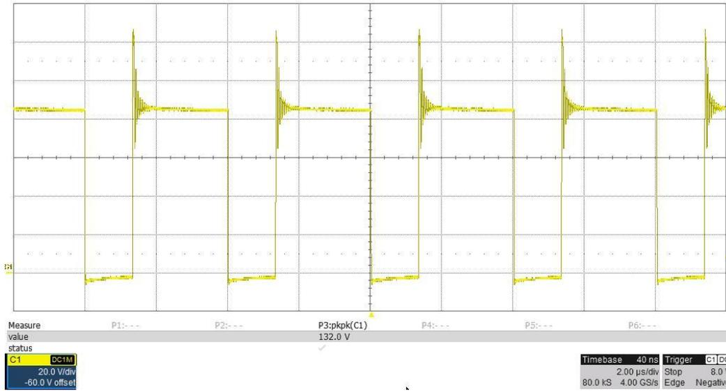
Drain voltage of Q1, 57V input and 3A load.
