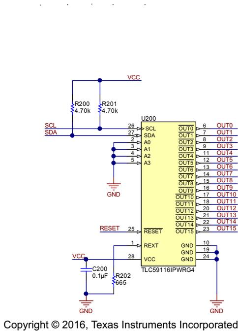
Figure 9. TLC59116-Q1 16-Channel LED Driver With I<sup>2</sup>C Interface
