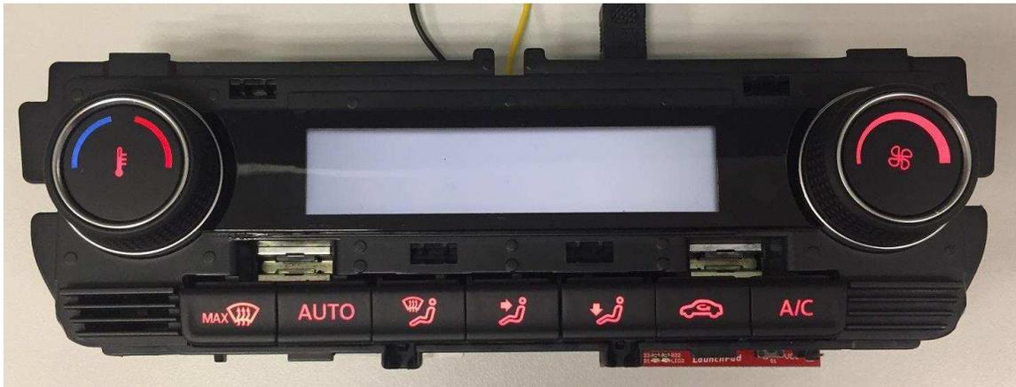
Figure 20. LED Dimming With 45% Duty Cycle
