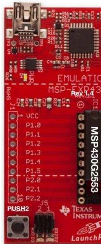
Figure 15. MSP-EXP430G2553 Pinout
