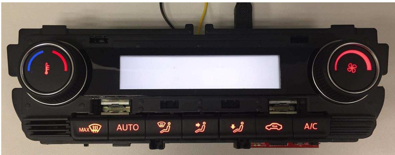
Figure 13. TIDA-01500 into HMI Housing
