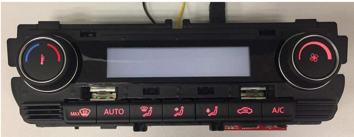
**Figure 19. LED Dimming With 20% Duty Cycle**
