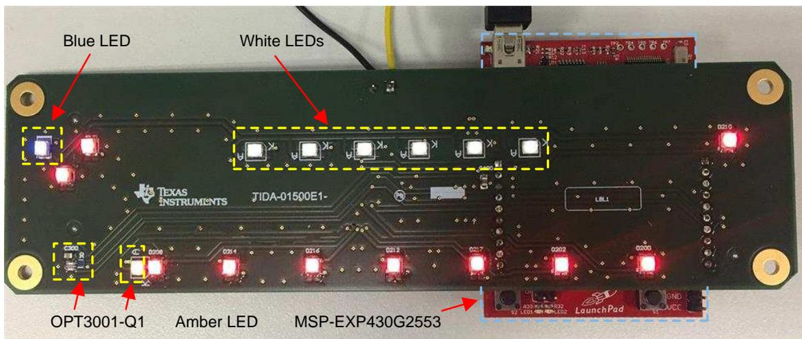
**Figure 5. LaunchPad™ Development Kit With TIDA-01500—Top Side**
