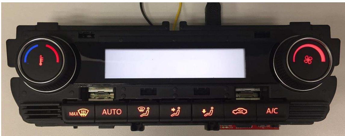
Figure 21. LED Dimming With 80% Duty Cycle
