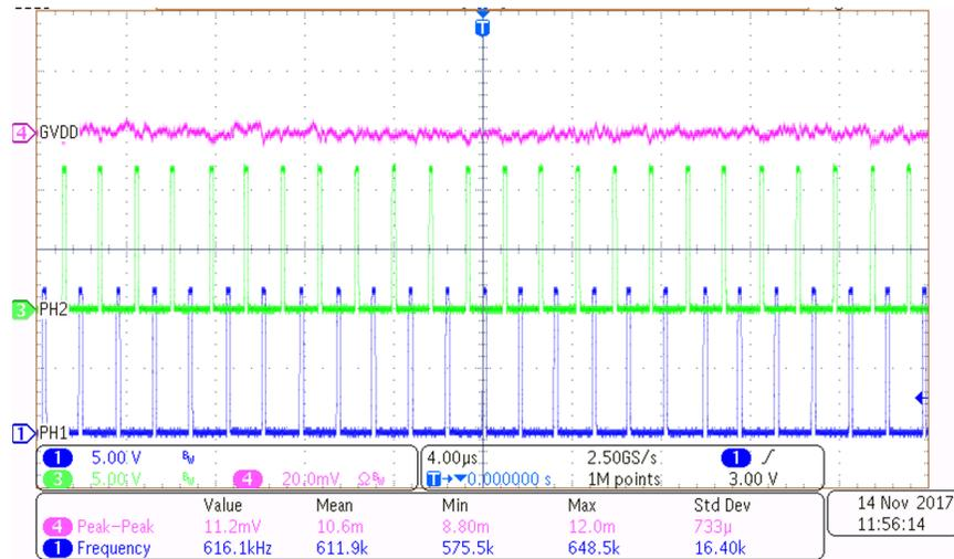
Figure 11. GVDD Rail—Steady State, 30 A
