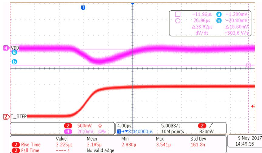
Figure 14. VDD Rail—60-A to 120-A Transient Undershoot, 10% Duty Cycle
