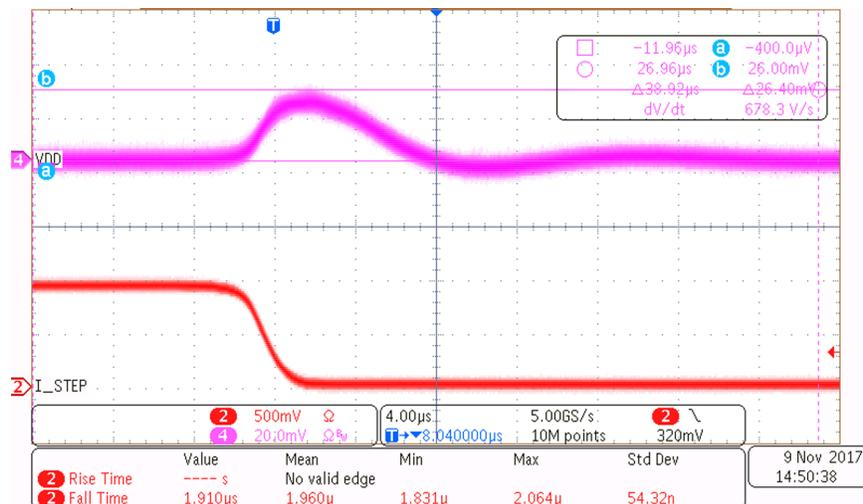
Figure 15. VDD Rail—60-A to 120-A Transient Overshoot, 10% Duty Cycle
