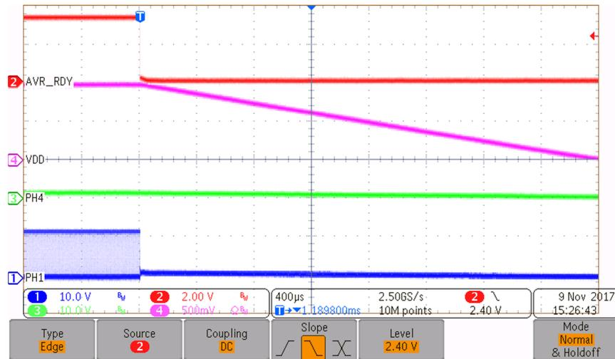
Figure 29. VDD Rail—10-A Shutdown
