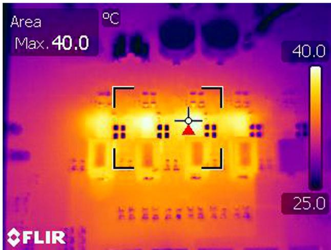
Figure 24. VDD Rail Power Stage Temperatures, 60-A Load
