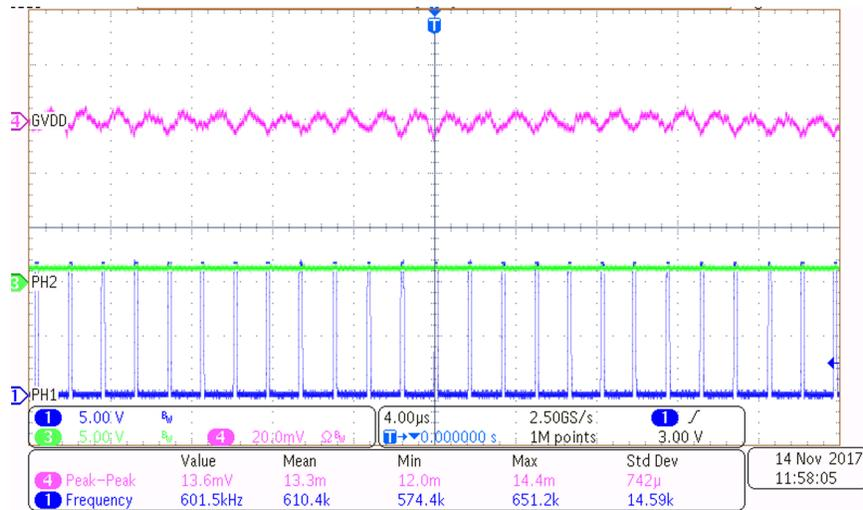
**Figure 10. GVDD Rail—Steady State, 10 A**
