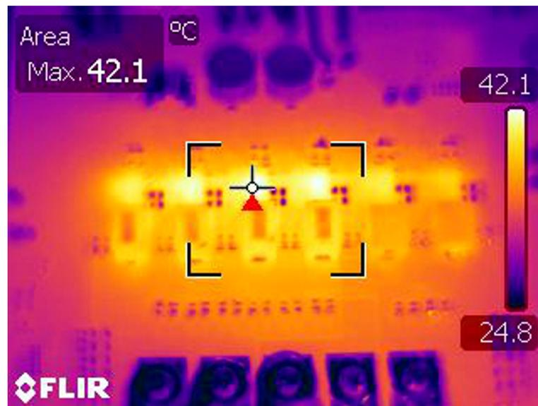
Figure 26. Dual-Rail Power Stage Temperatures
