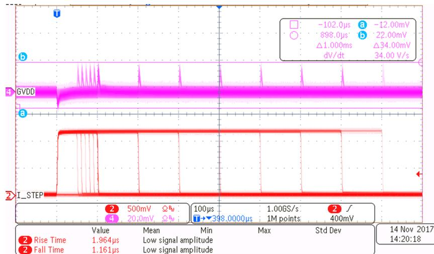
Figure 19. GVDD Rail—10-A to 20-A Transient, 10% to 80% Duty Cycle Sweep
