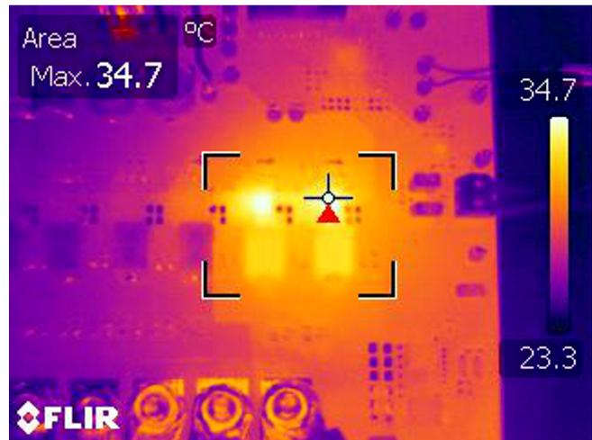
Figure 25. GVDD Rail Power Stage Temperatures, 30-A Load
