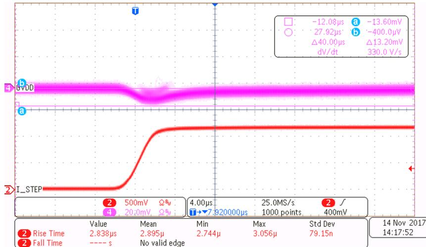
Figure 17. GVDD Rail—30-A to 50-A Transient Undershoot, 10% Duty Cycle
