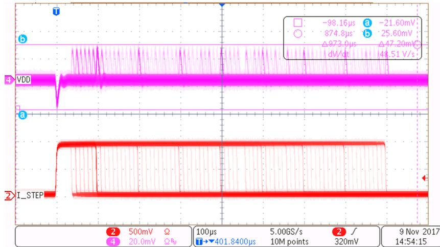
Figure 16. VDD Rail—60-A to 120-A Transient, 10% to 80% Duty Cycle Sweep
