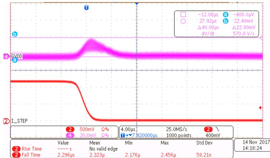
Figure 18. GVDD Rail—30-A to 50-A Transient Overshoot, 10% Duty Cycle
