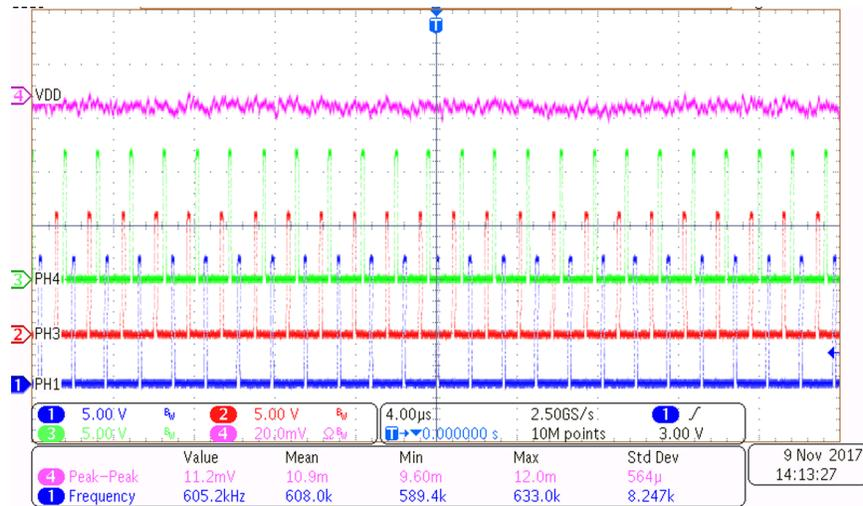
**Figure 9. VDD Rail—Steady State, 120 A**
