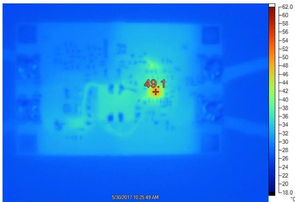
Figure 12. Thermal Image at  $V_{IN} = 36\text{ V}$
