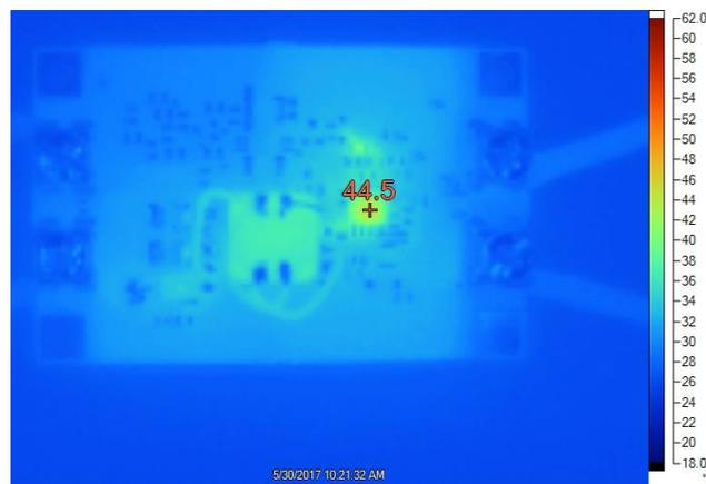
Figure 14. Thermal Image at  $V_{IN} = 24\text{ V}$
