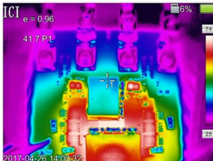
**Figure 37. Thermal Image of Output Inductor (L1)**
