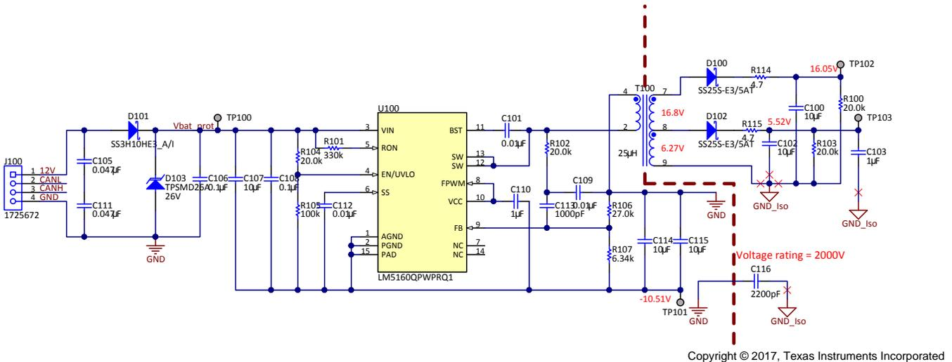
Figure 5. Power supply, Isolated Fly-Buck-Boost Converter
