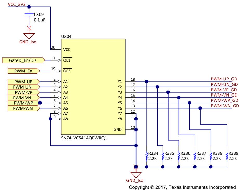
**Figure 15. SN74LVC541-Q1 Octal Buffer With Tri-State Outputs Connected Between MCU and Gate Drivers**
