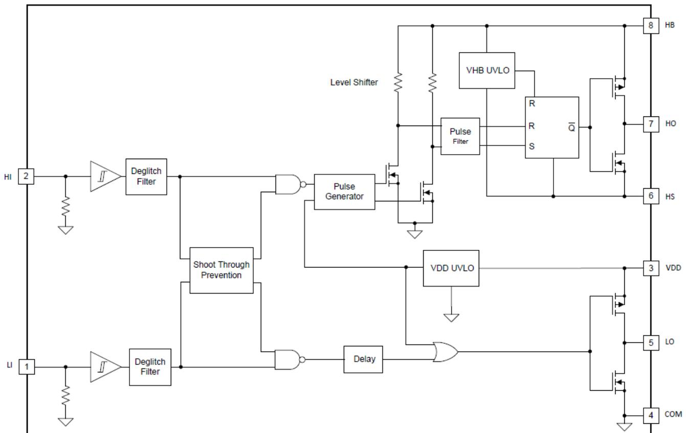
**Figure 10. UCC27712-Q1 Functional Block Diagram**
