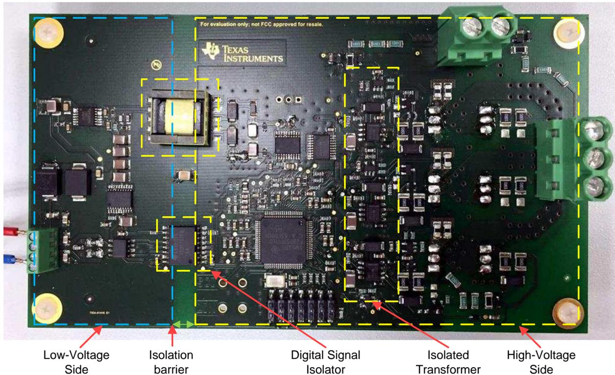
**Figure 3. TIDA-01418 PCB—Top View** <sup>(1)</sup>
