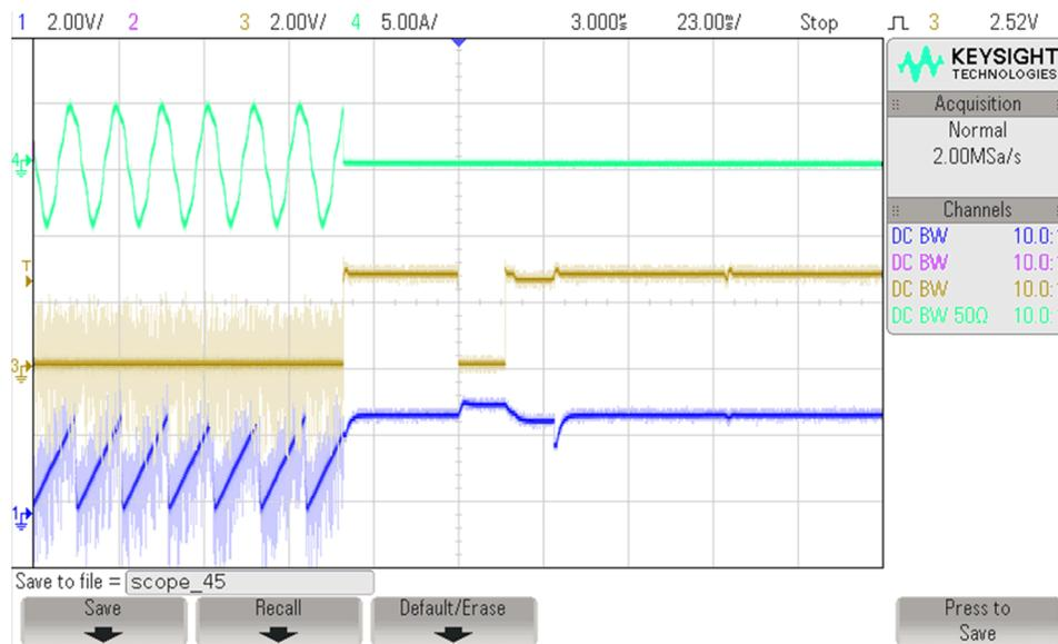
Figure 25. Overcurrent Condition
