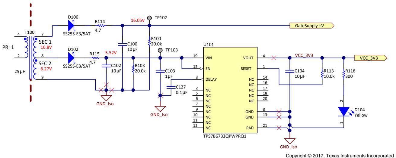
Figure 6. Isolated Transformer With Two Output Voltages on Secondary Side
