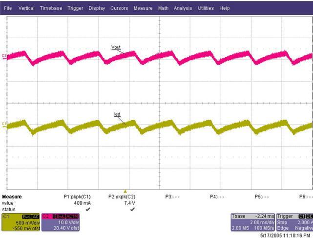
Figure 30. Output Voltage and Current Ripple With 196-W LED Load at 120-V AC
