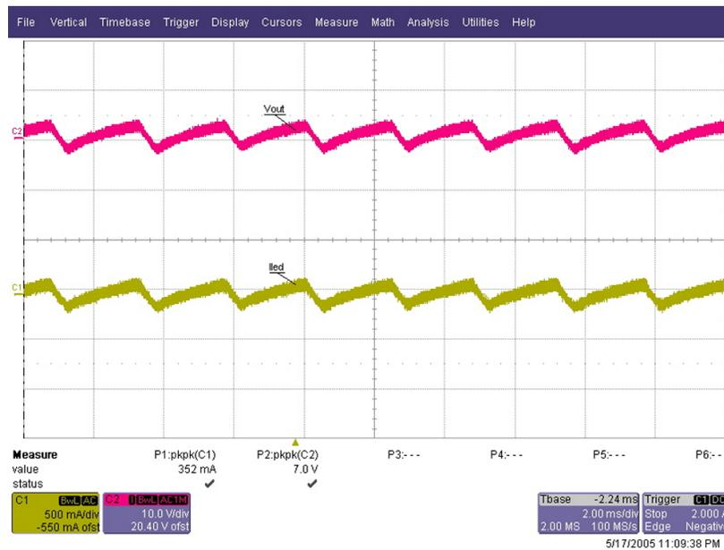
Figure 32. Output Voltage and Current Ripple With 196-W LED Load at 265-V AC
