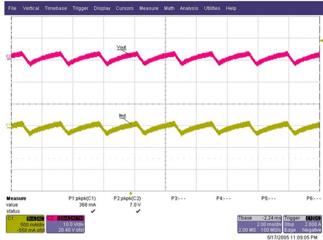
Figure 31. Output Voltage and Current Ripple With 196-W LED Load at 230-V AC
