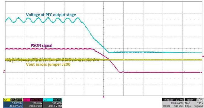
Figure 40. Turnoff at 230-V AC With 196-W LED Load at Output
