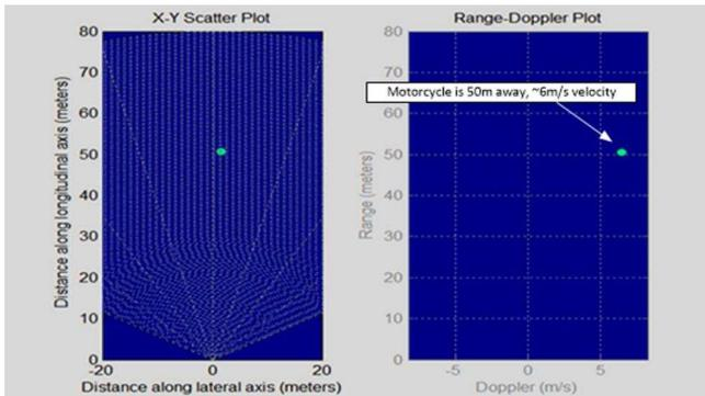
Figure 8. Motorcycle Test at 50 m
