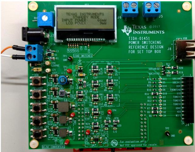
**Figure 8. Full Board 12 V<sub>IN</sub> With LCD ON**
