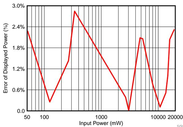
Figure 21. Input Power Accuracy
