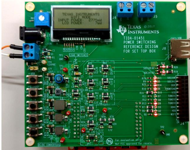
Figure 14. Stream Button LEDs (WIFI, Tuner3, Front End, SOC+DDR)
