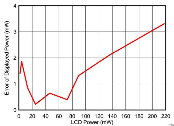
Figure 22. LCD Power Accuracy
