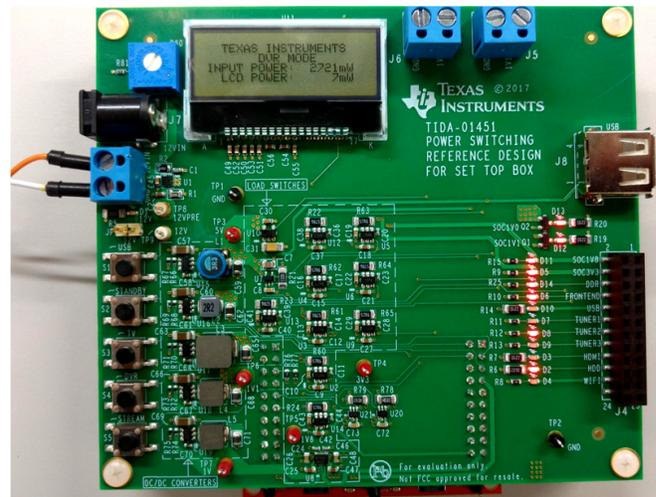
Figure 13. DVR Button LEDs (HDD, Tuner2, Front End, SOC+DDR)
