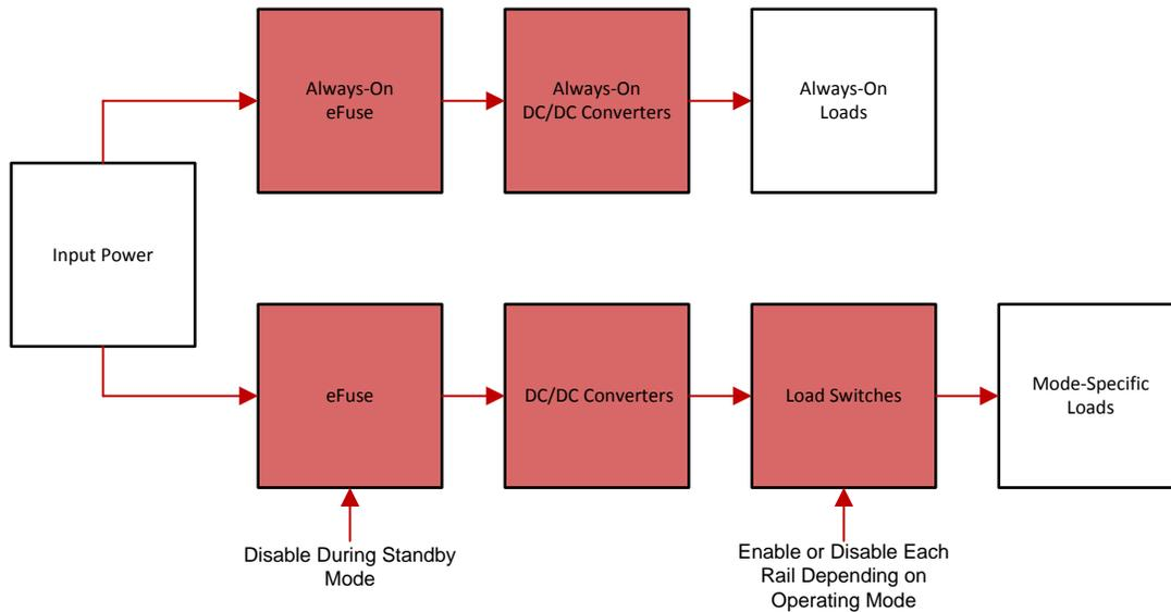
**Figure 4. Separate Always-On Power Tree for Additional Power Savings**
