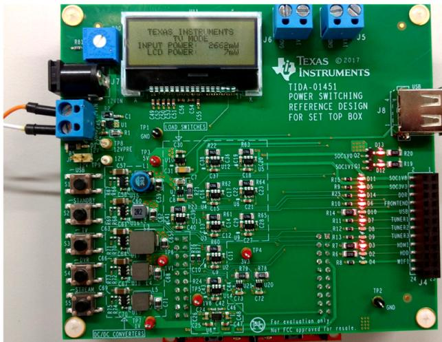
Figure 12. TV Button LEDs (HDMI, Tuner1, Front End, SOC+DDR)
