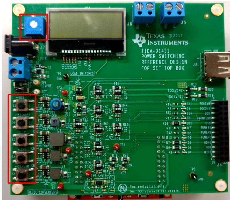
**Figure 7. Board Image With Buttons and Potentiometer Highlighted**
