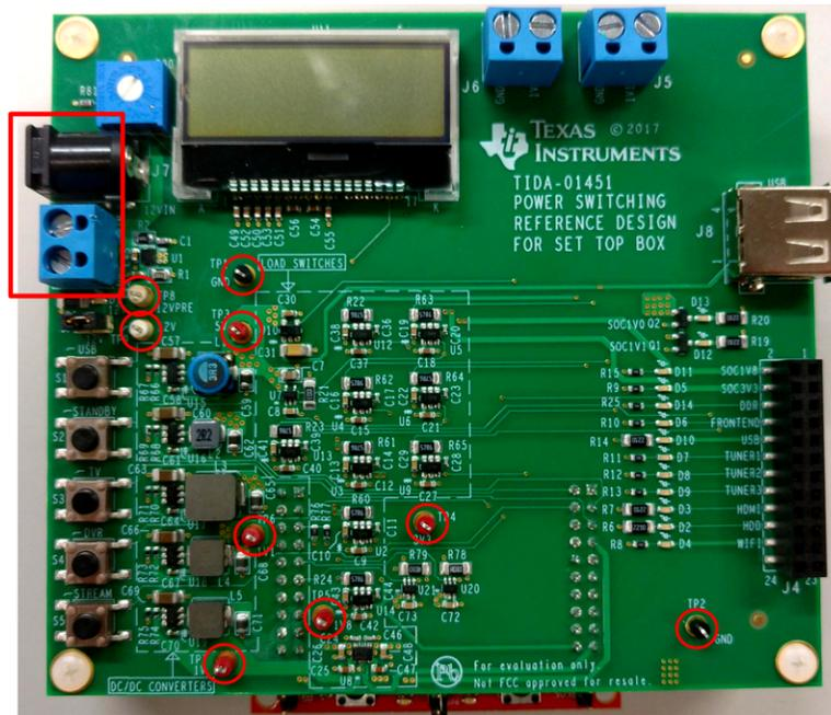
**Figure 6. Board Image With TP Highlighted and Items Relevant to Setup**
