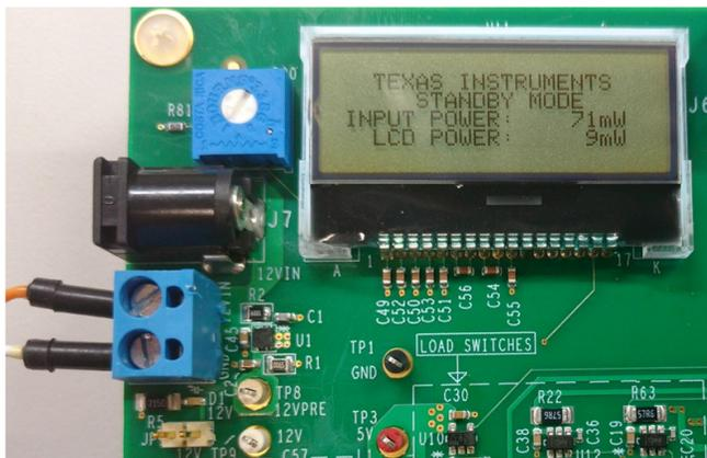
Figure 16. LCD at Lowest Brightness
