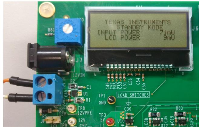
**Figure 9. LCD With Power Measurements**
