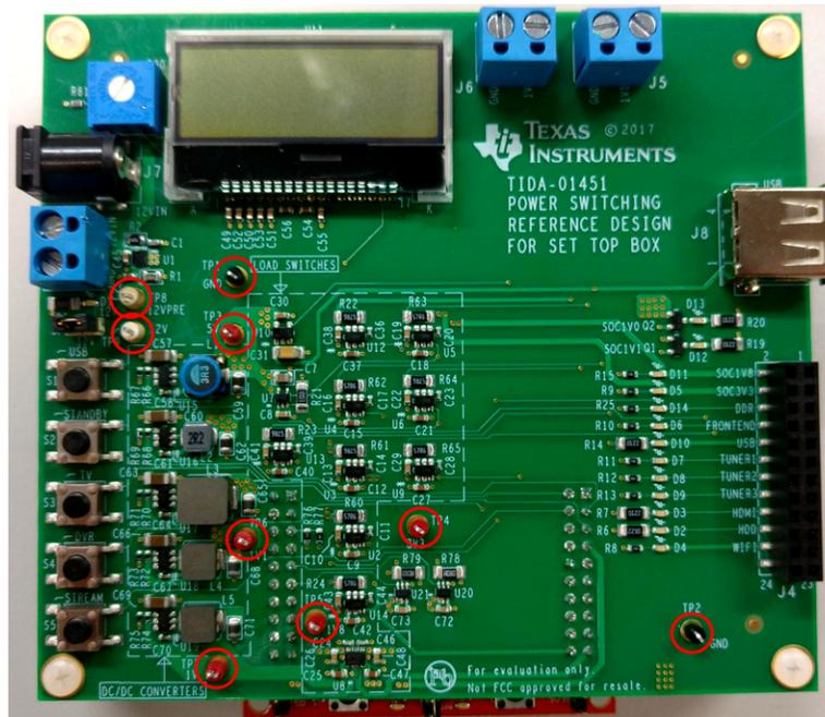
Figure 18. Board Image With Test Points Highlighted
