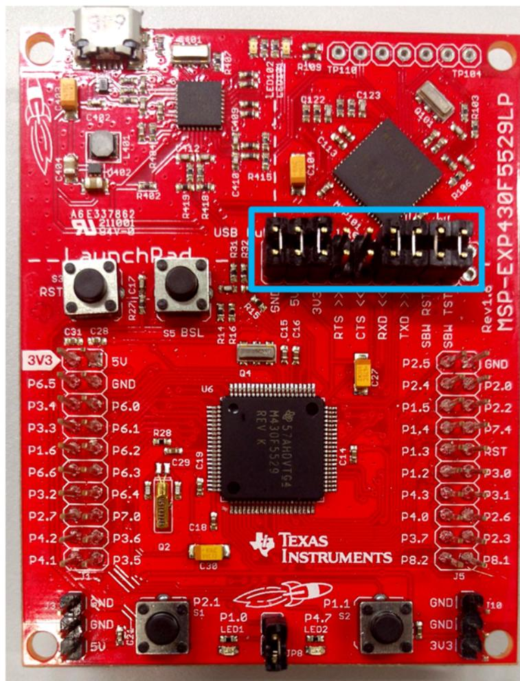
Figure 5. MSP430™ LaunchPad™ Jumpers to Remove
