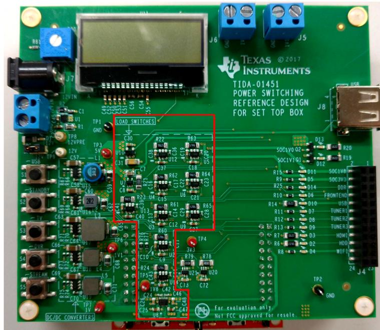
Figure 2. "LOAD SWITCHES" Area
