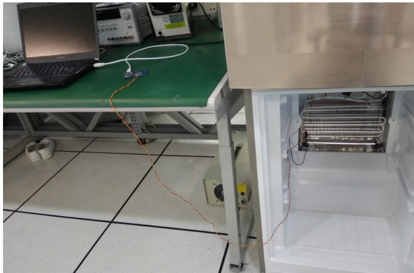
**Figure 35. Long Cable Test Setup**
