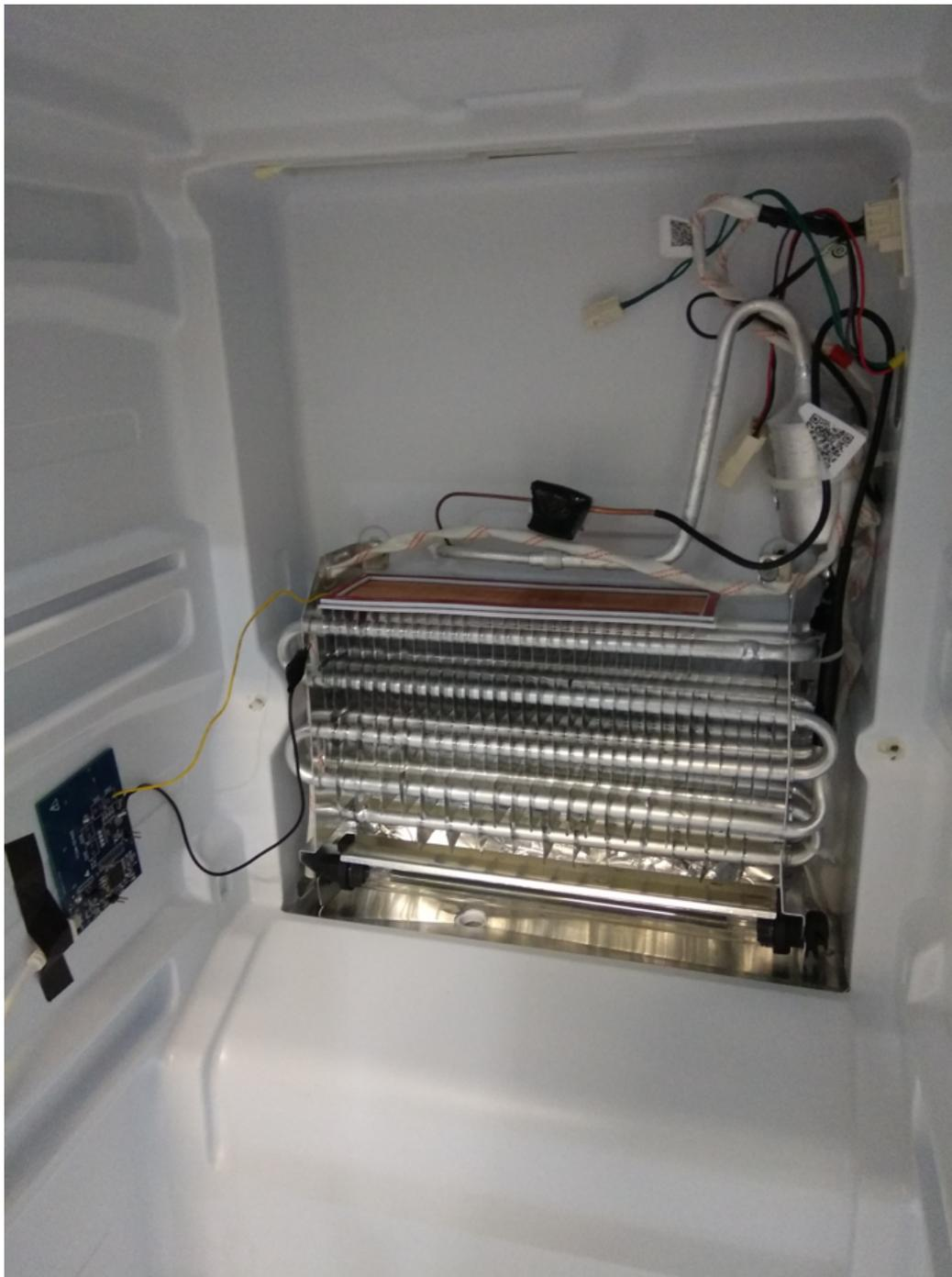
**Figure 23. Evaporator In Refrigerator**
