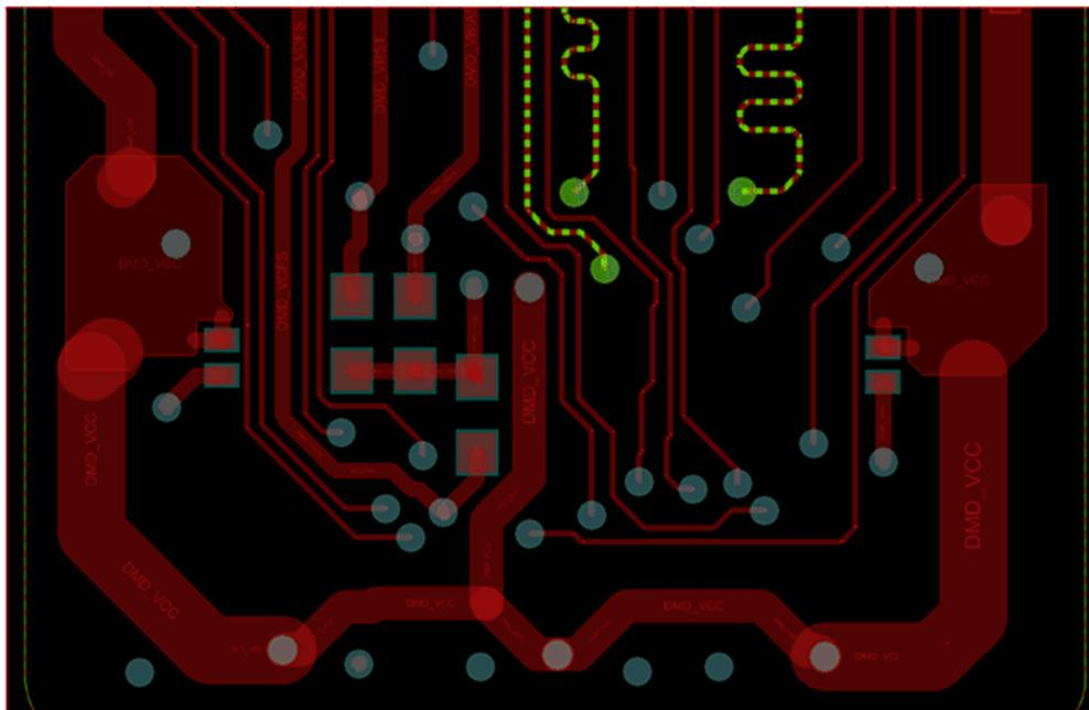
Figure 13. DMD Flex Cable—Bottom Layer
