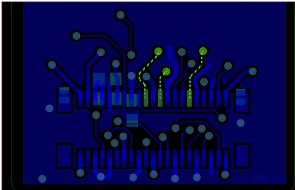
Figure 12. DMD Flex Cable—Top Layer
