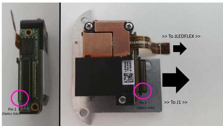
**Figure 3. Overview of Connection for 0.2 nHD Optical Engine**
