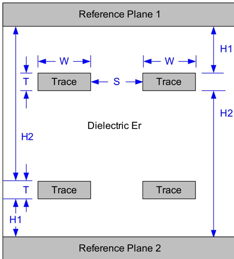
**Figure 11. PCB Stacking Geometries**
