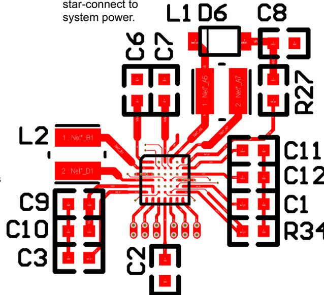
Place C3 (V6V) close to IC and route on top metal. This is low-current trace.
