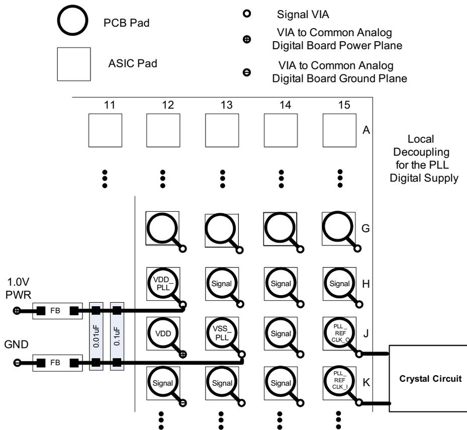
Figure 10. PLL Filter Layout
