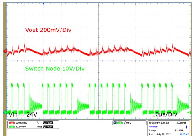
Figure 8. Switch Node, Full Load
