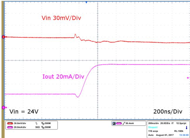
Figure 9. Load Transient, 25 mA to 75 mA
