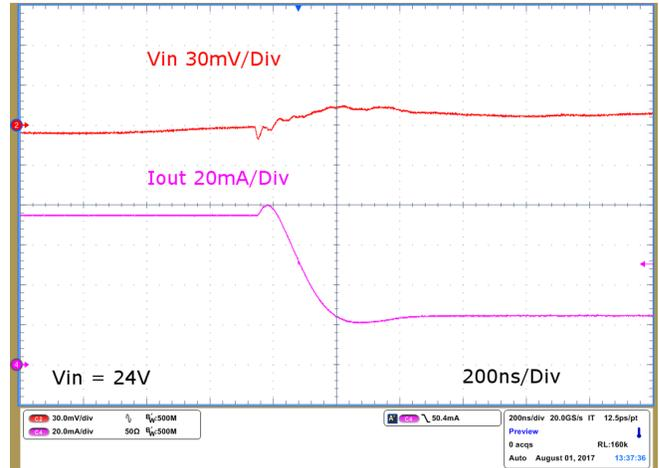
Figure 10. Load Transient, 75 mA to 25 mA
