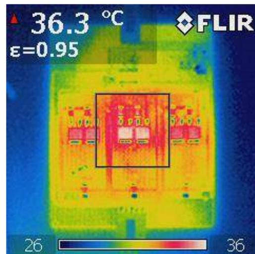
Figure 12. Thermal Image of Position Light Function at 25°C, 12-V Input Voltage
