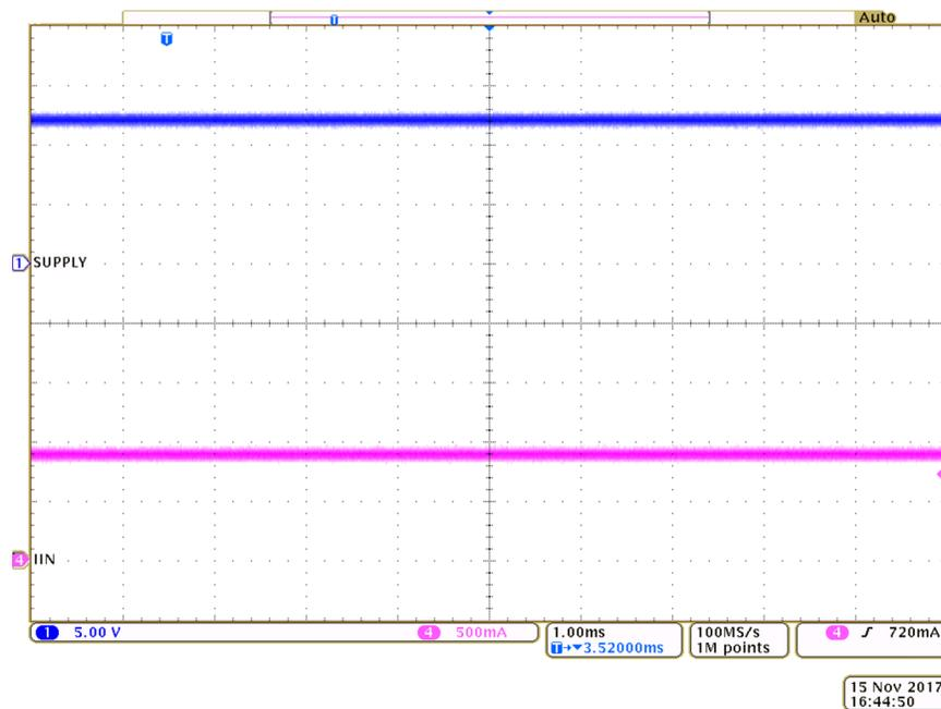
**Figure 9. DRL Function Waveform—CH1: Supply Voltage, CH4: Input Current**
