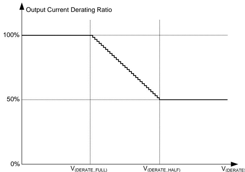
**Figure 5. Output-Current Derating Profile**
