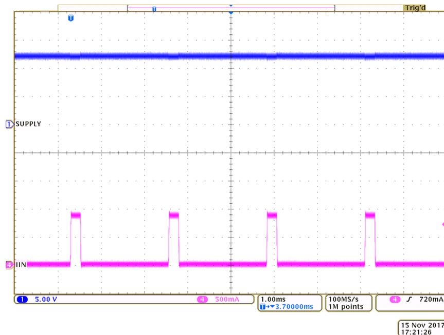
Figure 10. Position Light Function Waveform—CH1: Supply Voltage, CH4: Input Current
