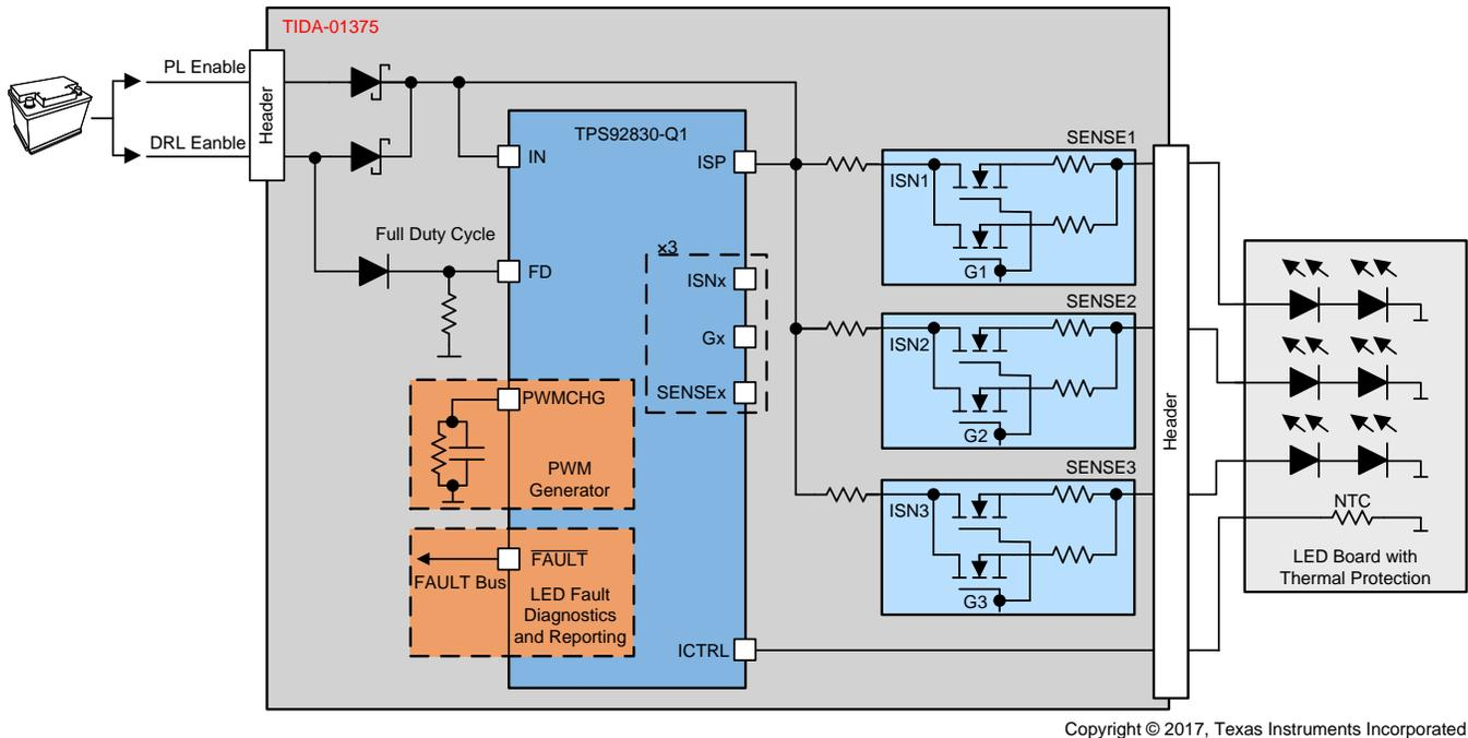
Figure 1. TIDA-01375 Block Diagram
