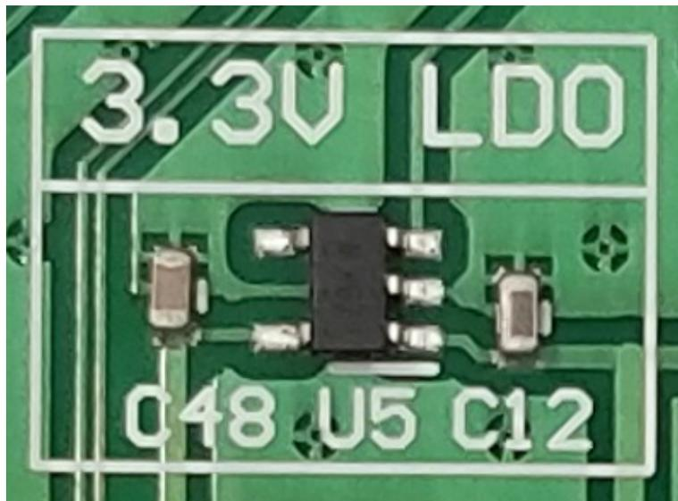
**Figure 17. TLV71333P-Q1 LDO Circuitry on PCB**
