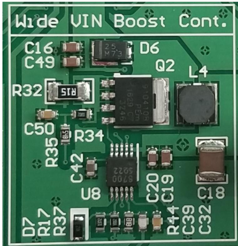
Figure 13. LM5022-Q1 Boost Controller Circuitry on PCB
