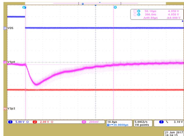
Figure 45. Buck Converter Load Step Increase Response
