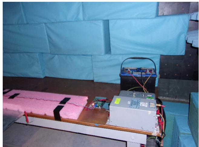
**Figure 52. Master Node Setup for Radiated Emission**
