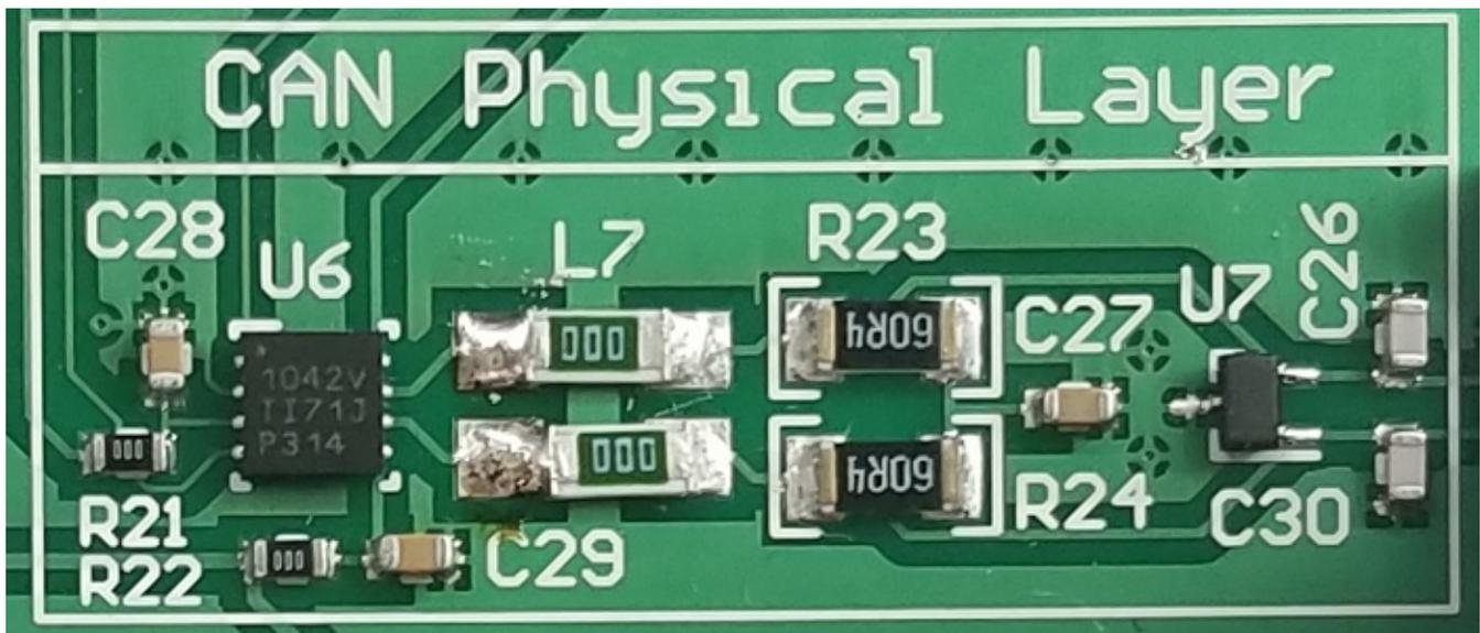
Figure 19. CAN Physical Layer Circuitry on PCB
