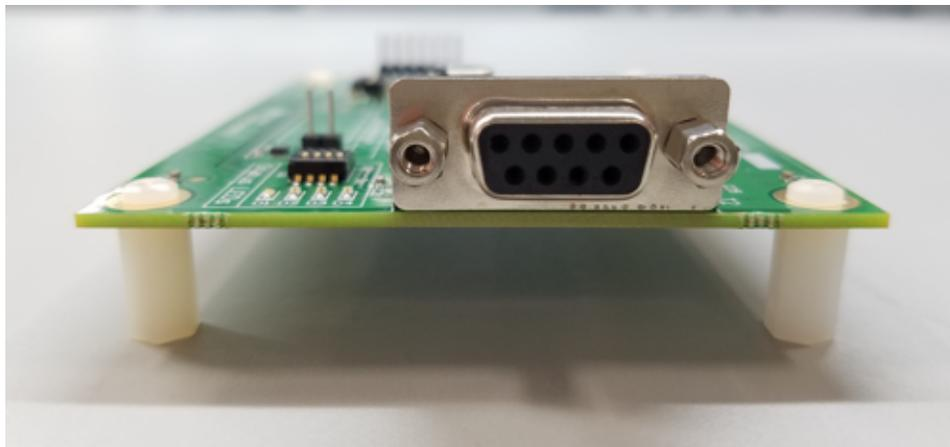
**Figure 21. External Connector for Power and CAN on PCB**
