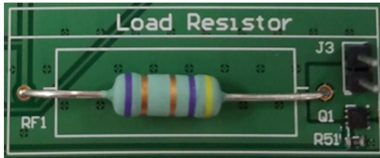
**Figure 23. Dummy Load Resistor Circuitry on PCB**
