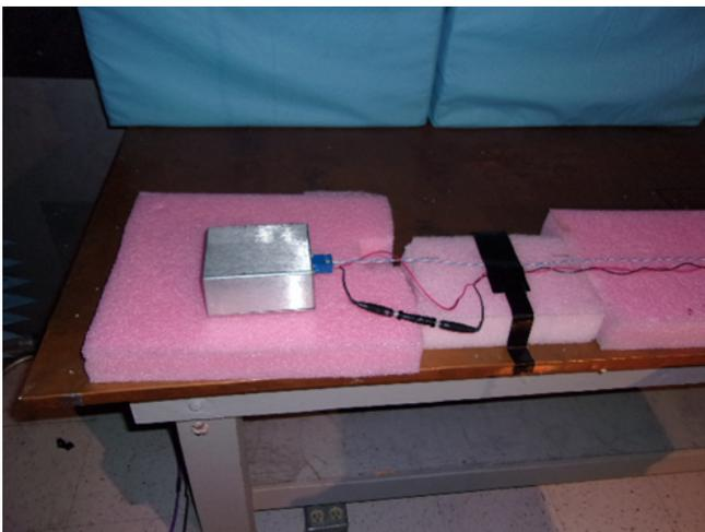
**Figure 51. Slave Node Setup for Radiated Emissions**
