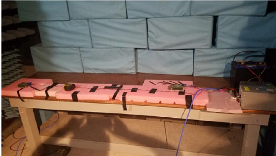
**Figure 49. Conducted Emissions Setup**
