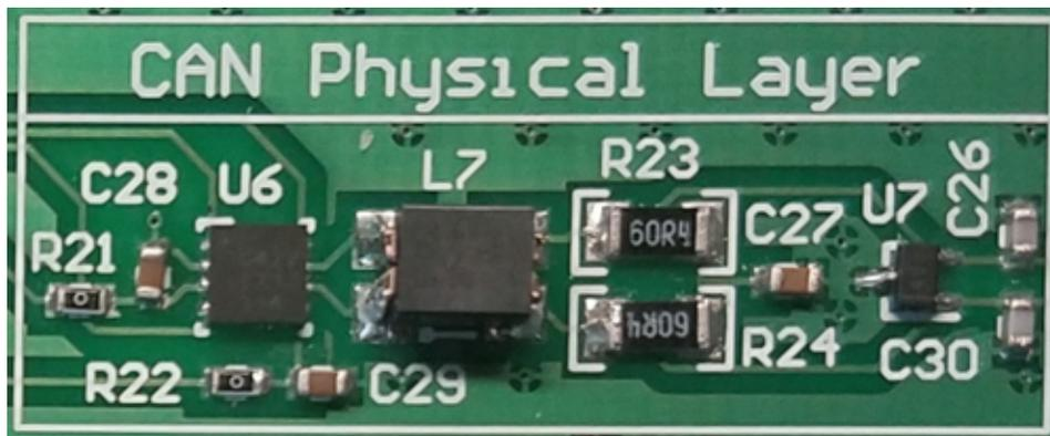
Figure 14. CAN Physical Layer Circuitry on PCB
