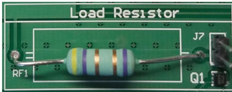
**Figure 18. Dummy Load Resistor Circuitry on PCB**
