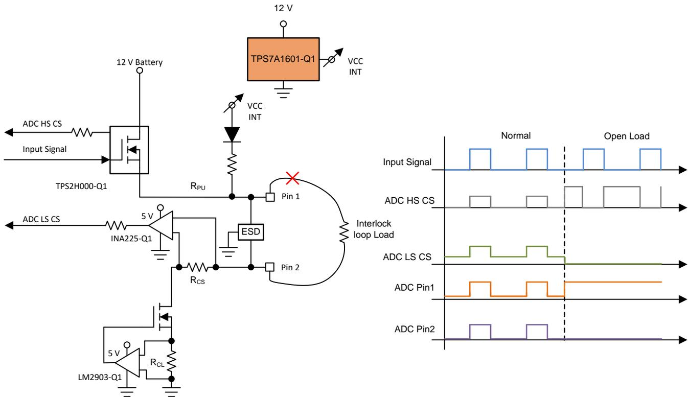
**Figure 12. Interlock Line Open Load**
