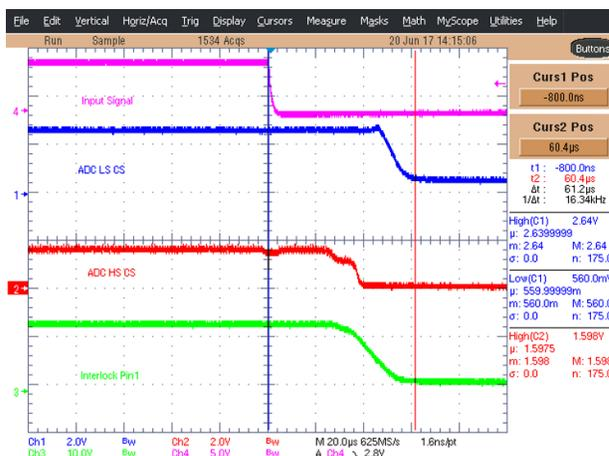
Figure 43. TIDA-01445 Low-Side Current Sense (Fall Time)
