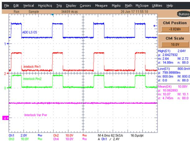
Figure 24. Interlock VCC at 10 V
