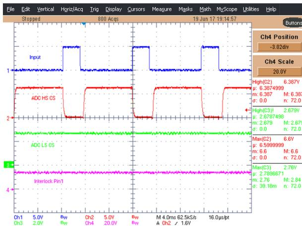
Figure 46. TIDA-01445 Short Circuit to Battery at Pin 1
