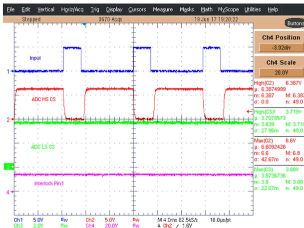
Figure 47. TIDA-01445 Short Circuit to Battery at Pin 2
