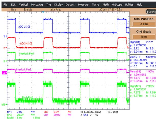
Figure 33. TIDA-01445 at 150-Ω Load Resistance
