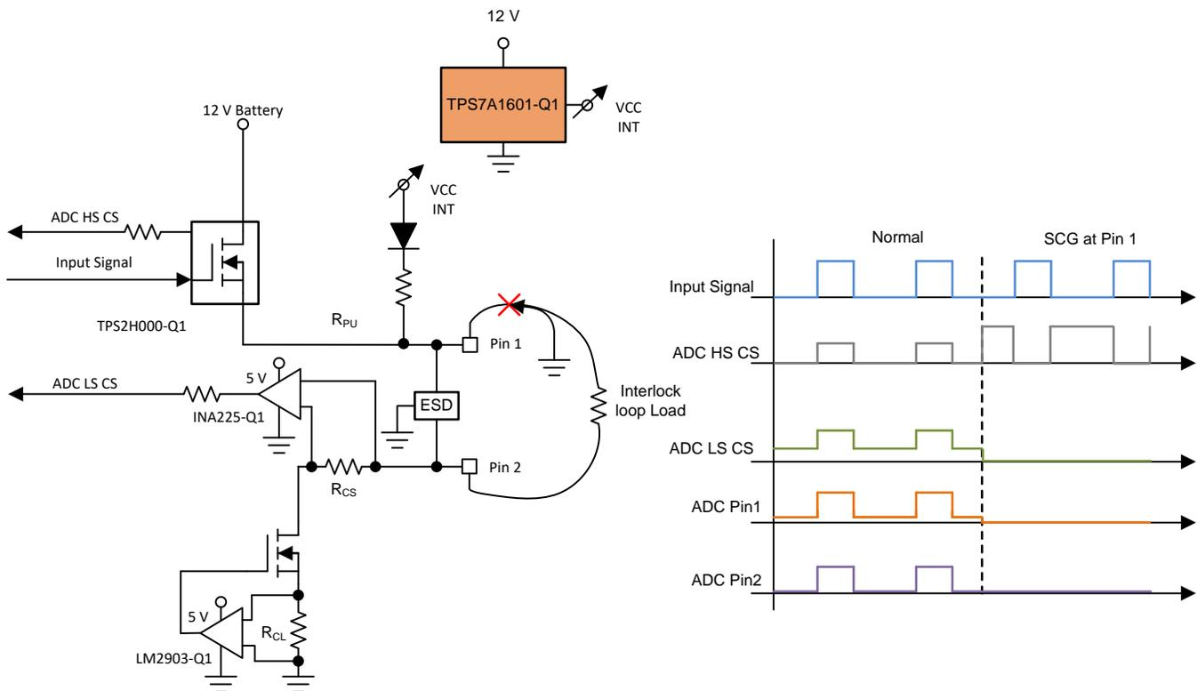
Figure 10. Interlock Line Short Circuit to Ground
