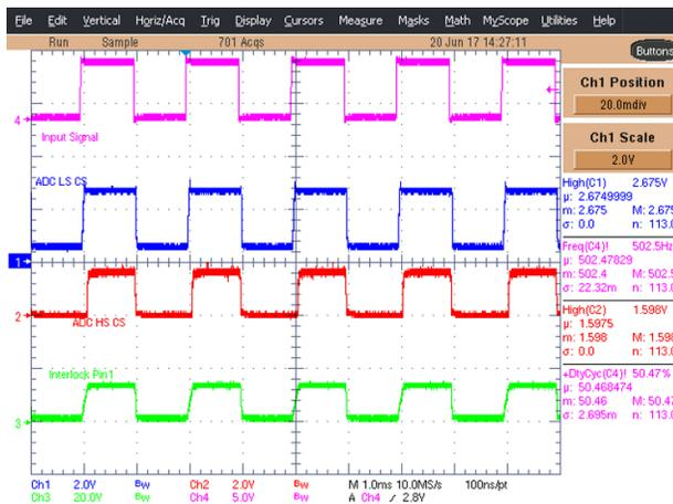
Figure 36. TIDA-01445 for 500 Hz and 50% Duty Cycle
