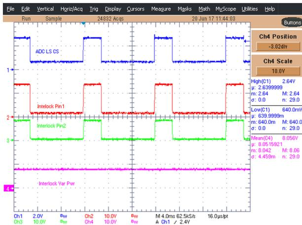
Figure 22. Interlock VCC at 8 V
