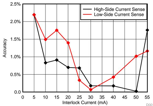
**Figure 18. Accuracy of High-Side and Low-Side Current Sense**
