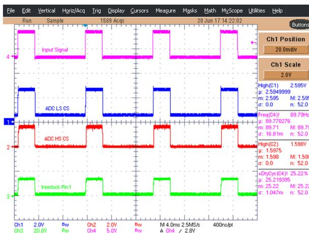
Figure 39. TIDA-01445 for 90 Hz and 25% Duty Cycle
