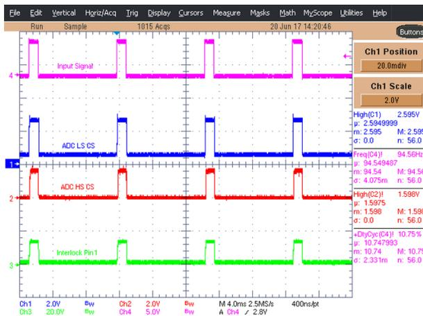
Figure 38. TIDA-01445 for 95 Hz and 10% Duty Cycle
