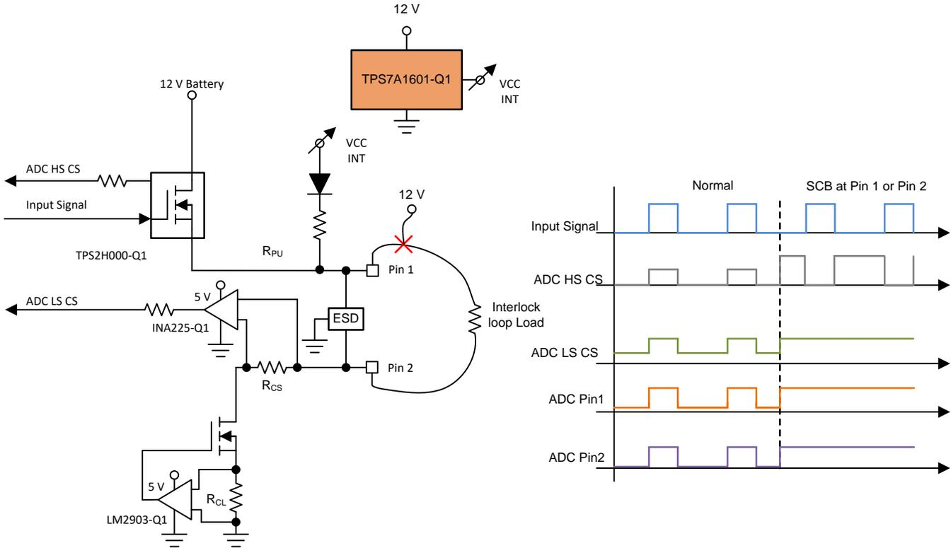
**Figure 11. Interlock Line Short to 12-V Battery**
