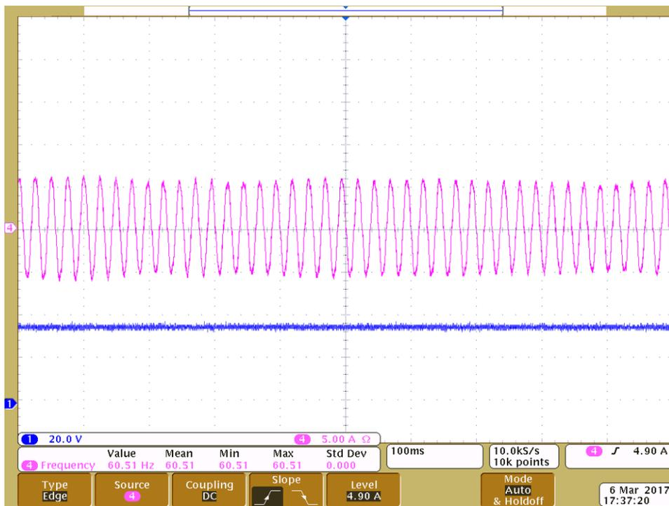
Figure 21. Motor Running at 900 rpm With Light Load
