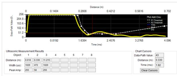
**Figure 45. Detection of Foot at 330 mm Using PUI Transducer**
