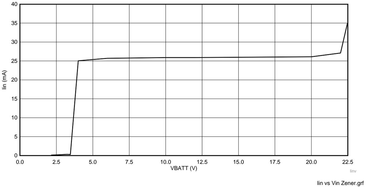
**Figure 18. Input Current Versus Input Voltage, TPS3700-Q1 Overvoltage Threshold at 25 V, TIDA-01424 Board Only**
