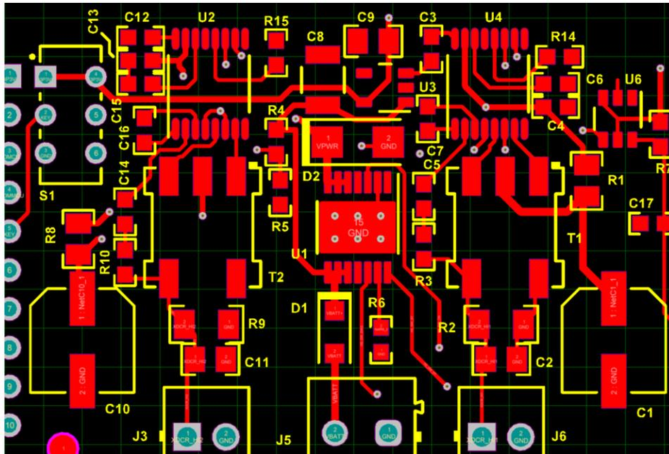
Figure 67. Top Layer Routing of TIDA-01424 Board, With GND Plane Hidden
