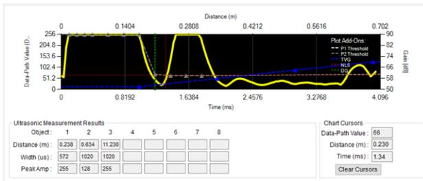
**Figure 41. Sports Shoe Detected at 238 mm**
