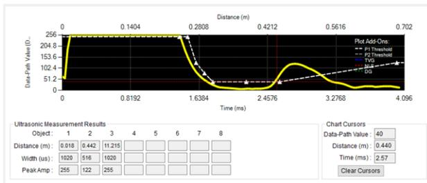
**Figure 43. Detection of Ground at 442 mm Using PUI Transducer**
