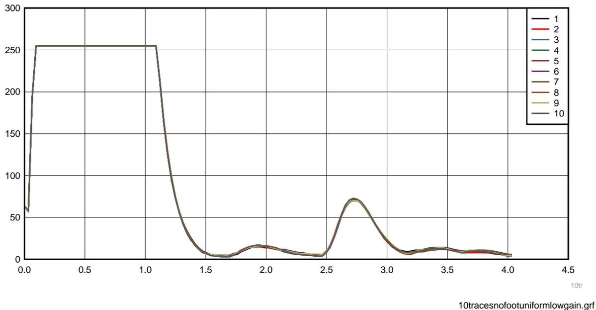
**Figure 26. Ten Sequential Traces With No Foot, Uniform Low TVG Setting**
