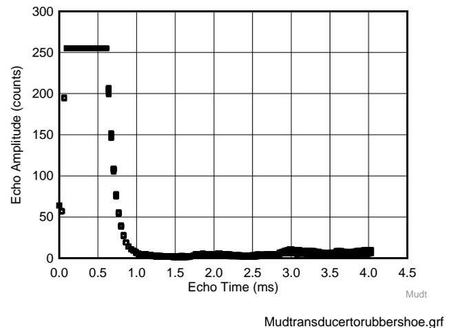
**Figure 60. Response With Normal Transducer to Rubber Shoe**
