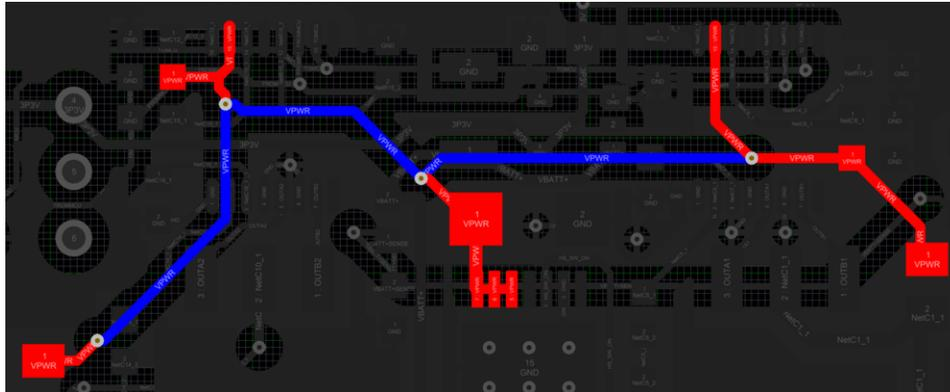
Figure 69. Routing of VPWR Routing From High-Side Switch to PGA460-Q1 Devices and Transformers
