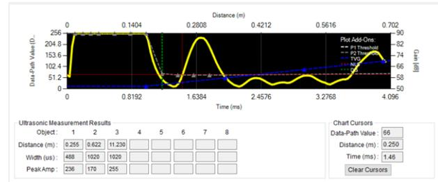
**Figure 40. Sports Shoe Detected at 255 mm**
