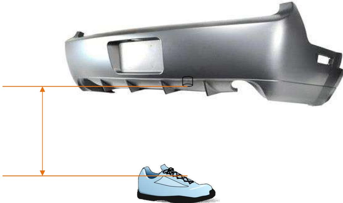
**Figure 27. Vertical Distance Measurement From Ultrasonic Transducer to Shoe**
