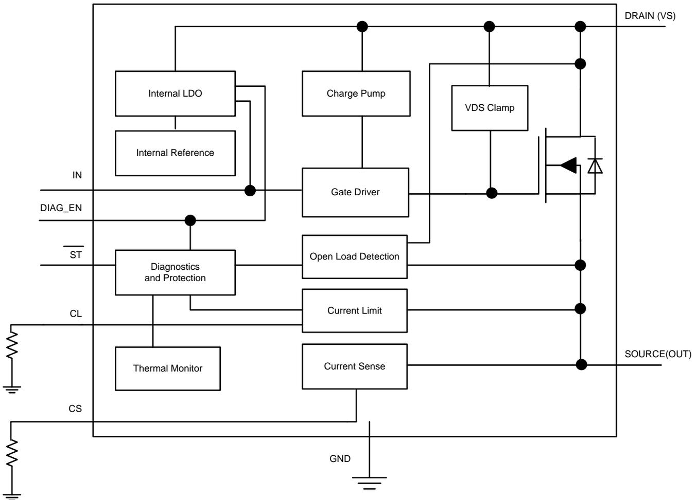
Figure 3. Functional Block Diagram of TPS1H100-Q1
