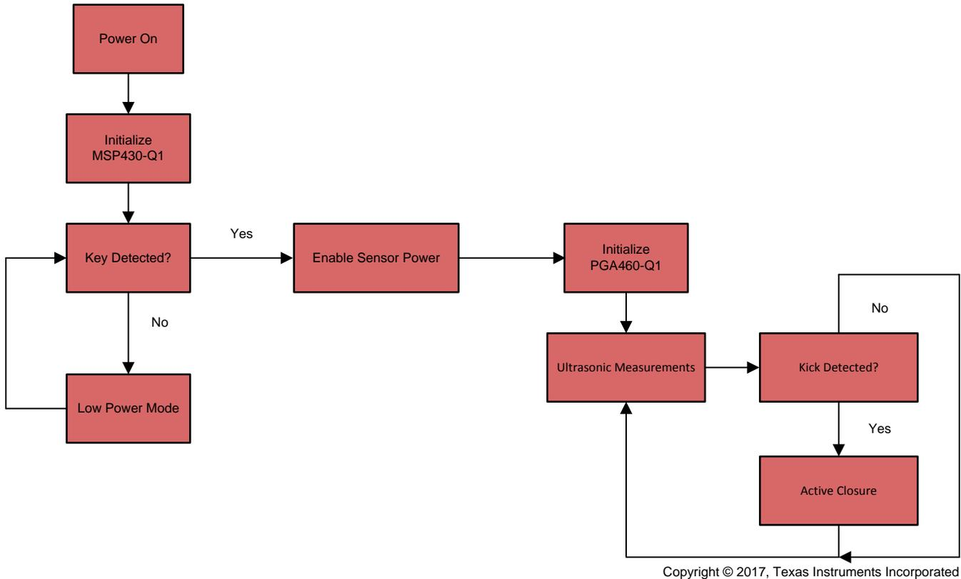
**Figure 14. Simplified Software Flow for Ultrasonic Kick-to-Open Design**
