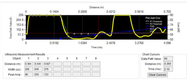
**Figure 35. Sports Shoe Detected at 364 mm**
