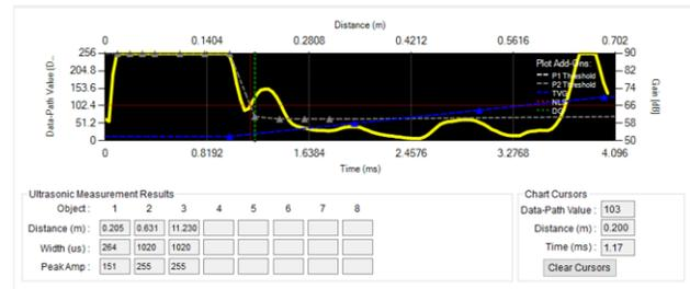
**Figure 42. Sports Shoe Detected at 205 mm**
