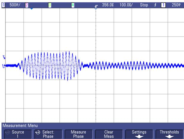
Figure 23. Ultrasonic Acoustic Waveform, R = 2.7 k $\Omega$ , C = 1500 pF
