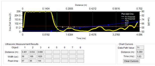
**Figure 39. Sports Shoe Echo Below Threshold at 260 mm, Ground Detected at 461 mm**
