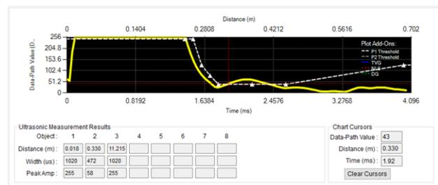
**Figure 48. Foot Not Detected Closer Than 270 mm, Secondary Surface Detected at 330 mm, Using PUI Transducer**
