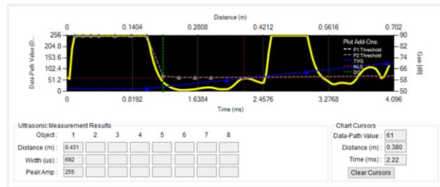
**Figure 34. Sports Shoe Echo Below Threshold, Ground Detected at 431 mm**
