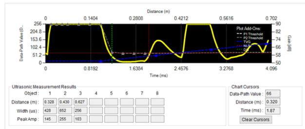
**Figure 36. Sports Shoe Detected at 328 mm**
