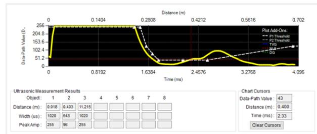
**Figure 44. Detection of Foot at 403 mm Using PUI Transducer**
