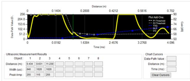
Figure 28. Echo With Rubber Top Shoe, Ground Detection
