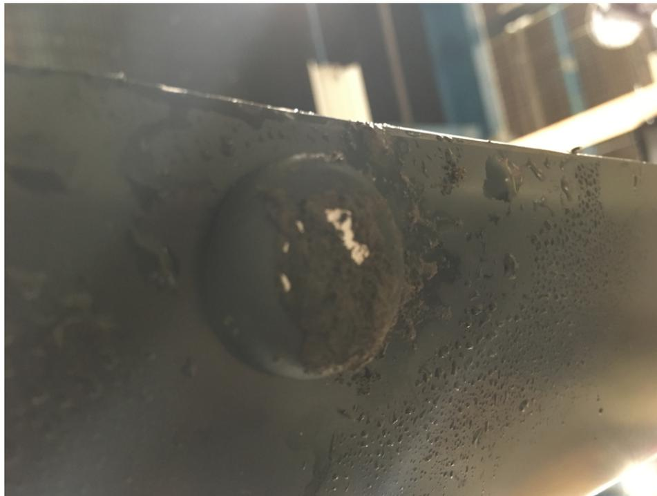
**Figure 59. Mud on Ultrasonic Transducer**
