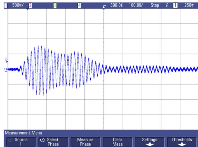
Figure 24. Ultrasonic Acoustic Waveform, R = 10 k $\Omega$ , C = 700 pF
