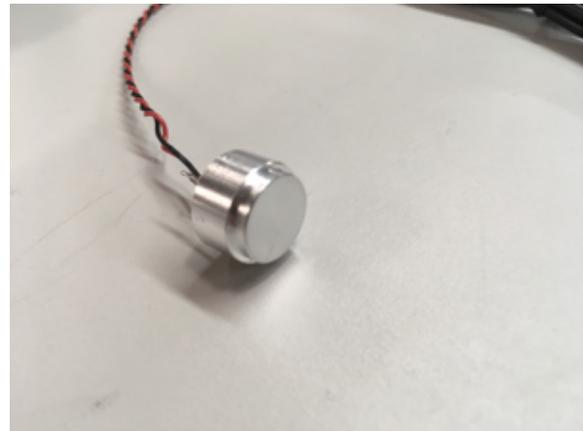
**Figure 12. Closed-Top PUI Ultrasonic Transducer**
