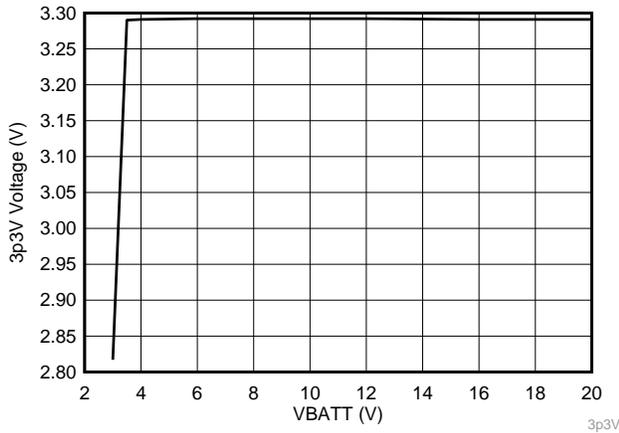
Figure 20. 3.3-V Supply Voltage Versus Input Voltage
