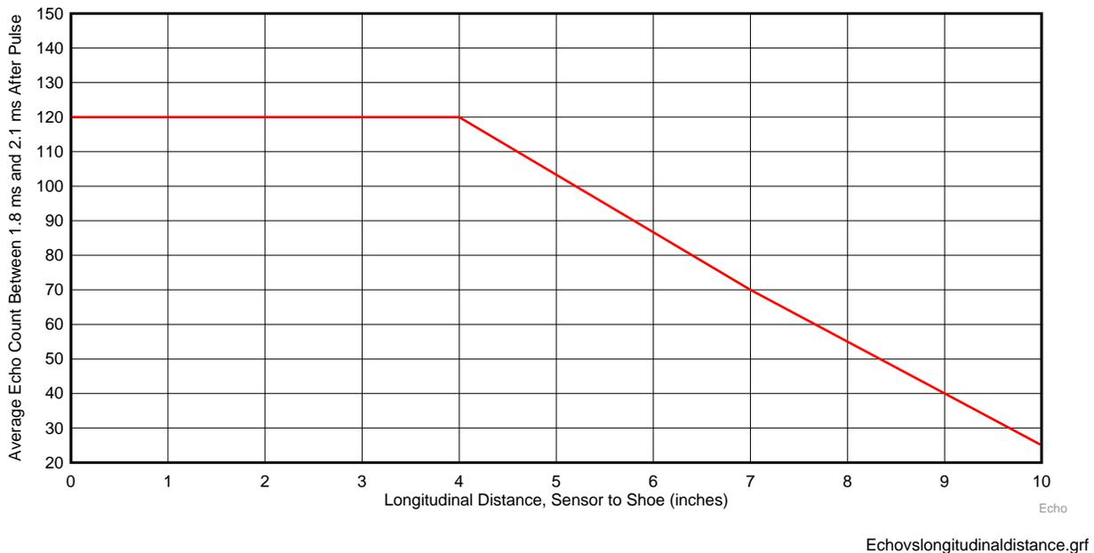
**Figure 53. Effect of Kicking Gesture Directed at Point Displaced From Ultrasonic Transducer**
