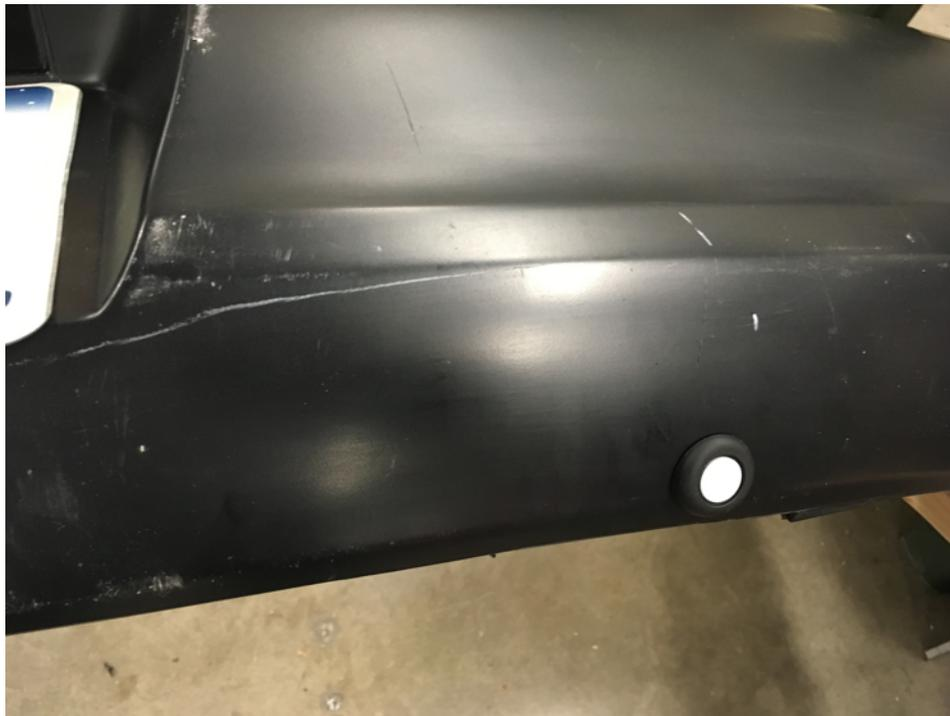
**Figure 15. Bumper Cover With Ultrasonic Sensor**
