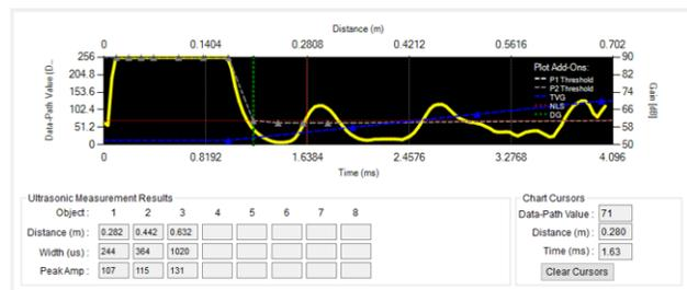
**Figure 38. Sports Shoe Detected at 282 mm**
