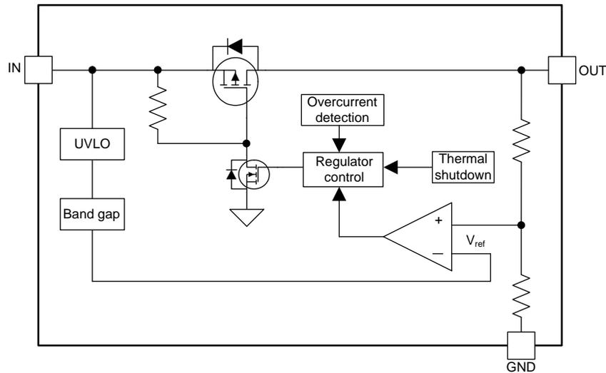
**Figure 4. TPS7B6933-Q1 Functional Block Diagram**
