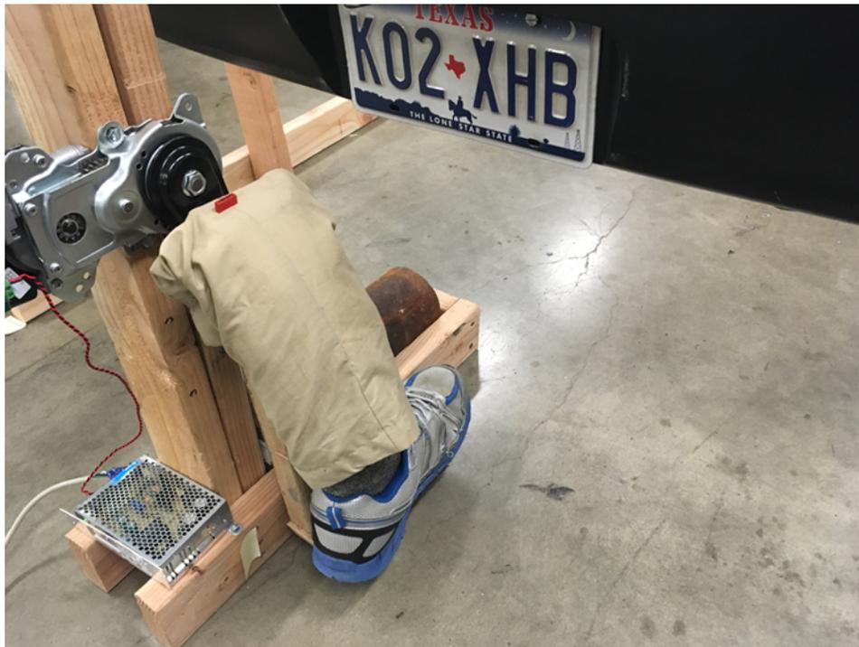
**Figure 16. Kicking Mechanism Used for Testing**
