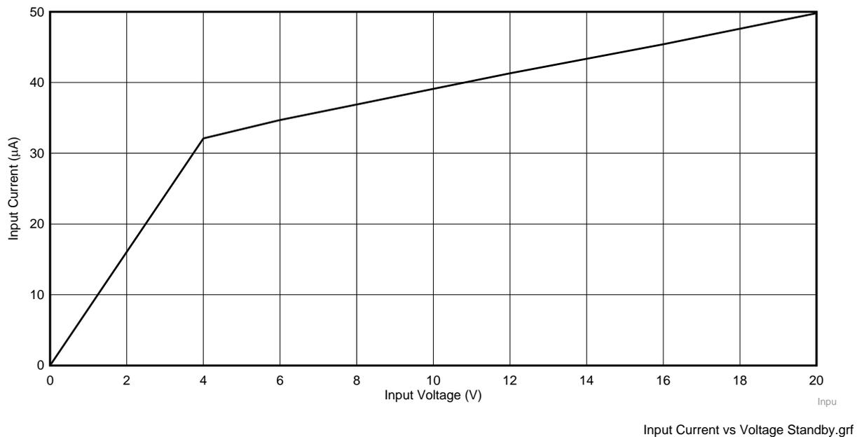
Figure 19. Input Current Versus Input Voltage, Standby Mode
