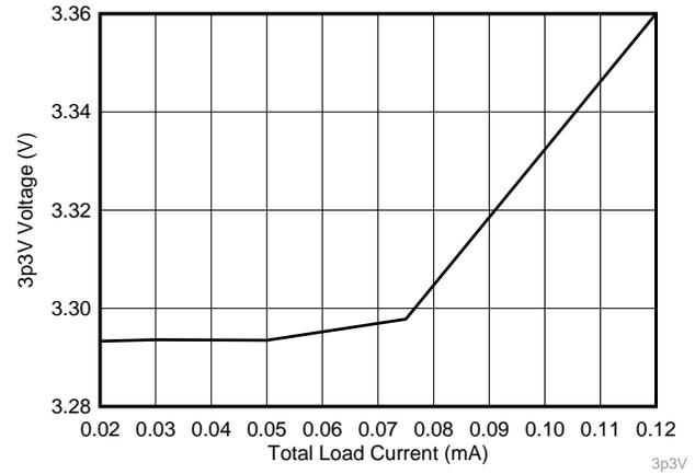
Figure 21. 3.3-V Supply Voltage Versus Load Current
