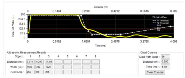
**Figure 46. Detection of Foot at 292 mm Using PUI Transducer**
