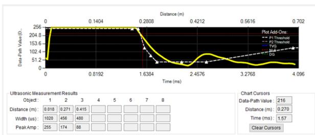
**Figure 47. Detection of Foot at 271 mm Using PUI Transducer**
