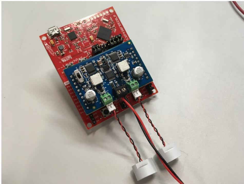
Figure 13. TIDA-01424 Board Mounted on MSP430™ LaunchPad™ Board
