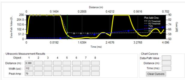
**Figure 33. Sports Shoe Detected at 380 mm**
