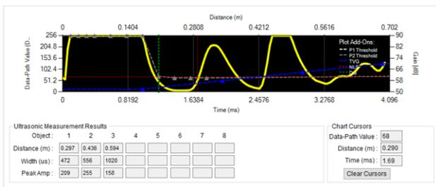
**Figure 37. Sports Shoe Detected at 297 mm**
