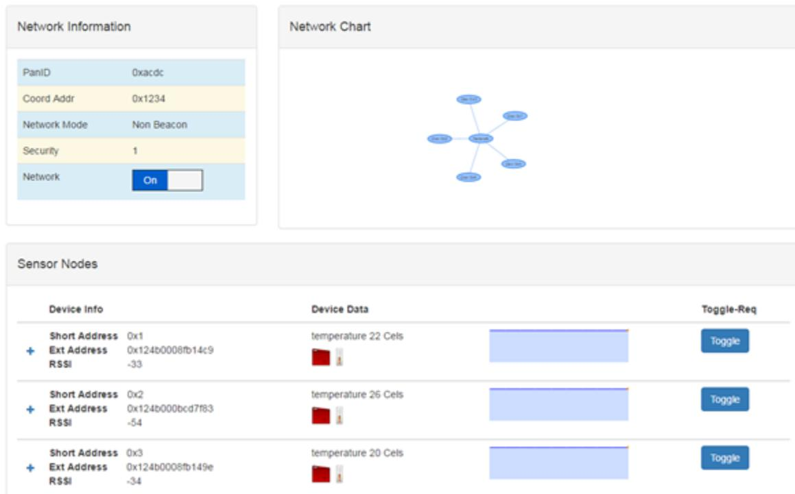
Figure 71. AWS Front End After Devices Joined
