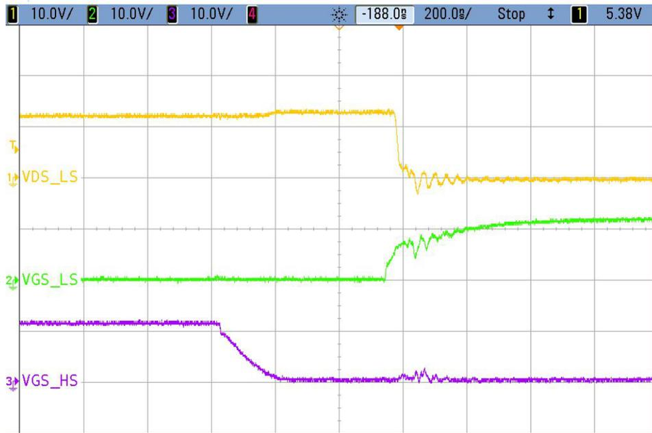
Figure 13. Switching Waveform for Turnon of Bottom FETs
