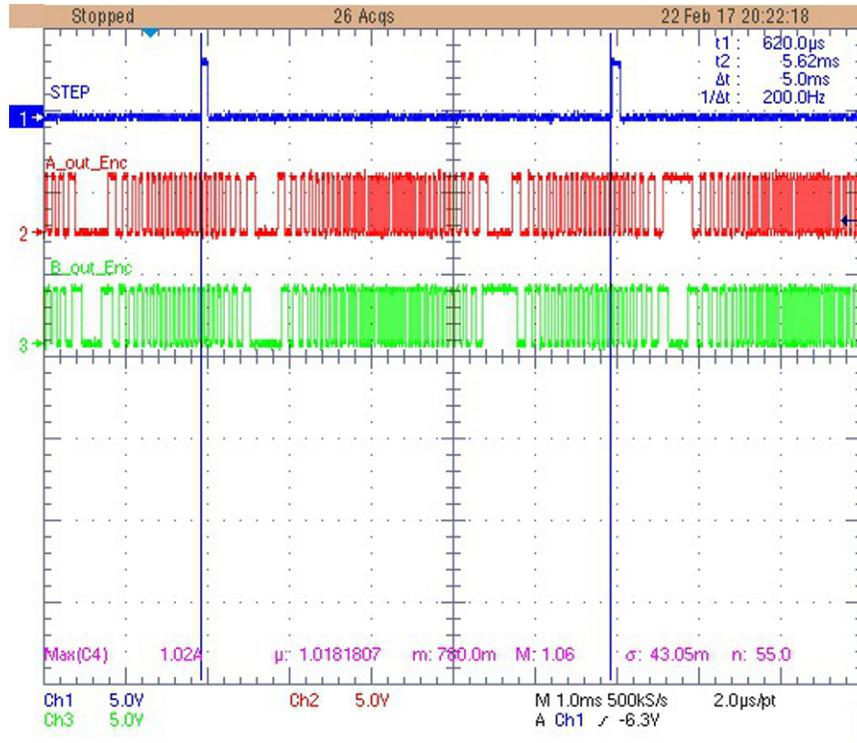
Figure 29. Resonance Condition at 5 ms
