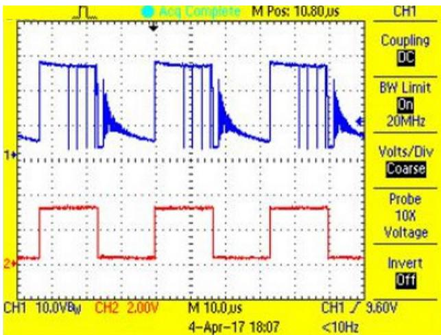
Figure 45. Switch Node and PWM Waveform for White LED String at 50% Duty Cycle
