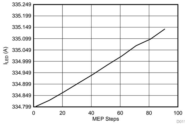
Figure 17.  $I_{LED}$  versus MEP Steps for Green LED String at 30-kHz PWM Dimming Frequency
