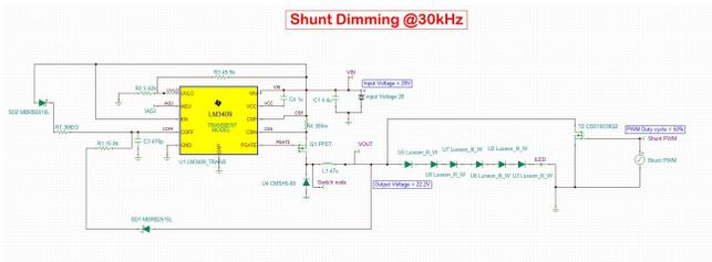
**Figure 57. Simulation Circuit for Shunt Dimming at 30 kHz With LM3409**
