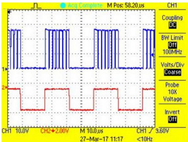
Figure 49. Switch Node and Shunt PWM Waveform for Green LED String at 50% Duty Cycle
