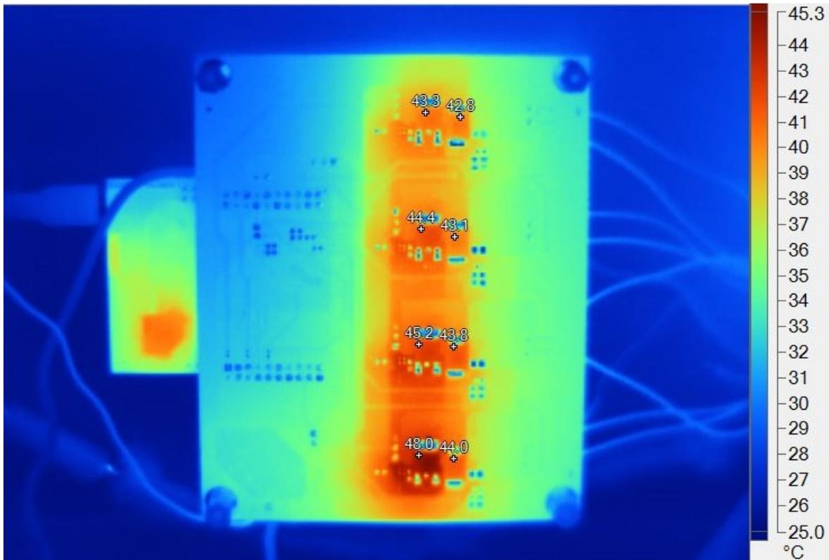
**Figure 60. Thermal Image of Bottom Side of TIDA-01415 Board for PWM Dimming at 2.9-A Total LED Current (100% Duty Cycle for All Strings)**
