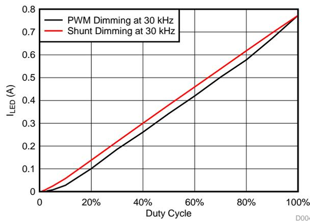
**Figure 30. I<sub>LED</sub> (A) versus Duty Cycle (%) for PWM or Shunt Dimming at 30 kHz for White LED String**
