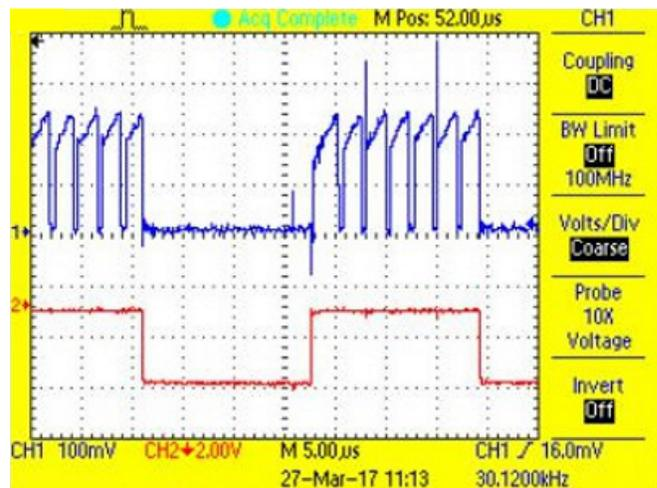
Figure 50. P-FET Current During On-Time and Shunt PWM Waveform for Green LED String at 50% Duty Cycle
