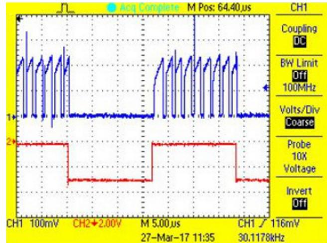
**Figure 52. P-FET Current During On-Time and Shunt PWM Waveform for Blue LED String at 50% Duty Cycle**
