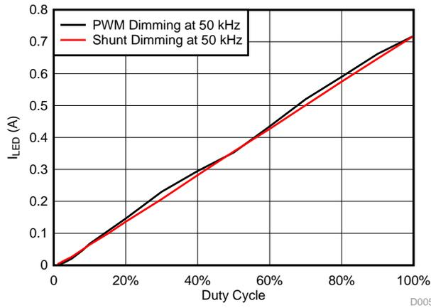
**Figure 31.  $I_{LED}$  (A) versus Duty Cycle (%) for PWM or Shunt Dimming at 50 kHz for Red LED String**
