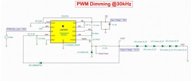
**Figure 55. Simulation Circuit for PWM Dimming With LM3409**
