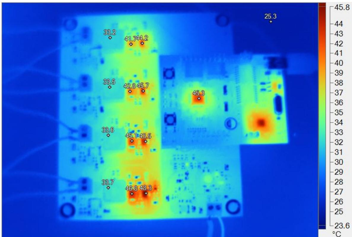
**Figure 61. Thermal Image of Top Side of TIDA-01415 Board for Shunt Dimming at 2.9-A Total LED Current (100% Duty Cycle for All Strings)**
