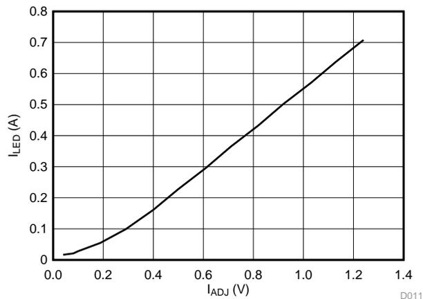
**Figure 24.  $I_{LED}$  (A) versus  $I_{ADJ}$  (V) for Green LED String**
