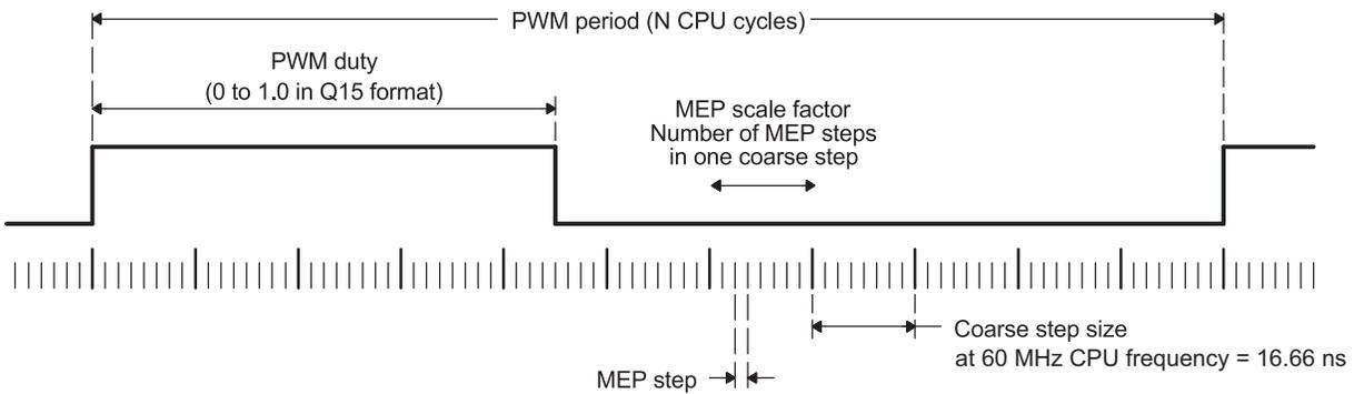
**Figure 16. Conventional PWM and HRPWM Timing Diagram**
