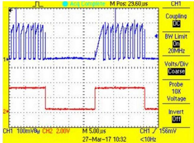
Figure 40. P-FET Current During On-Time and PWM Waveform for Red LED String at 50% Duty Cycle
