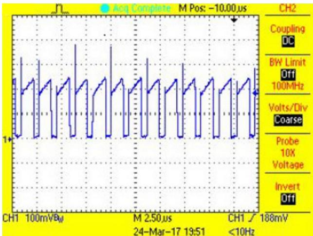
Figure 37. P-FET Current During On-Time at  $I_{ADJ} = 1.24$  V for Blue String
