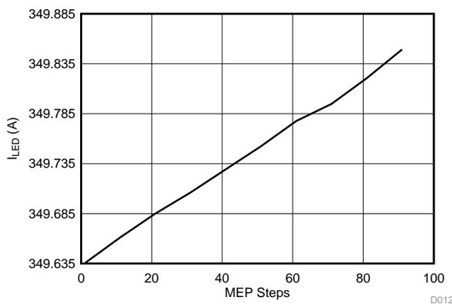
Figure 18.  $I_{LED}$  versus MEP Steps for Green LED String at 30-kHz Shunt Dimming Frequency
