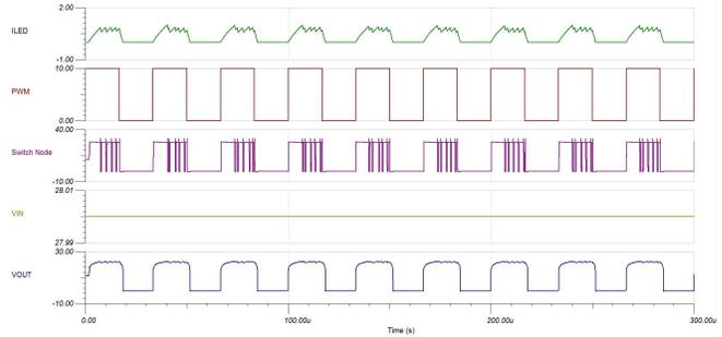
**Figure 56. Simulation Results for PWM Dimming at 30 kHz**
