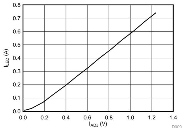
**Figure 26.  $I_{LED}$  (A) versus  $I_{ADJ}$  (V) for White LED String**
