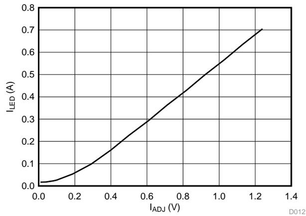
**Figure 25.  $I_{LED}$  (A) versus  $I_{ADJ}$  (V) for Blue LED String**
