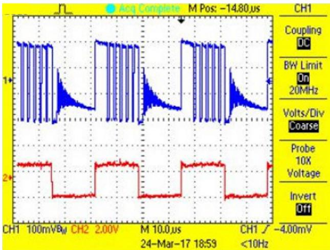
Figure 41. Switch Node and PWM Waveform for Green LED String at 50% Duty Cycle
