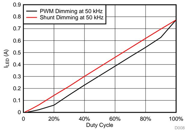
**Figure 34.  $I_{LED}$  (A) versus Duty Cycle (%) for PWM or Shunt Dimming at 50 kHz for White LED String**
