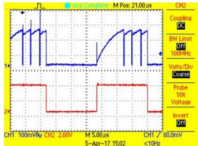
Figure 46. P-FET Current During On-Time and PWM Waveform for White LED String at 50% Duty Cycle
