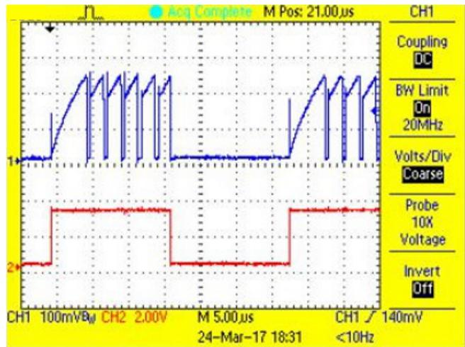
Figure 42. P-FET Current During On-Time and PWM Waveform for Green LED String at 50% Duty Cycle
