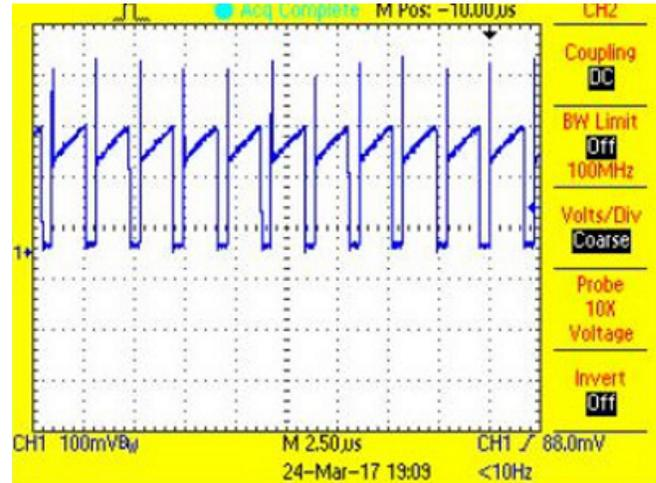
Figure 36. P-FET Current During On-Time at  $I_{ADJ} = 1.24$  V for Green String
