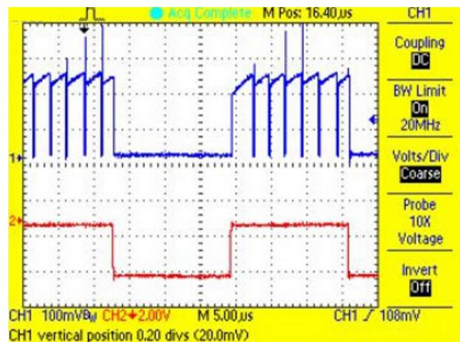
**Figure 54. P-FET Current During On-Time and Shunt PWM Waveform for White LED String at 50% Duty Cycle**
