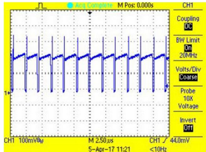
Figure 38. P-FET Current During On-Time at  $I_{ADJ} = 1.24$  V for White String
