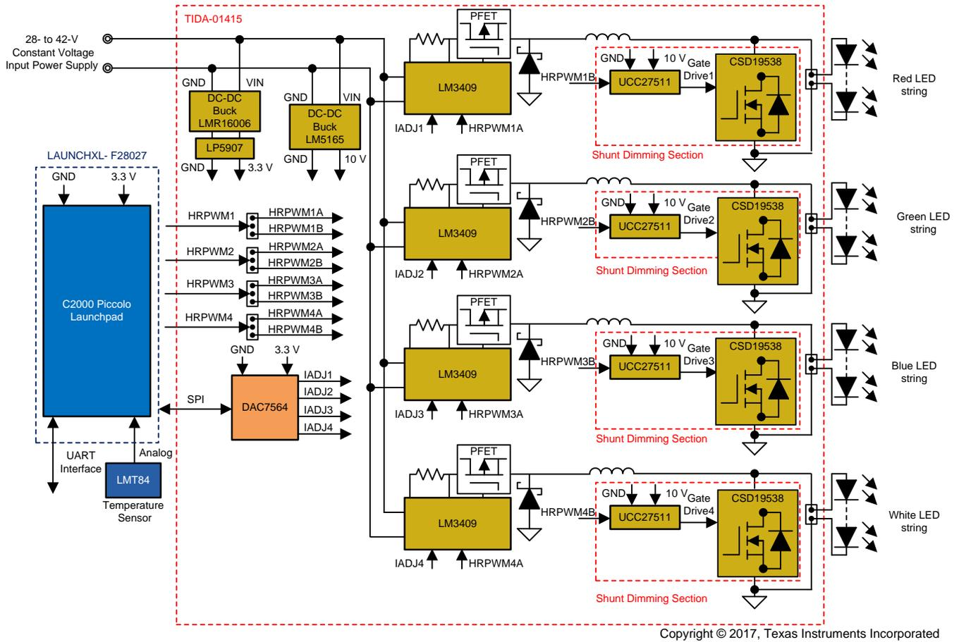
Figure 4. TIDA-01415 Block Diagram
