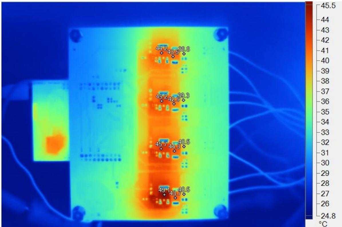
Figure 62. Thermal Image of Bottom Side of TIDA-01415 Board for Shunt Dimming at 2.9-A Total LED Current (100% Duty Cycle for All Strings)
