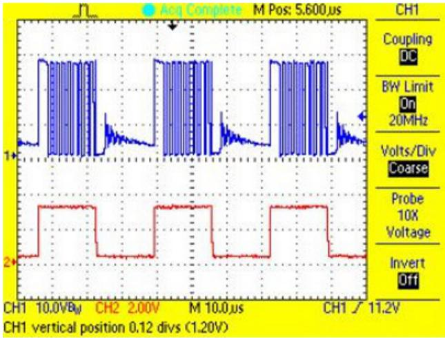
Figure 39. Switch Node and PWM Waveform for Red LED String at 50% Duty Cycle
