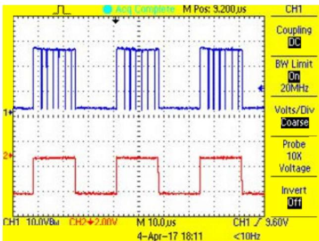
**Figure 53. Switch Node and Shunt PWM Waveform for White LED String at 50% Duty Cycle**
