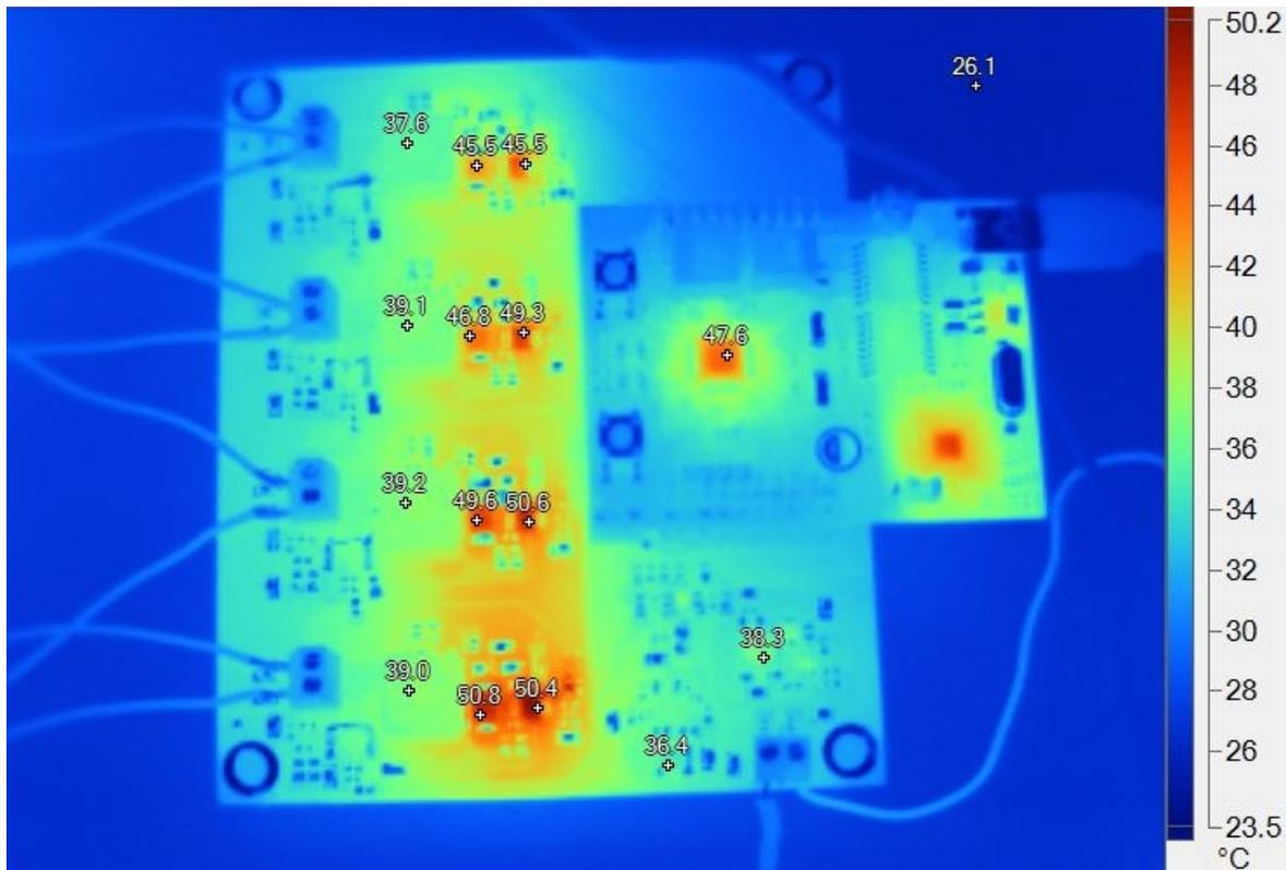
Figure 59. Thermal Image of Top Side of TIDA-01415 Board for PWM Dimming at 2.9-A Total LED Current (100% Duty Cycle for All Strings)
