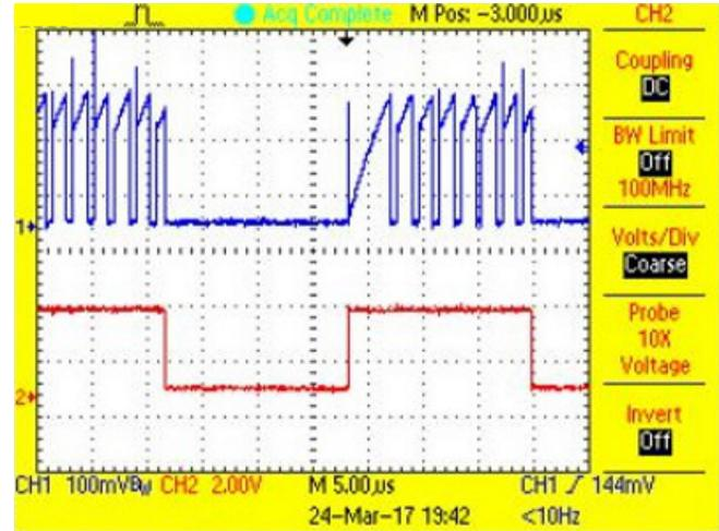
Figure 44. P-FET Current During On-Time and PWM Waveform for Blue LED String at 50% Duty Cycle
