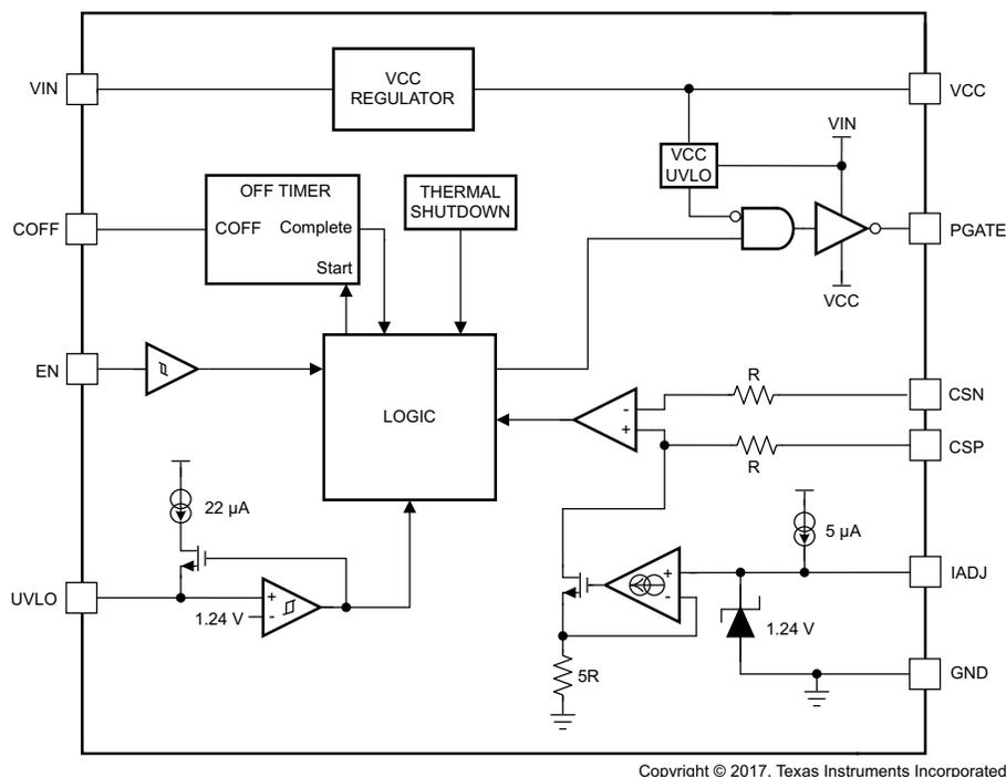
**Figure 5. Functional Block Diagram of LM3409**
