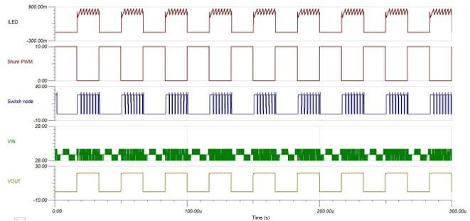
**Figure 58. Simulation Results for Shunt Dimming at 30 kHz**
