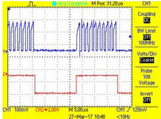
Figure 48. P-FET Current During On-Time and Shunt PWM Waveform for Red LED String at 50% Duty Cycle
