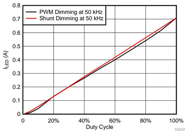
**Figure 33. I<sub>LED</sub> (A) versus Duty Cycle (%) for PWM or Shunt Dimming at 50 kHz for Blue LED String**
