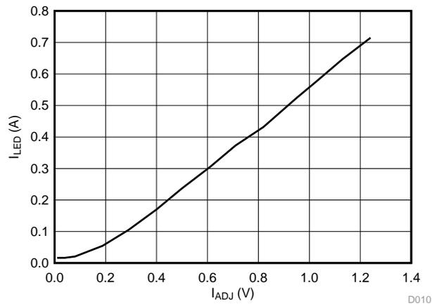
**Figure 23.  $I_{LED}$  (A) versus  $I_{ADJ}$  (V) for Red LED String**
